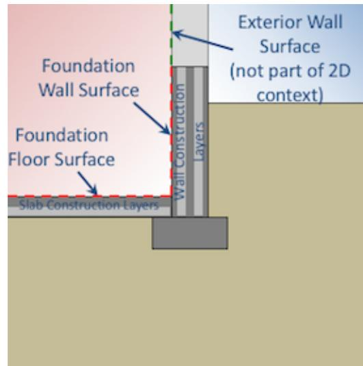
Figure 1.48: Two-dimensional interpretation of foundation surface data
