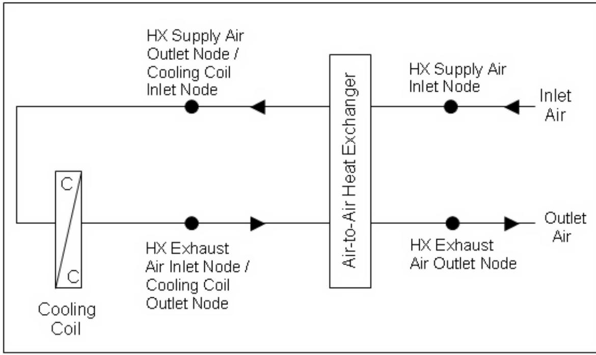
Figure 1.178: Schematic of the CoilSystem:Cooling:DX:HeatExchangerAssisted compound object
