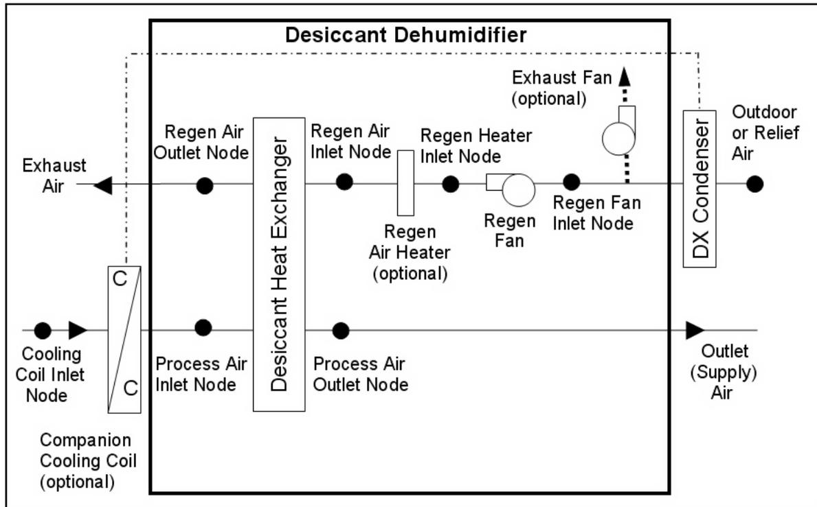
Figure 1.189: Schematic of `Dehumidifier:Desiccant:System` with Blow Through Regeneration Fan Placement
