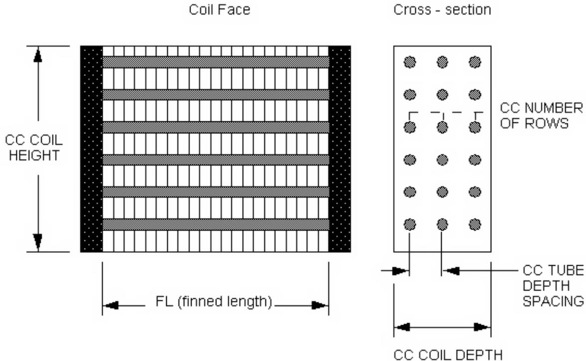
Figure 1.169: Geometry of a Cooling Coil (CC)
