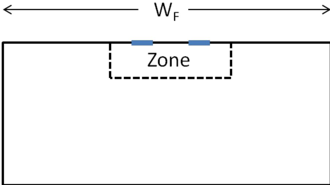
Figure 1.117: Footprint of a rectangular building showing  $W_F$ , the “Façade Width”, used by the Single Sided Wind Pressure Coefficient Algorithm.
