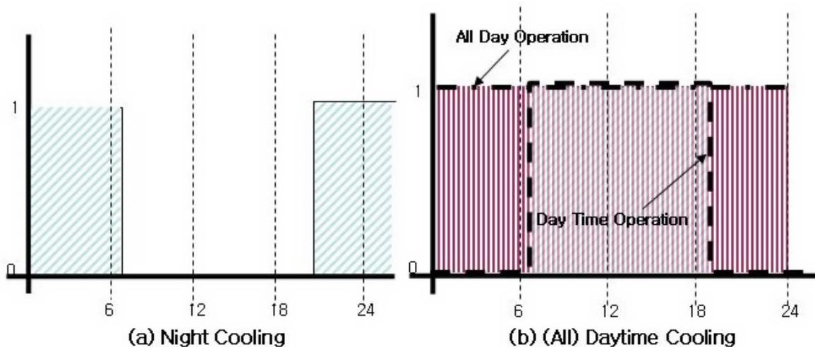
Figure 1.161: Example operating schedule for Ventilated Slab
