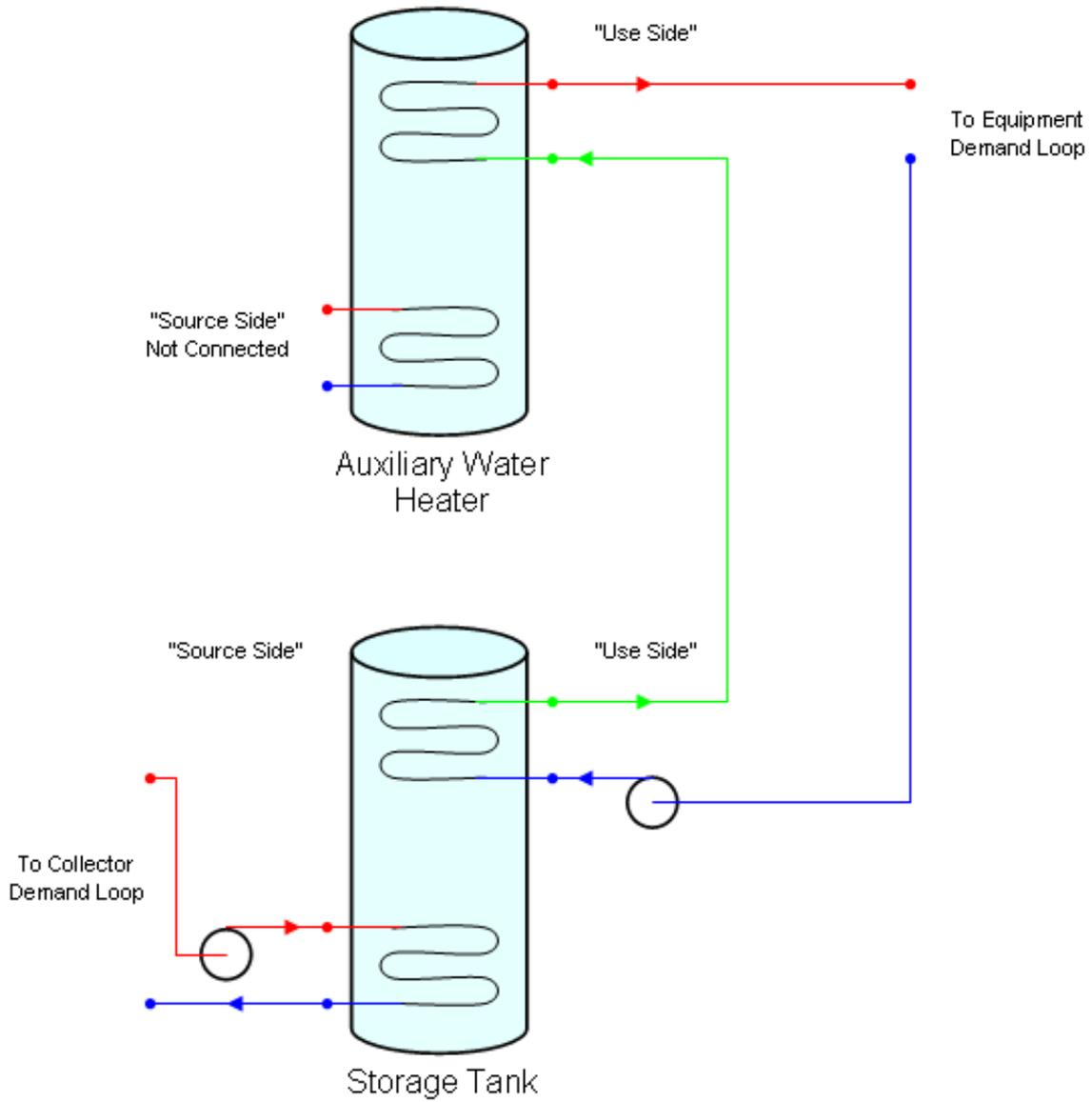
Figure 1.165: Two-Tank Solar Heating System Connection Diagram
