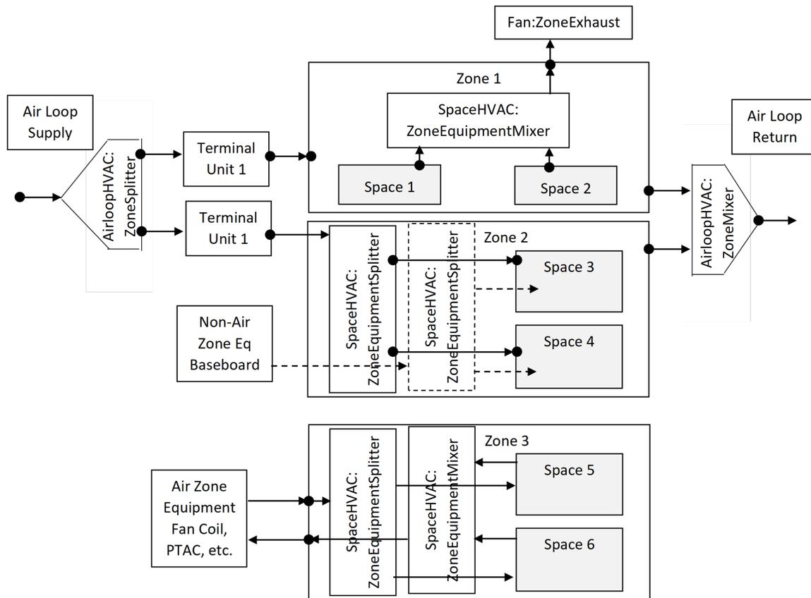
Figure 1.125: Space HVAC Equipment Connections
