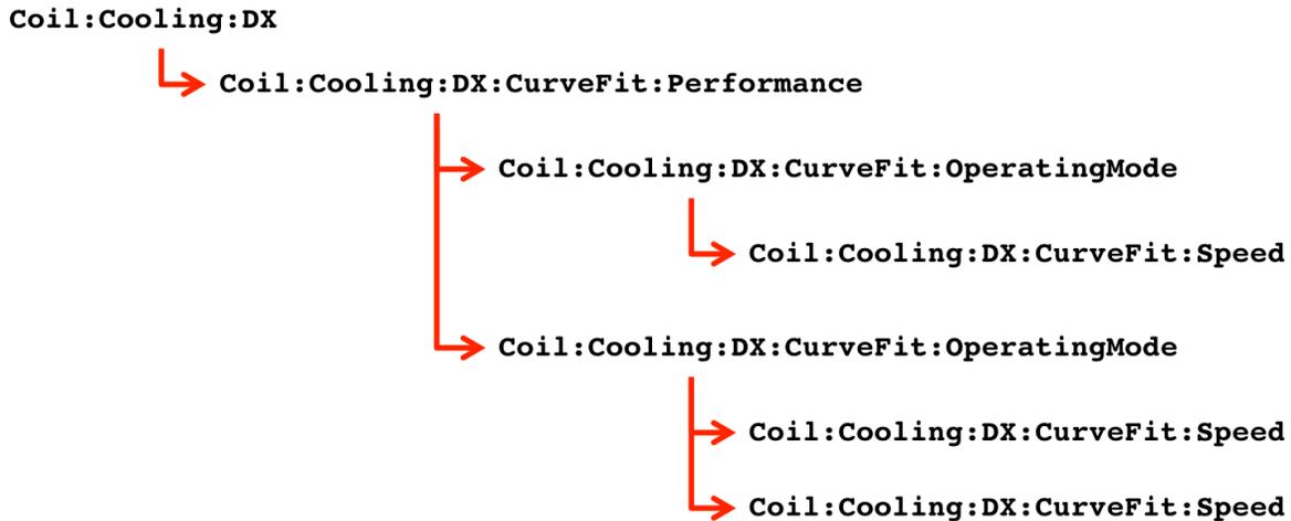
Figure 1.187: Hierarchy of references between cooling coil objects
