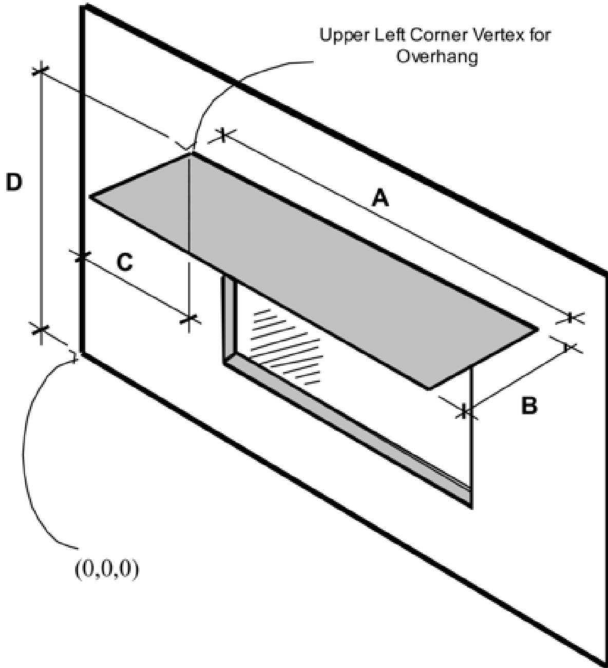
Figure 1.35: Illustration for Attached Shading Surface
