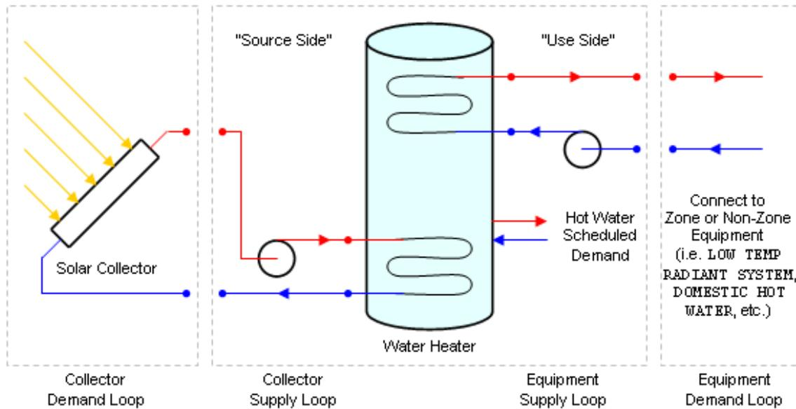
Figure 1.164: Solar Collector Plant Loop Connection Diagram
