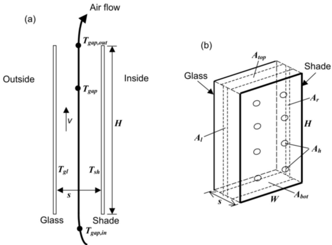
Figure 1.14: Vertical section (a) and perspective view (b) of glass and interior shade layers showing variables used in the gap air flow analysis. In (b), the air-flow opening areas  $A_{bot}$ ,  $A_{top}$ ,  $A_l$ ,  $A_r$  and  $A_h$  are shown schematically. See *Engineering Manual* for definition of thermal variables.
