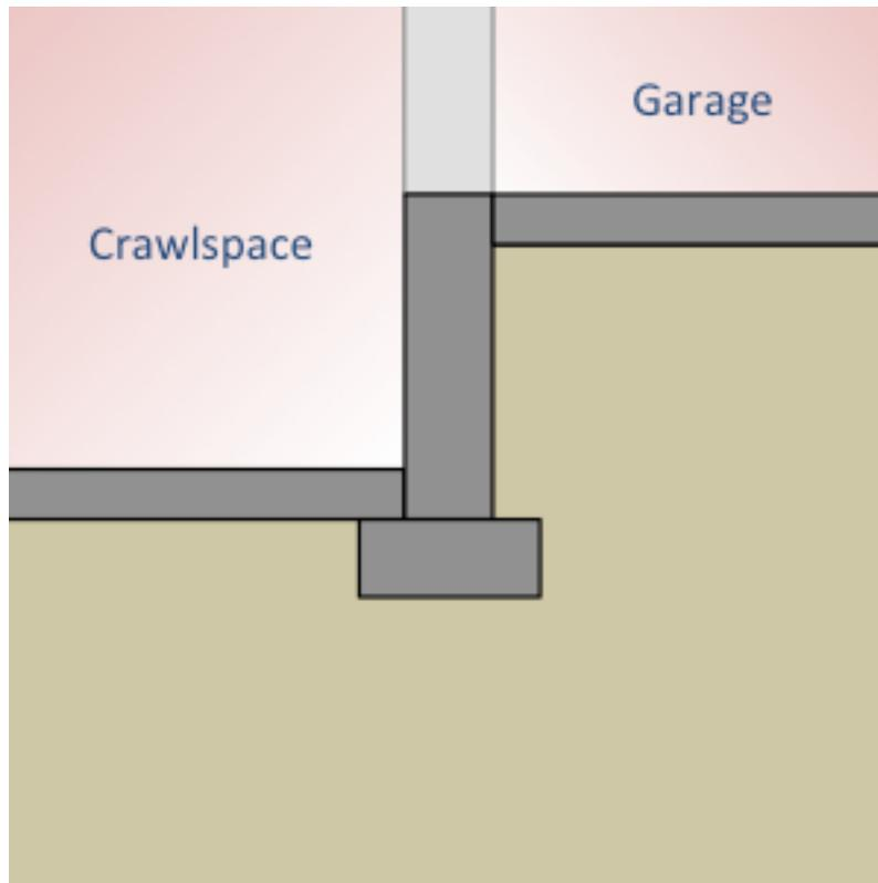
Figure 1.63: Interior foundation wall
