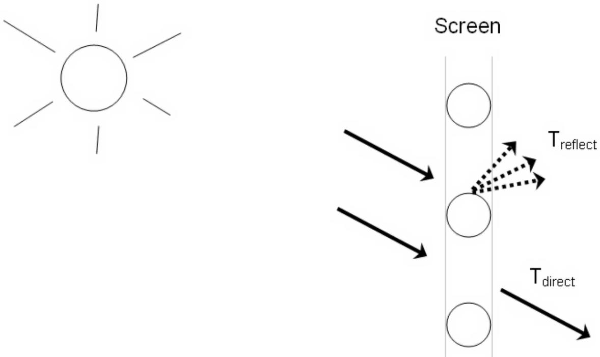
Figure 1.21: Direct beam and reflected beam transmittance components
