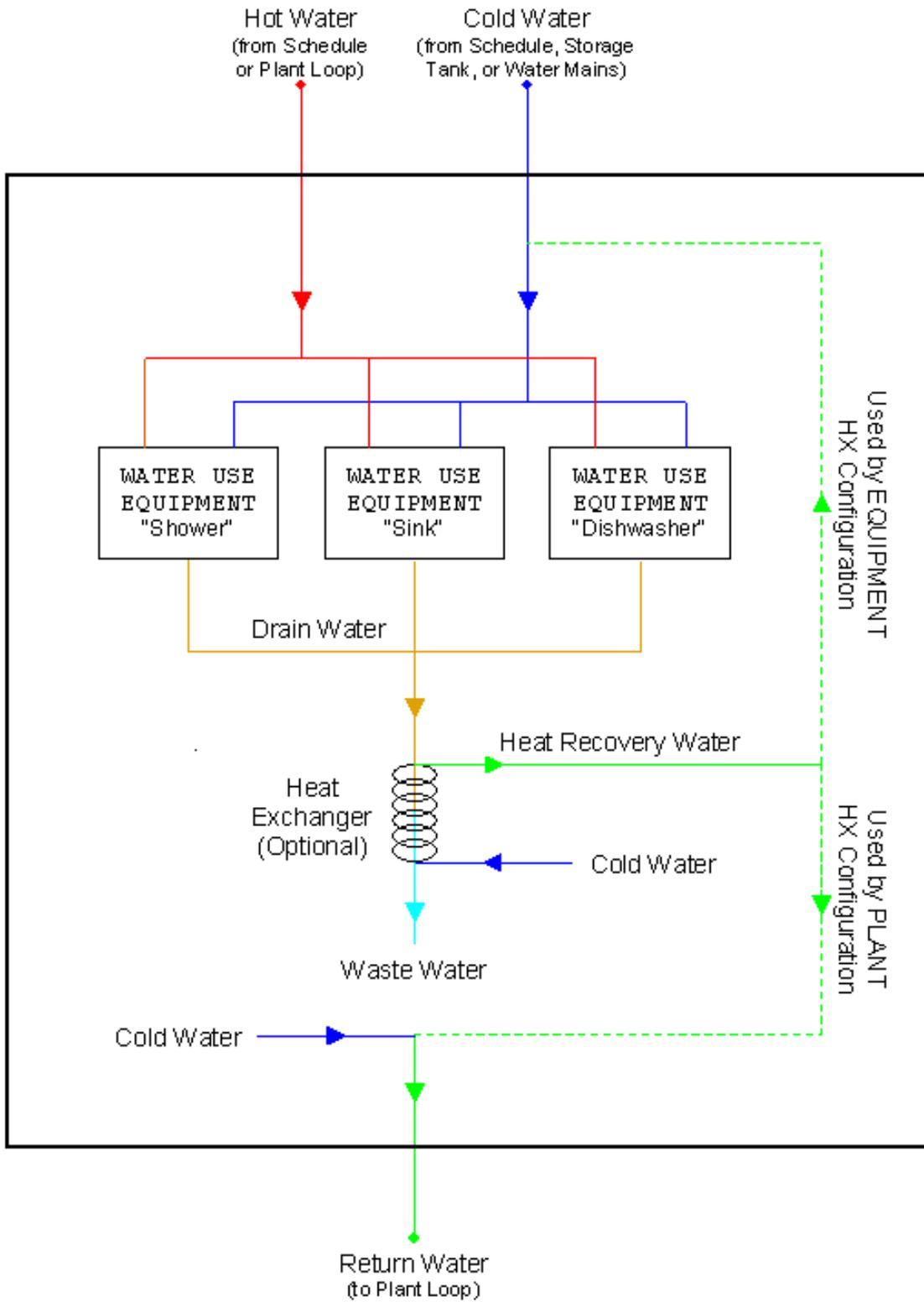
Figure 1.206: Diagram of internal connections for WaterUse:Connections
