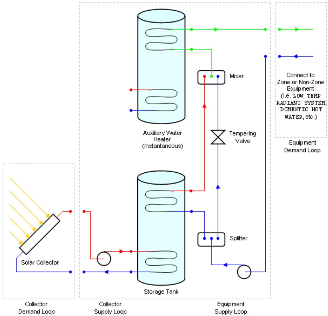
Figure 1.166: Two-Tank Solar Heating System with Tempering Valve
