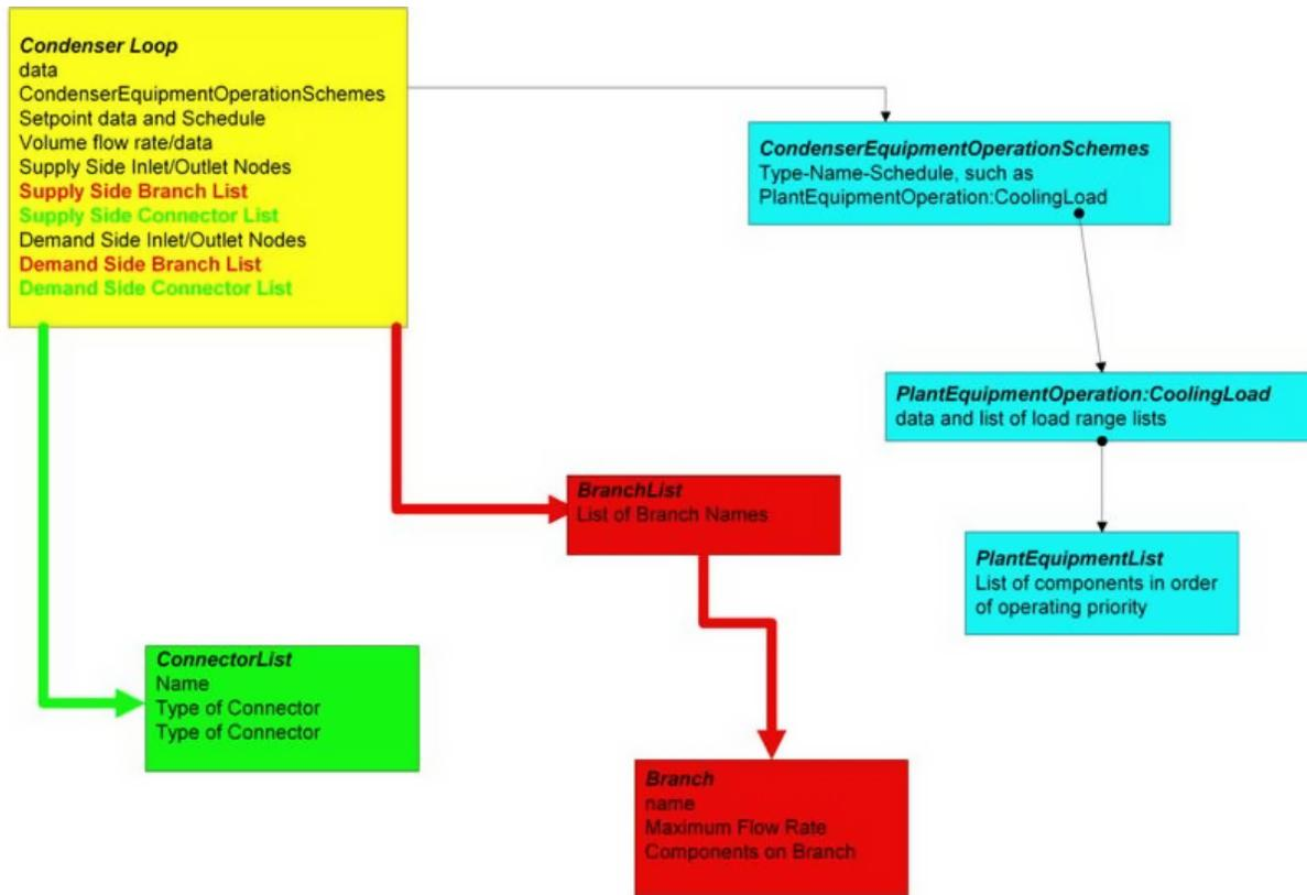
Figure 1.91: Condenser Loop Input Syntax Map
