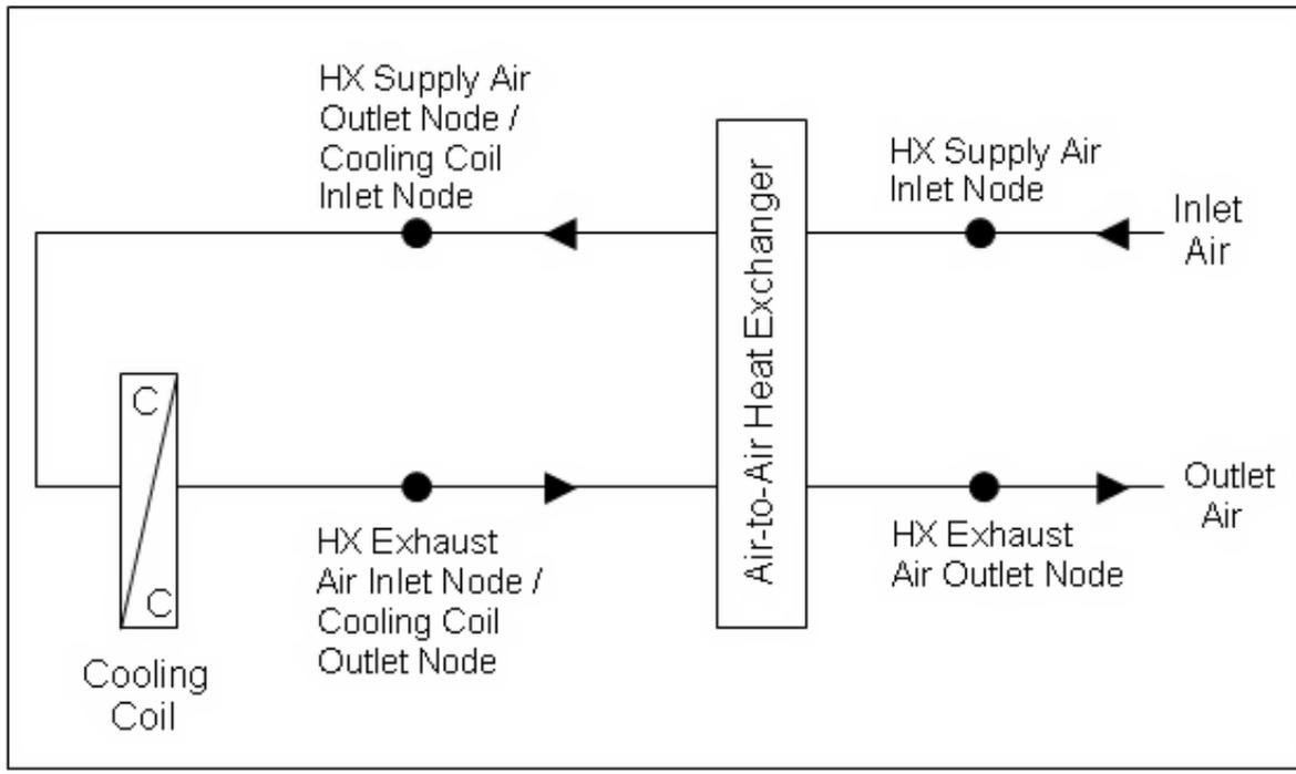
Figure 1.171: Schematic of the `CoilSystem:Cooling:Water:HeatExchangerAssisted` compound object
