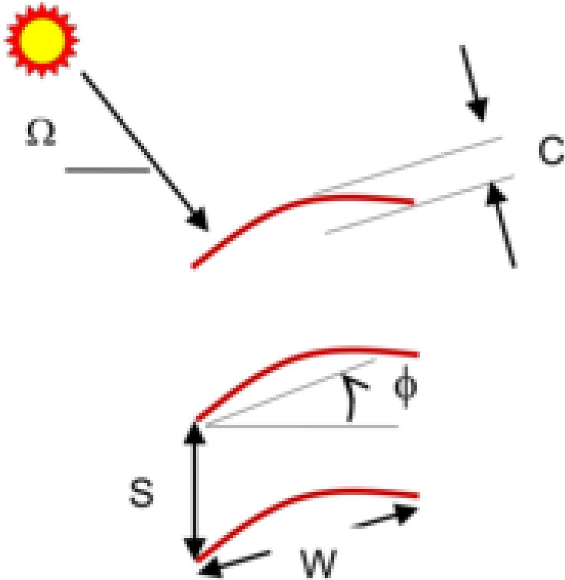
Figure 1.24: Geometry and Properties used for venetian blind analysis
