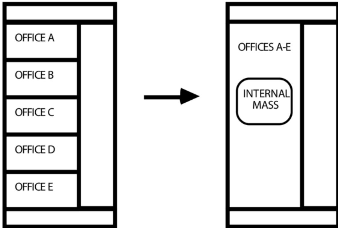
Figure 1.32: Representing 11 internal walls as internal mass
