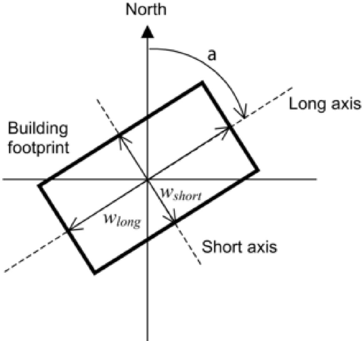
Figure 1.116: Footprint of a rectangular building showing variables used by the program to calculate surface-average wind pressure coefficients. The angle  $a$  is the “Azimuth Angle of Long Axis of Building.”  $w_{short}/w_{long}$  is the “Ratio of Building Width Along Short Axis to Width Along Long Axis.”
