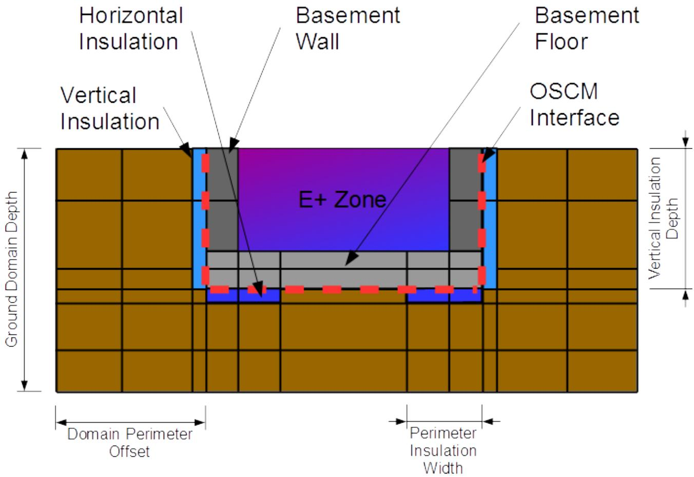
Figure 1.9: Basement Configuration
