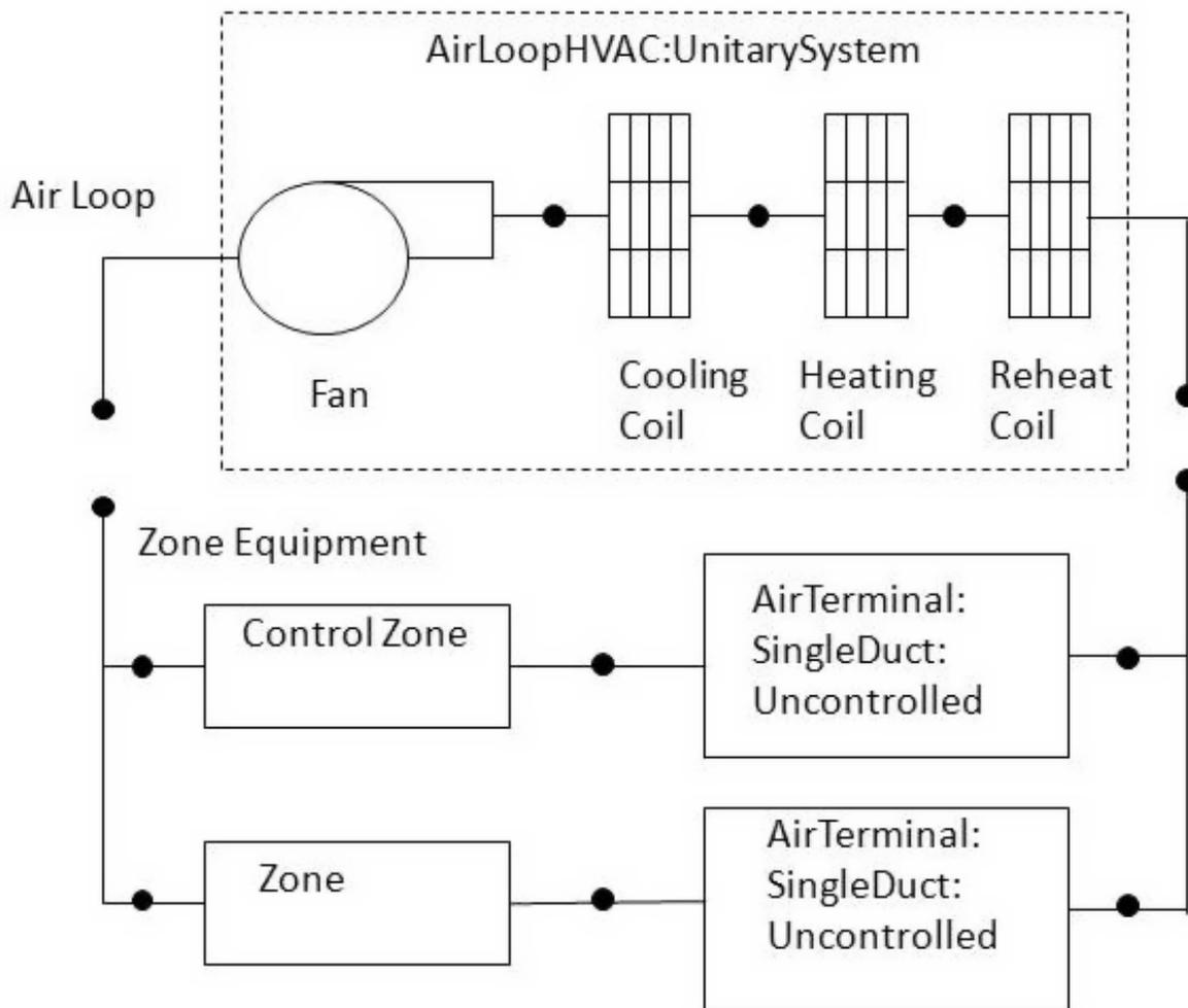
Figure 1.146: Schematic of the EnergyPlus Unitary System
