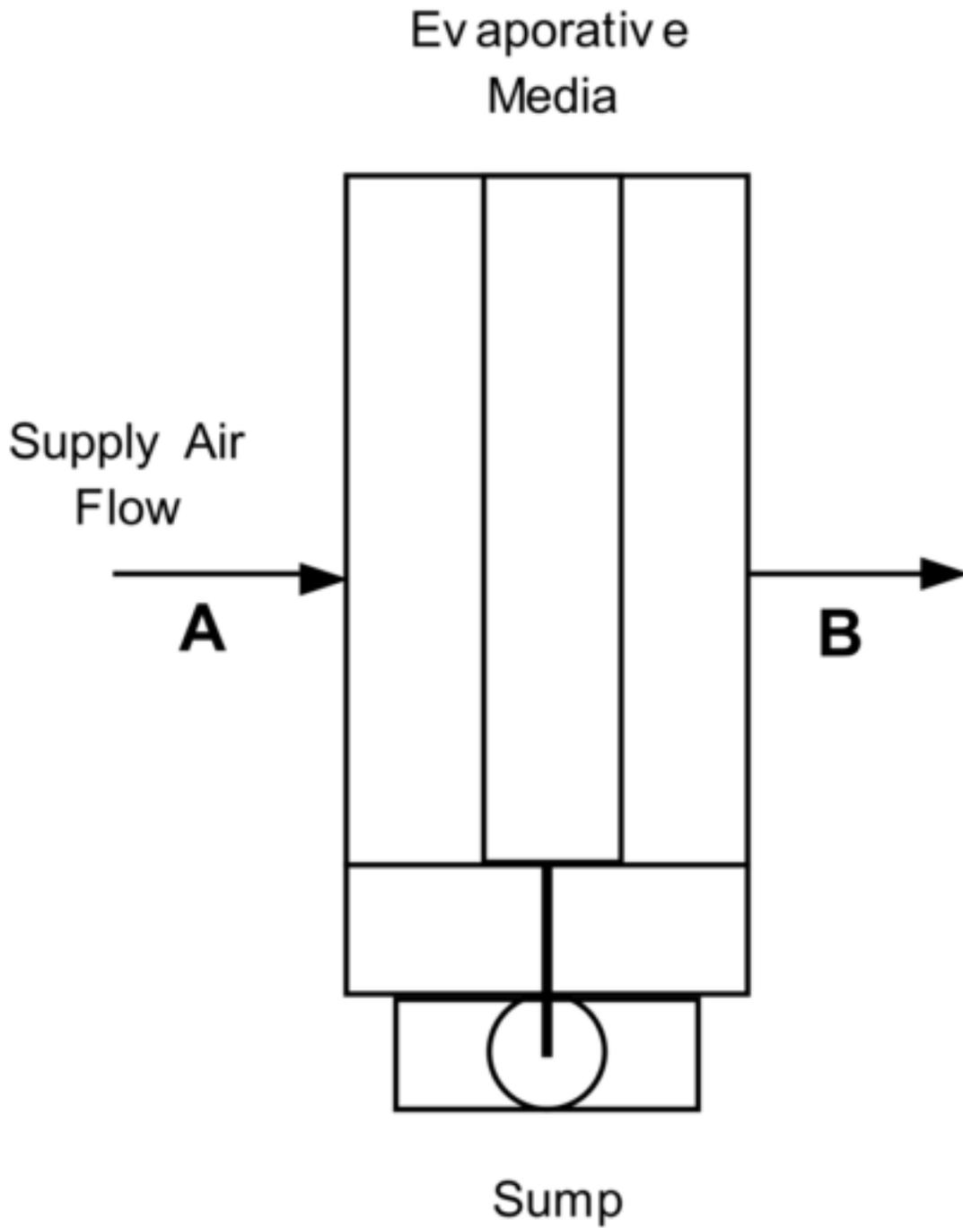
Figure 1.191: Direct Stage Evaporative Cooler
