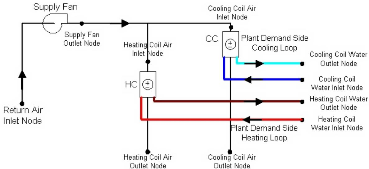
Figure 1.168: Example Air Loop Heating &amp; Cooling Coil
