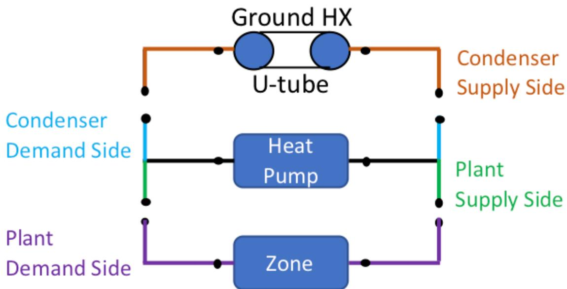
Figure 1.94: Schematic of EnergyPlus Ground Loop Heat Exchanger
