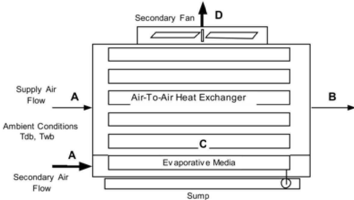
Figure 1.193: Evaporative Cooler – Indirect Dry Coil
