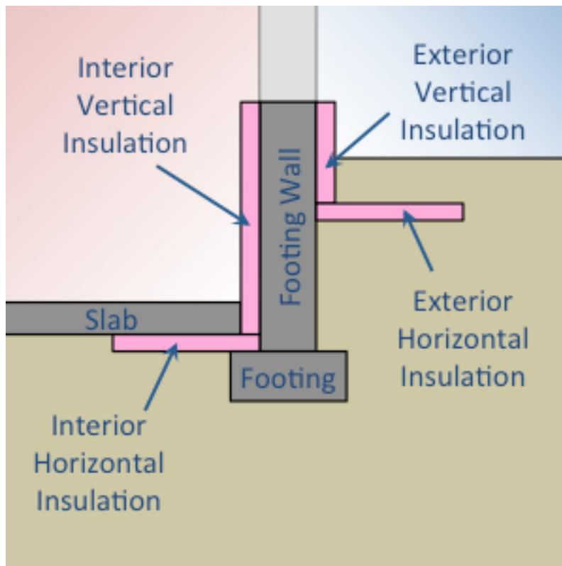
Figure 1.47: Structural and insulation components of Foundation:Kiva objects
