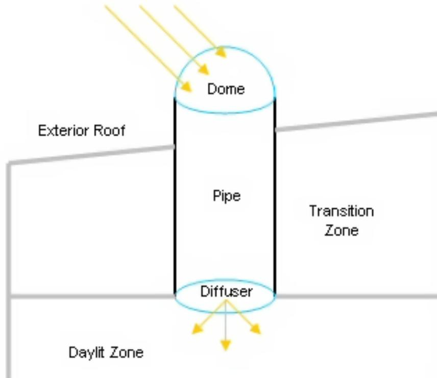
Figure 1.83: Tubular daylighting device diagram.
