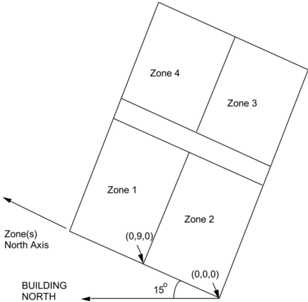
Figure 1.29: Illustration of Zone North Axis and Origins
