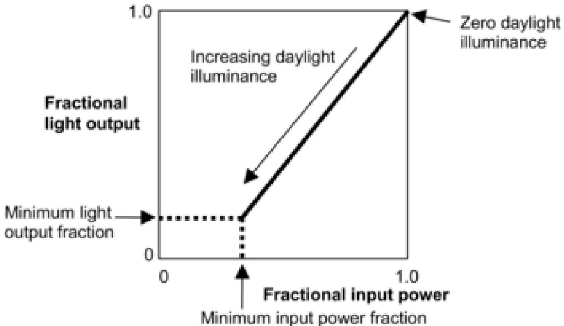
Figure 1.73: Illustration of continuous dimming relationship
