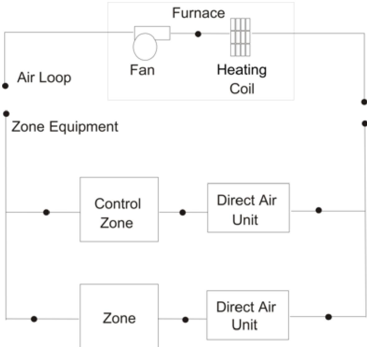
Figure 1.151: Schematic of Blow Through Furnace Model
