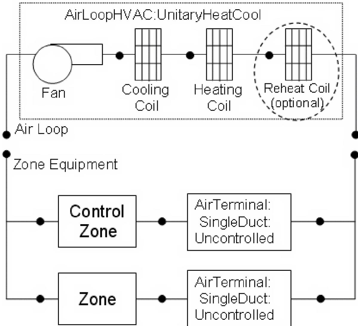
Figure 1.148: Schematic of Blow Through Heat/Cool Unitary System
