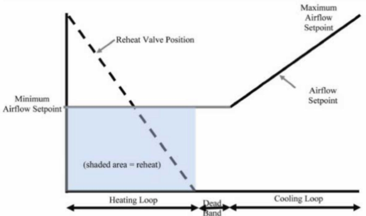
Figure 1.126: The Single Maximum Control Logic
