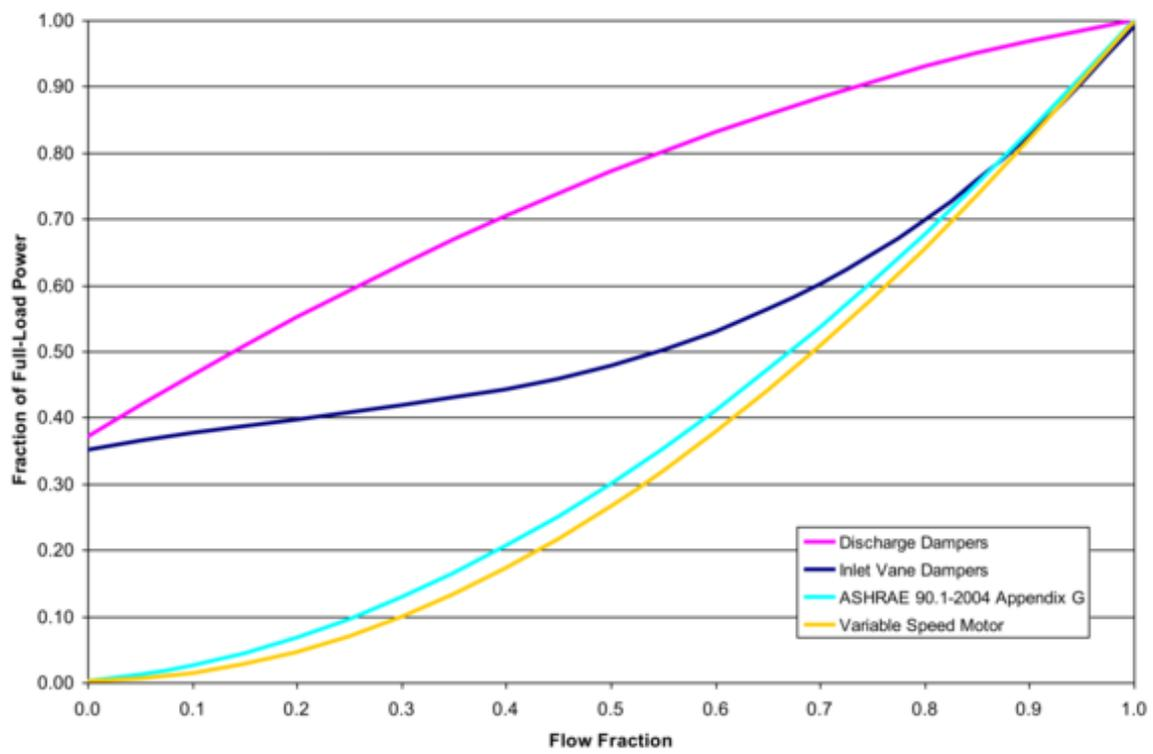
Figure 2.9: VAV Supply Fan Part-Load Power Coefficient Options
