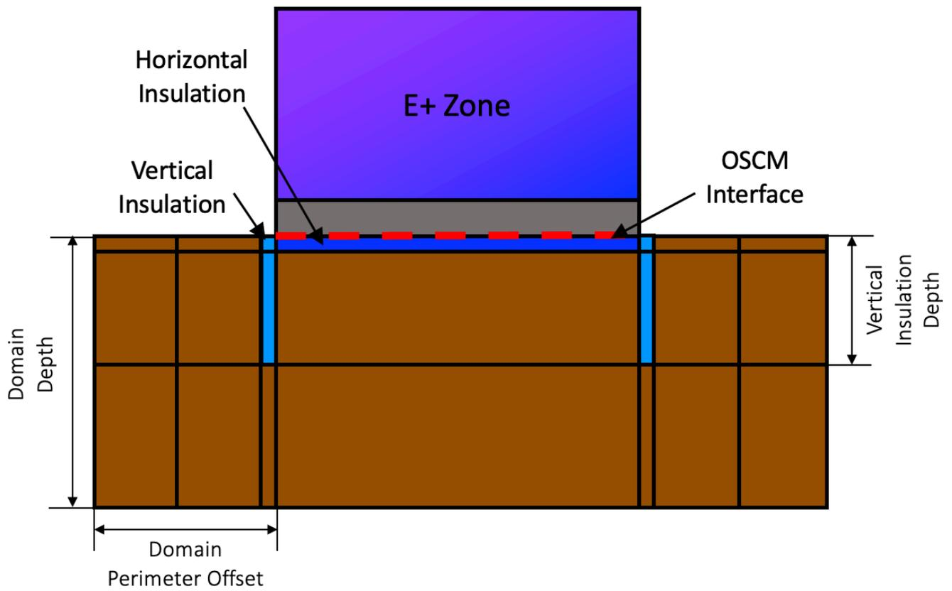
Figure 1.8: On-grade configuration
