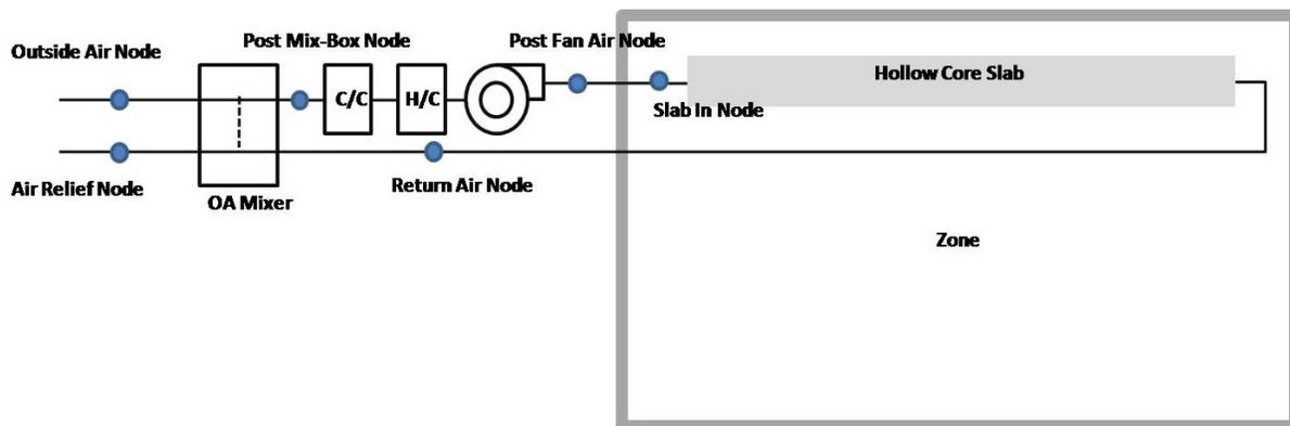
Figure 1.160: Ventilated Slab model - basic system
