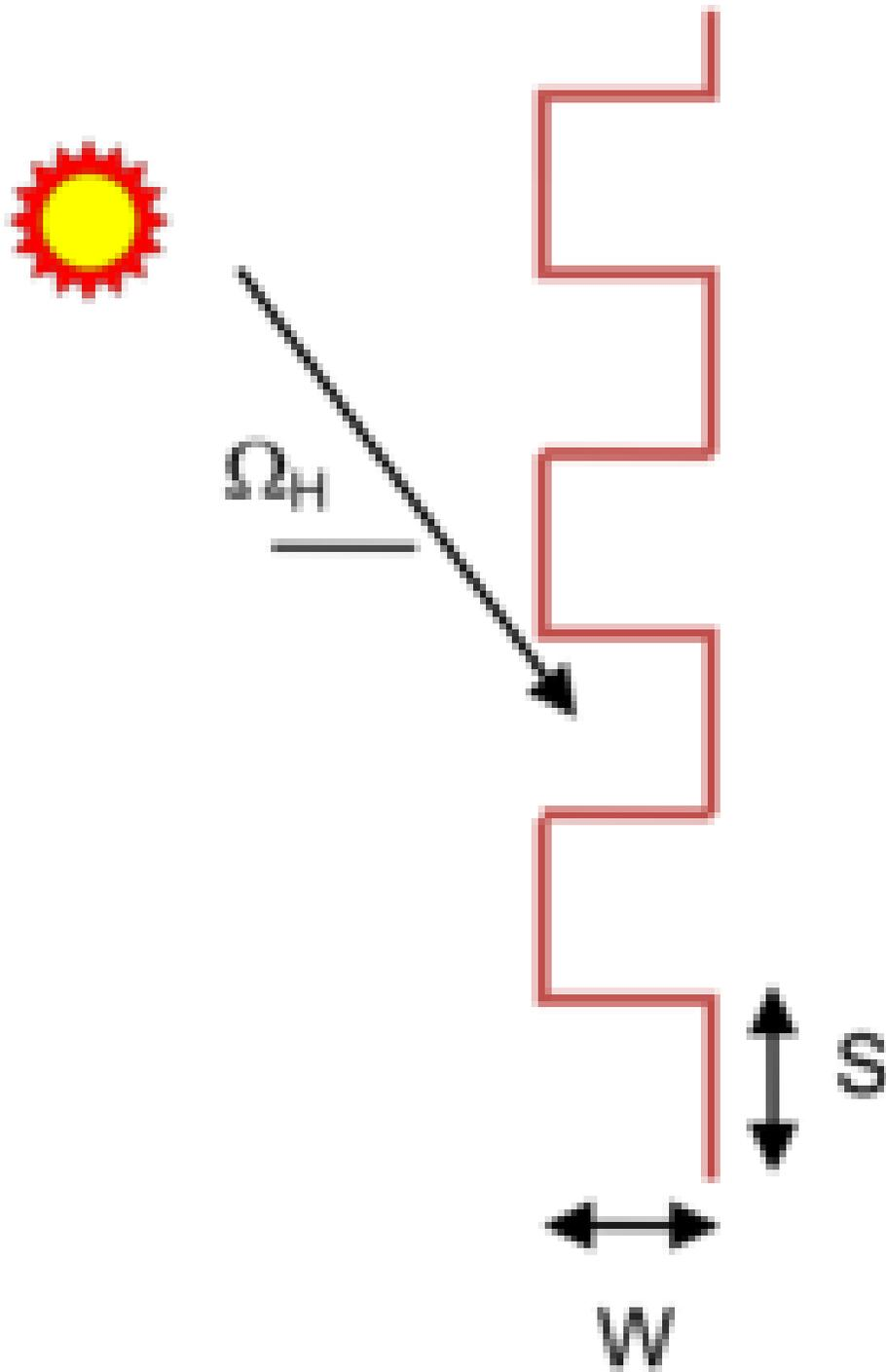
Figure 1.23: Geometry used for Pleated Drape Analysis
