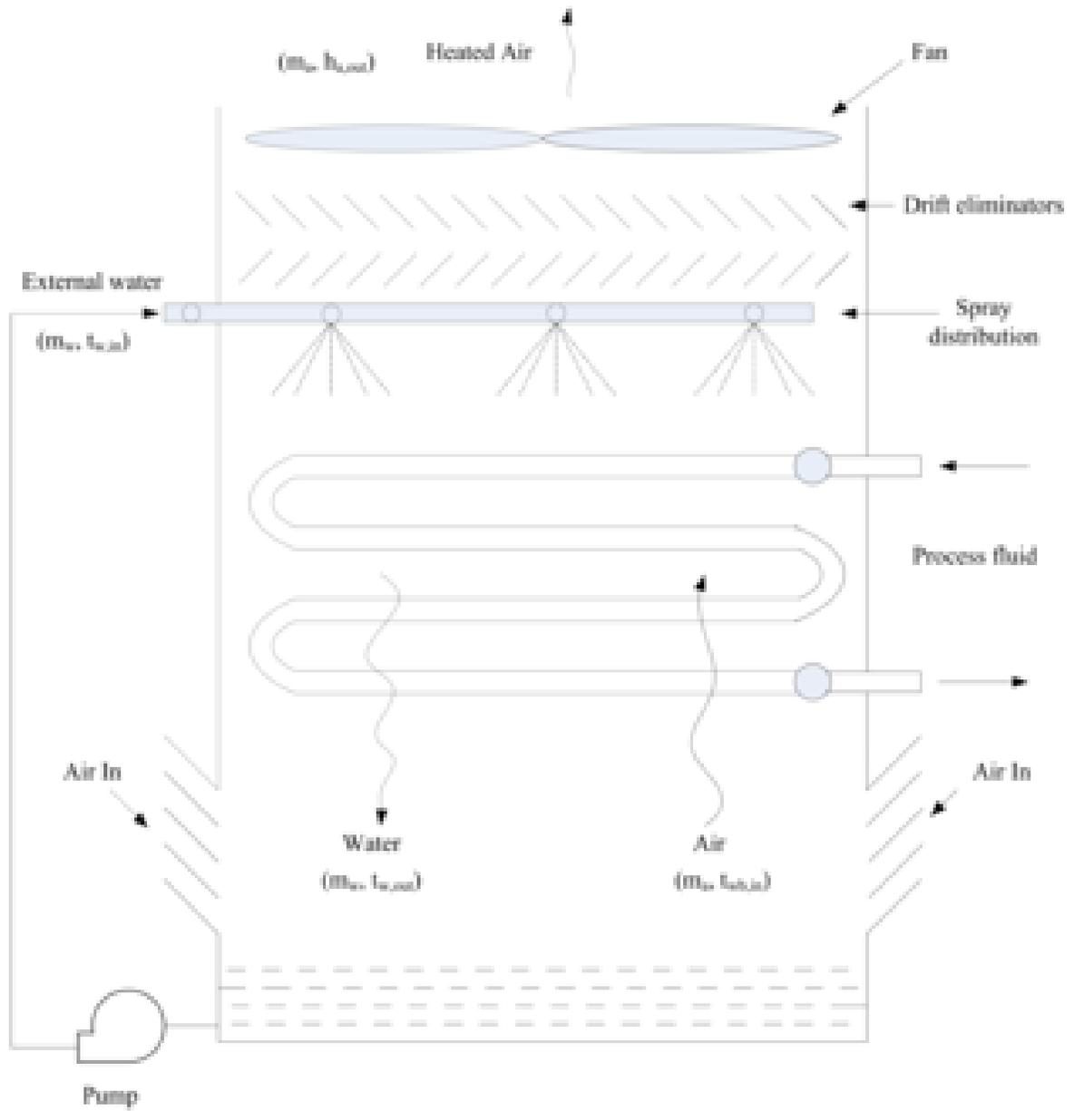
Figure 1.101: Schematic diagram for evaporative fluid cooler
