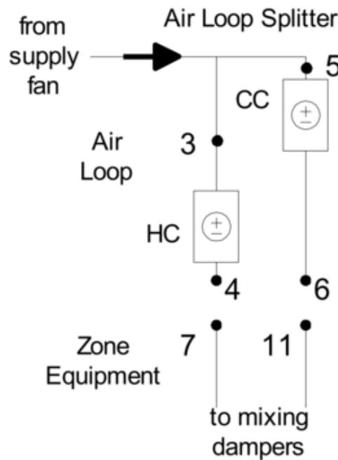
Figure 1.123: Air Loop/Zone Equipment Node Diagram
