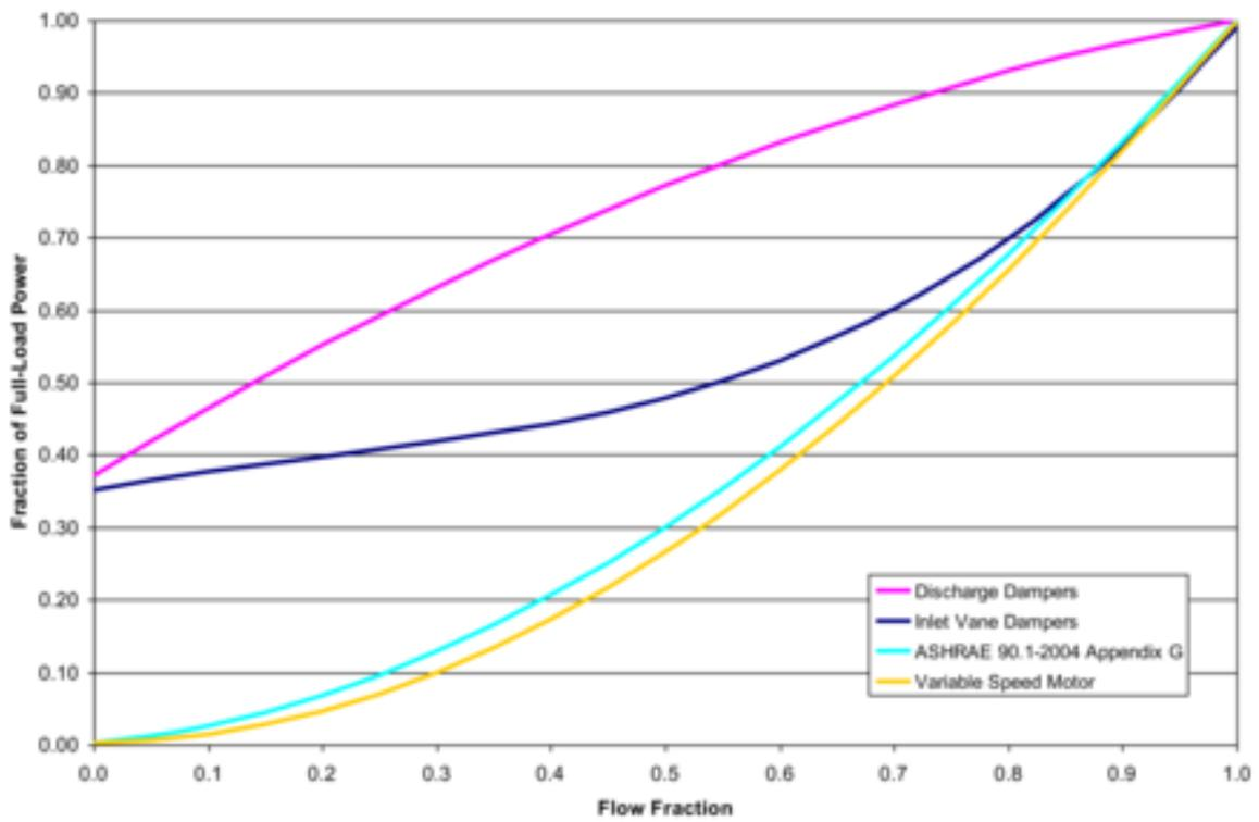
Figure 2.7: VAV Supply Fan Part-Load Power Coefficient Options
