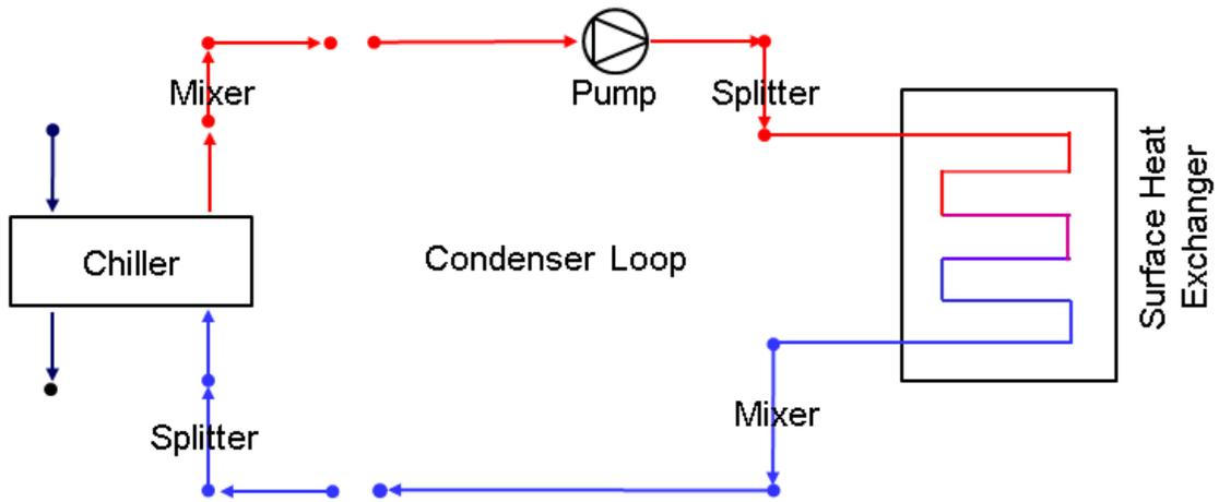
Figure 1.107: Example of Surface Ground Heat Exchanger as only heat exchanger on condenser loop
