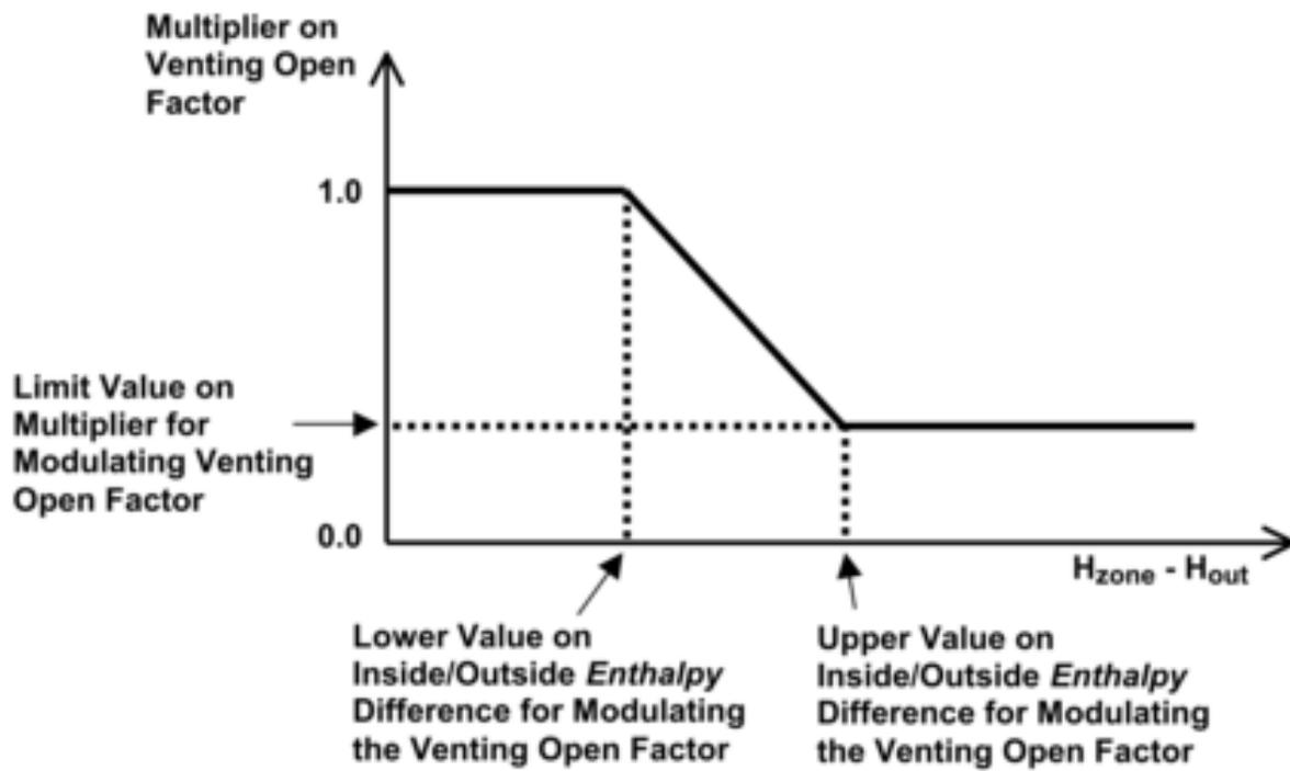
Figure 1.119: Modulation of venting area according to inside-outside enthalpy difference.
