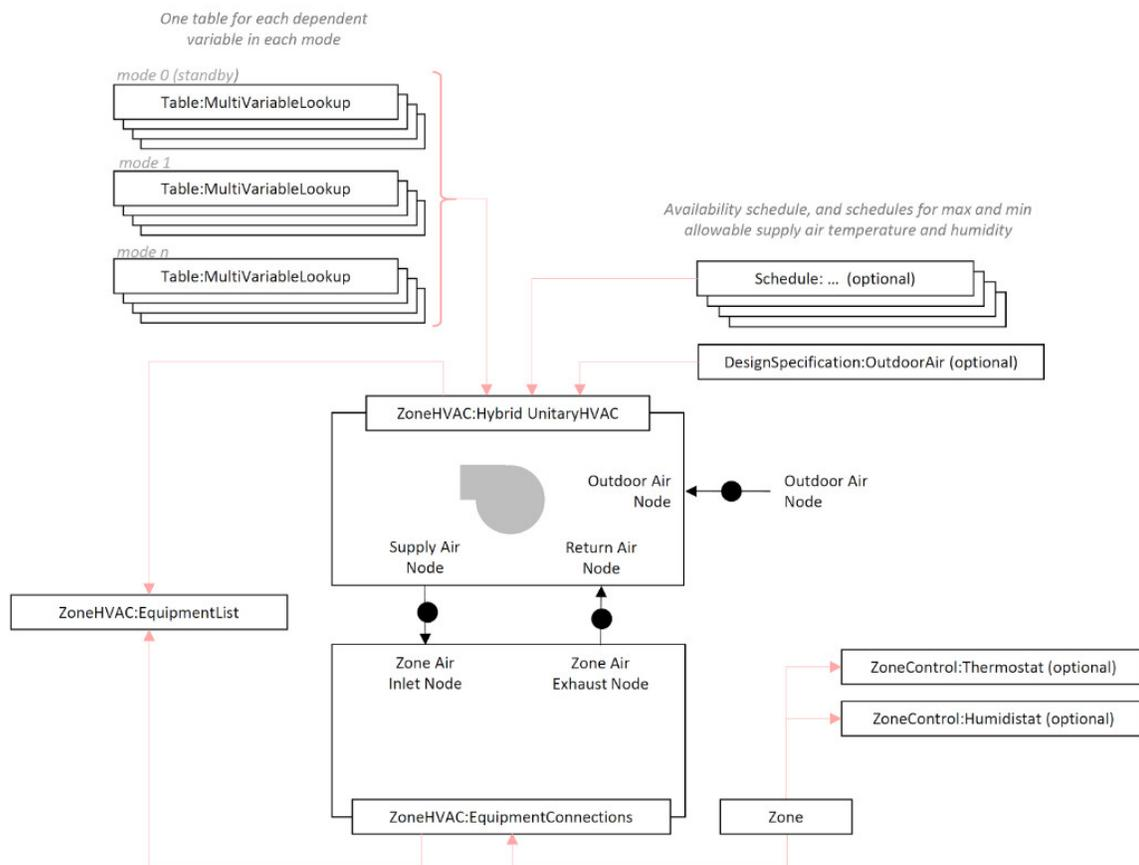
Figure 1.143: Schematic of object links for ZoneHVAC:HybridUnitaryHVAC
