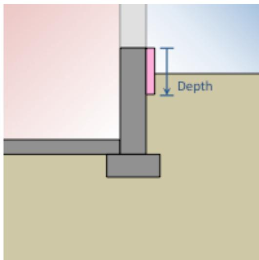
Figure 1.55: Placement of exterior vertical insulation
