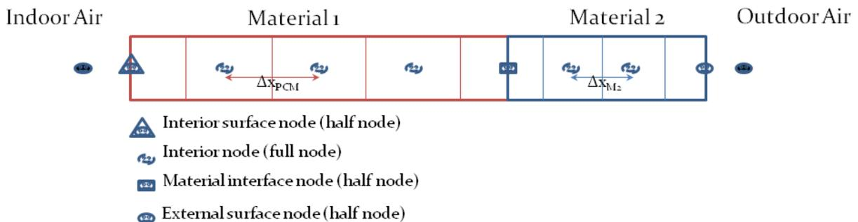
Figure 3.6: Node depiction for Conduction Finite Difference Model
