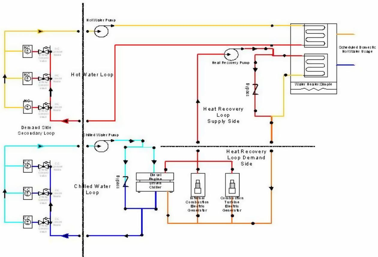
Figure 9.10: Example of a Heat Recovery Loop Simulation.
