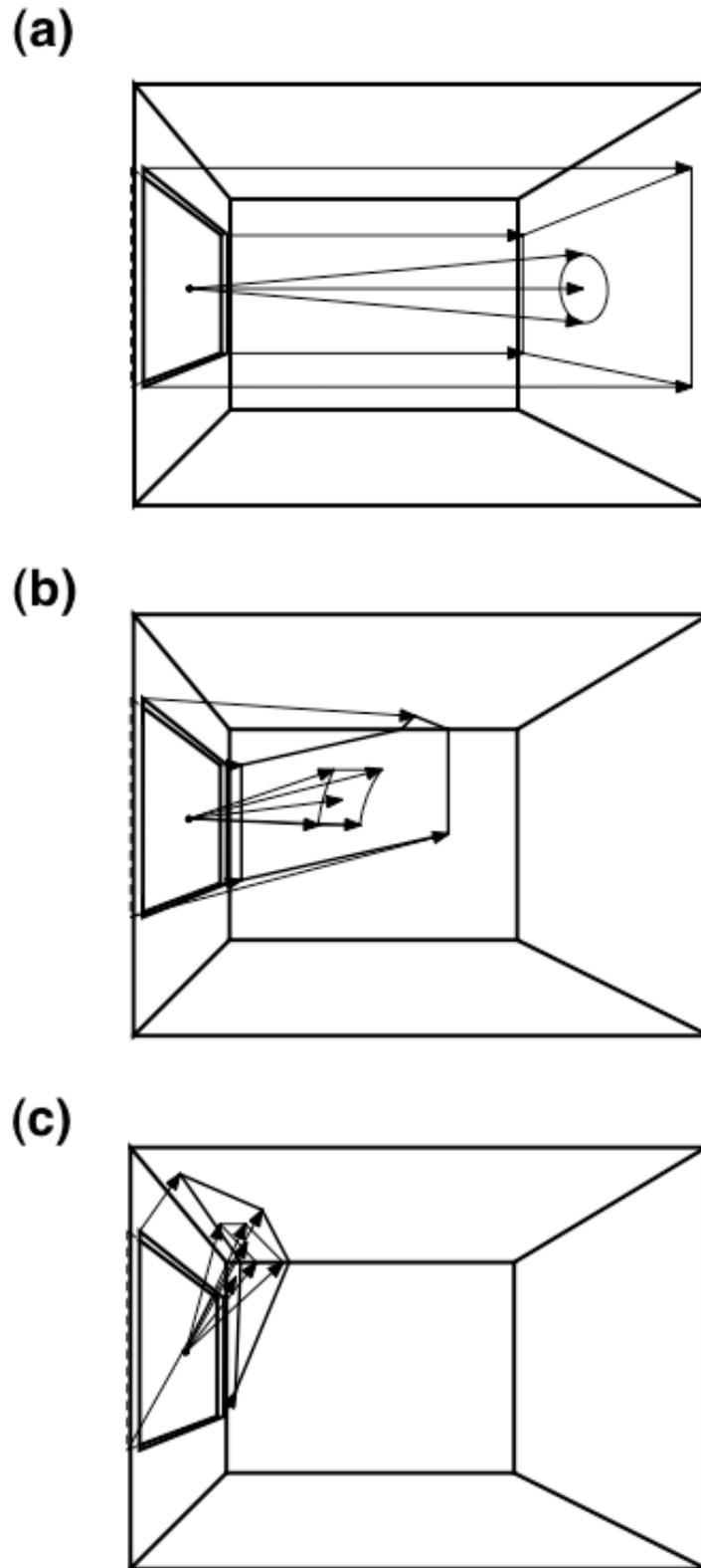
Figure 7.36: Transmitted Radiation in Three Directions for a Perimeter Office. (a)  $\theta = 0^\circ$ ; (b)  $\theta = 40^\circ$ ,  $\phi = 15^\circ$ ; (c)  $\theta = 70^\circ$ ,  $\phi = 67.5^\circ$ .  $\theta$  and  $\phi$  are the normal spherical angle coordinates in a right-handed coordinate system where  $y$  points up and  $z$  is normal to the window  $p$
