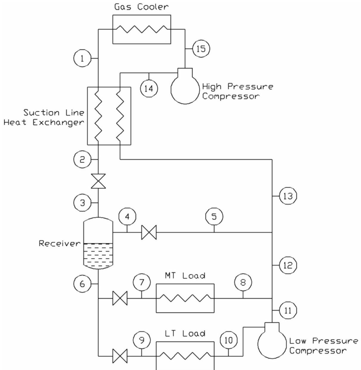
Figure 18.26: Schematic of the Transcritical CO<sub>2</sub> Booster Refrigeration Cycle.
