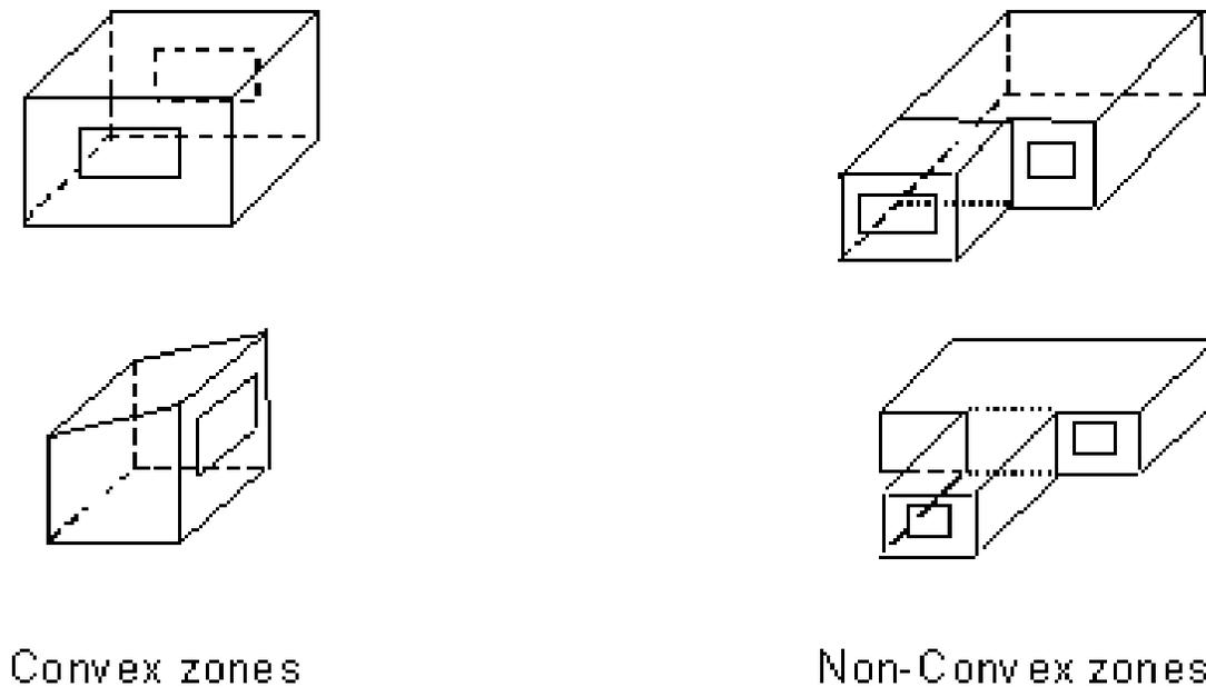
Figure 5.13: Illustration of Convex and Non-convex Zones
