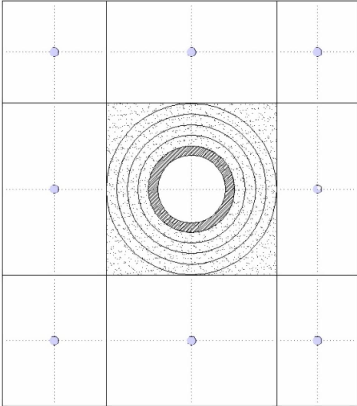
Figure 17.5: Radial "near-pipe" cell within a Cartesian cell
