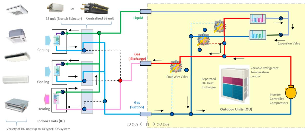
Figure 16.66: Schematic chart of a 3-pipe VRF-HR system
