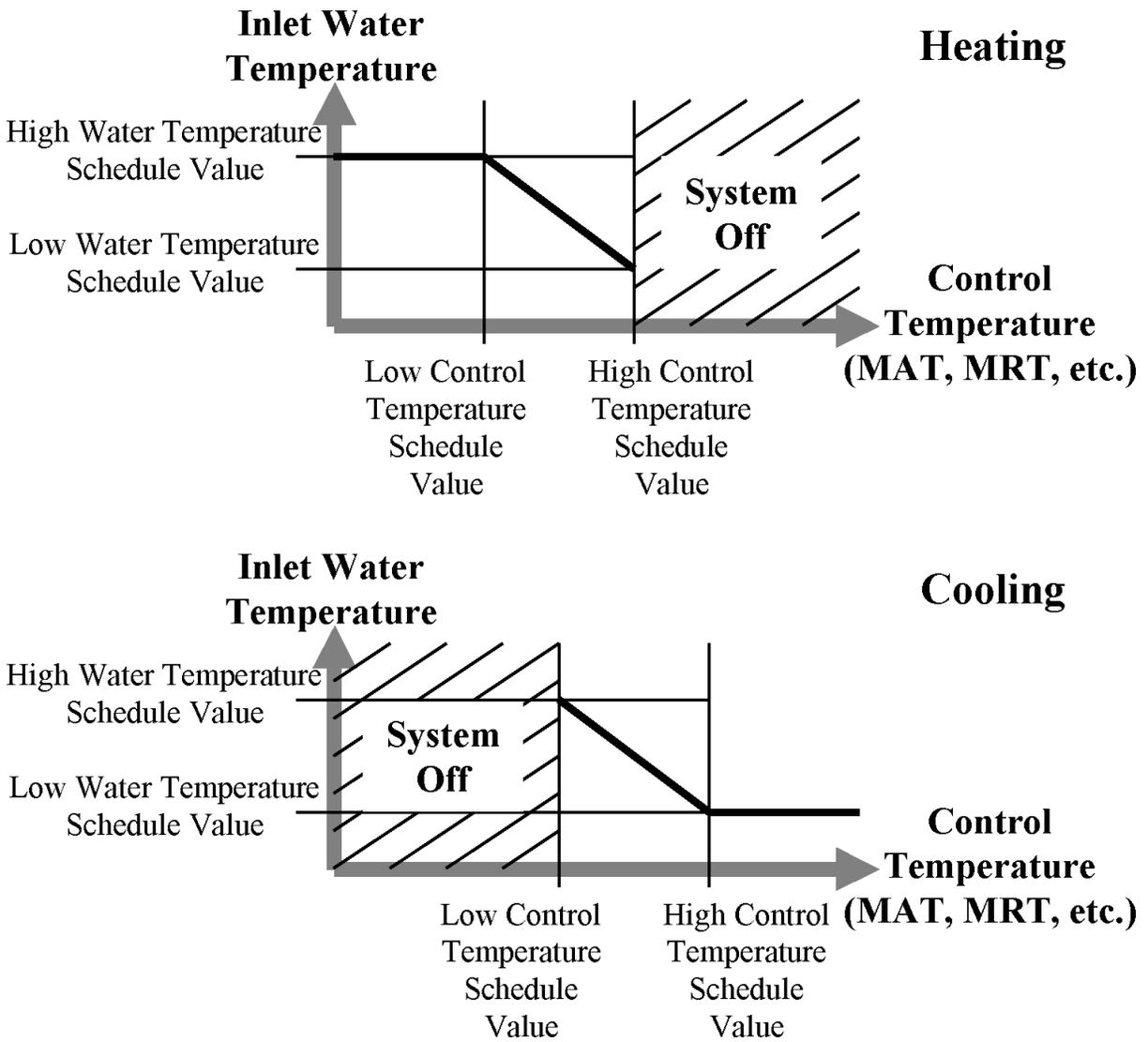
Figure 18.10: Variable Temperature Low Temperature Radiant System Controls
