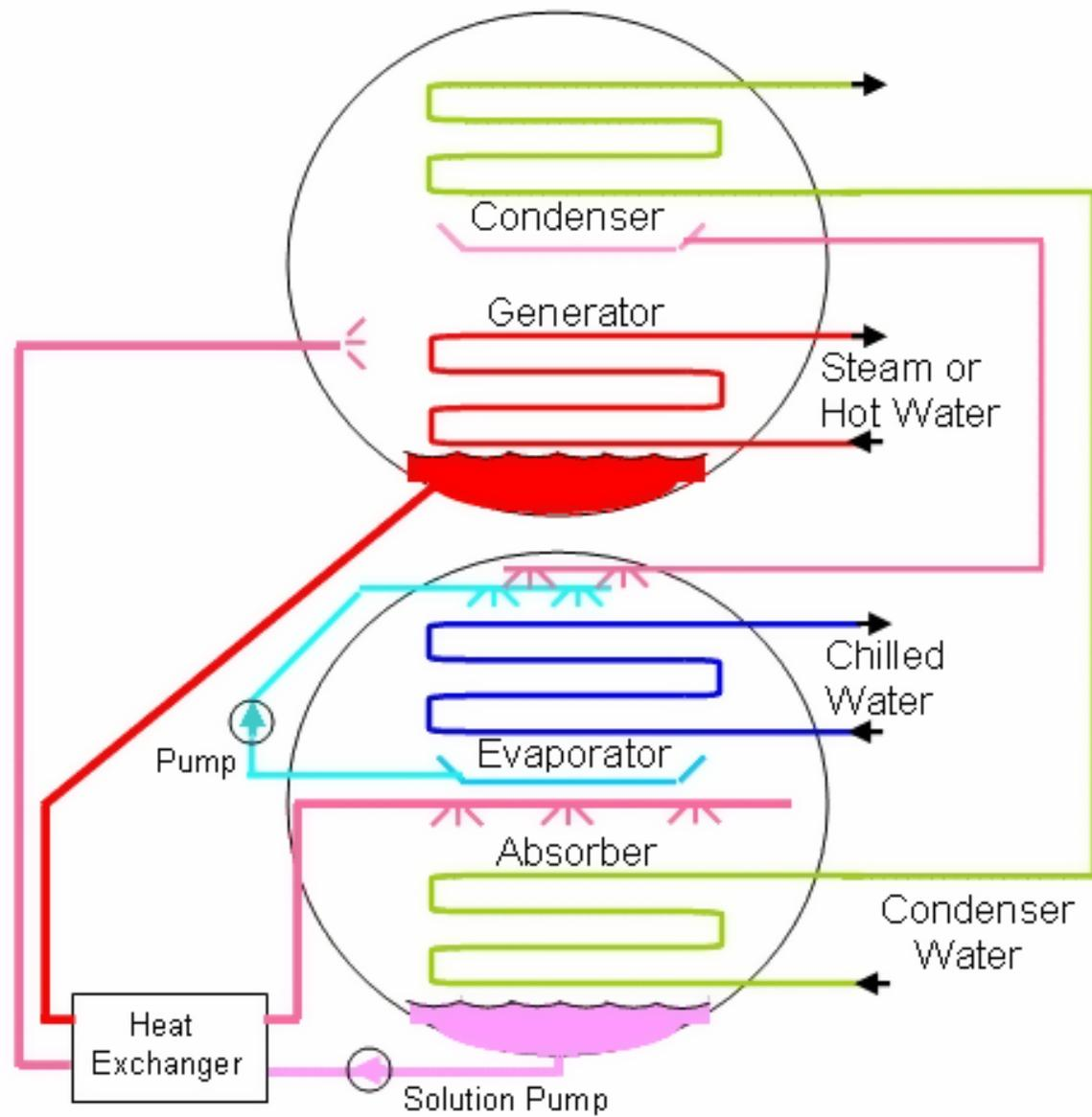
Figure 14.10: Schematic Diagram of a Single-Stage Absorption Chiller
