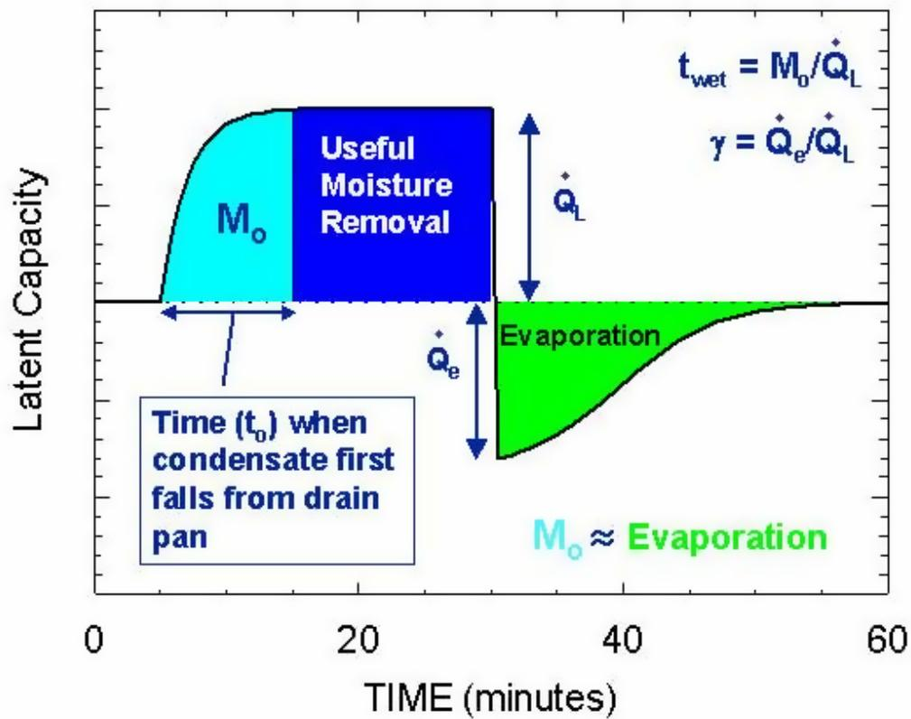
Figure 15.9: Concepts of Moisture Buildup and Evaporation
