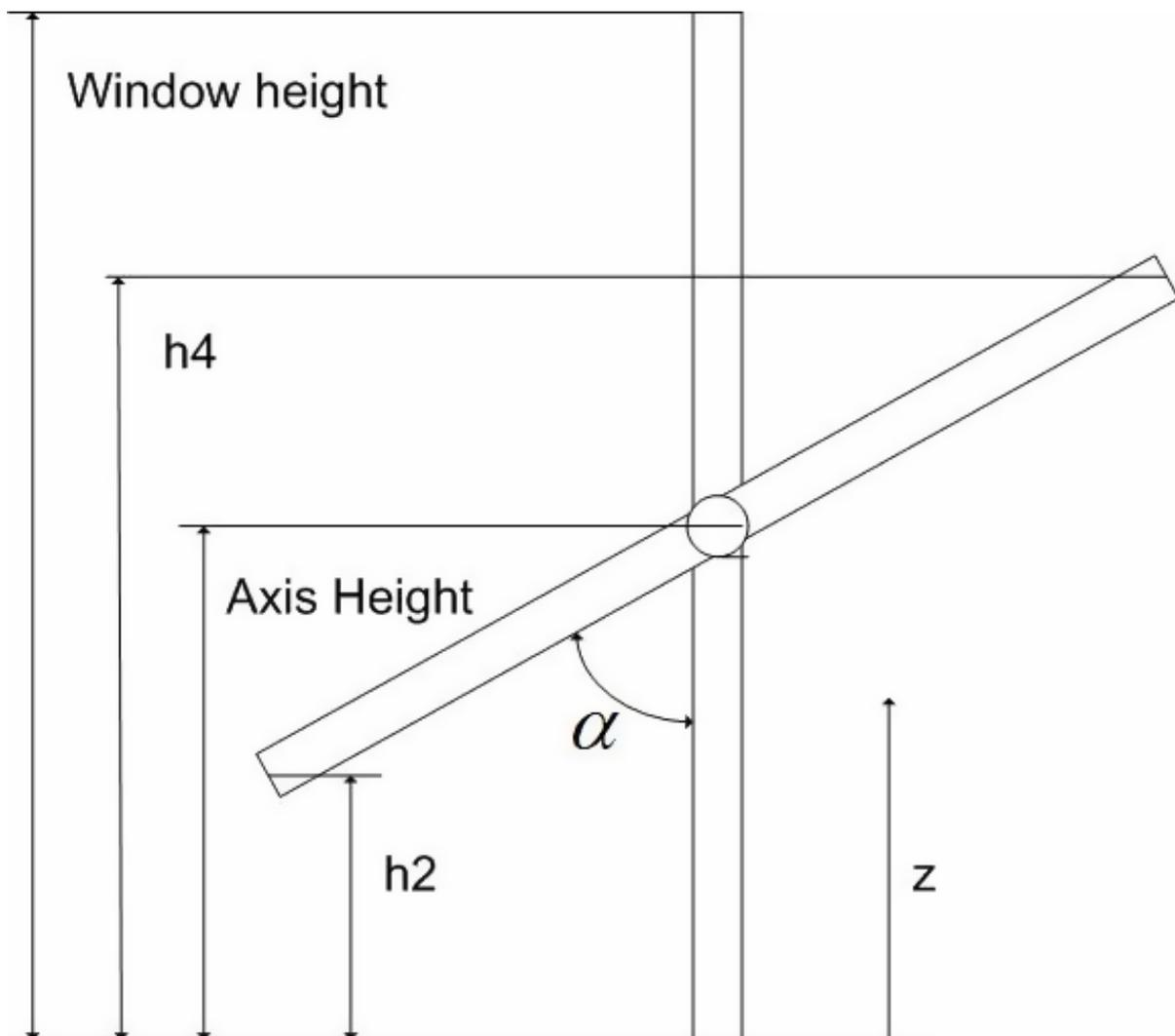
Figure 13.2: Schematic drawing of a horizontally-pivoted window
