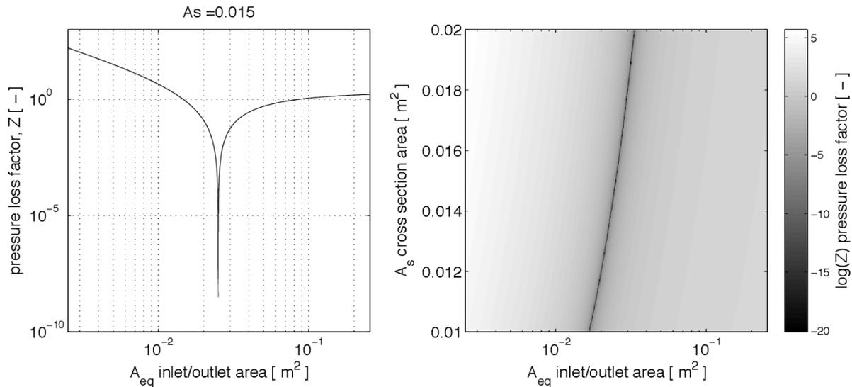
Figure 7.51: Pressure loss factor,  $Z$ , as a function of  $A_{eq}$  at  $A_s = 0.015m^2$ ; and (b) surface plot of  $Z$  as a function of  $A_s$  and  $A_{eq}$  for a 1m x 1m window. The minimum follows the predicted ratio of 5/3 between  $A_{eq}$  and  $A_s$ .
