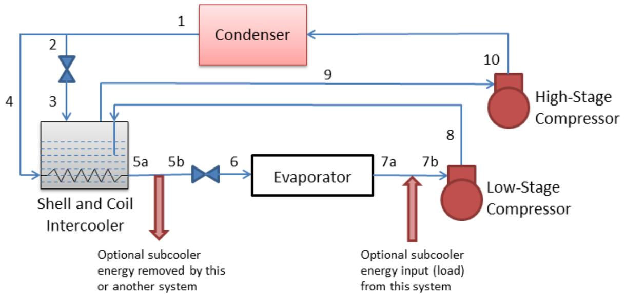
Figure 18.18: Two-Stage Compression System with a Shell-and-Coil Intercooler.
