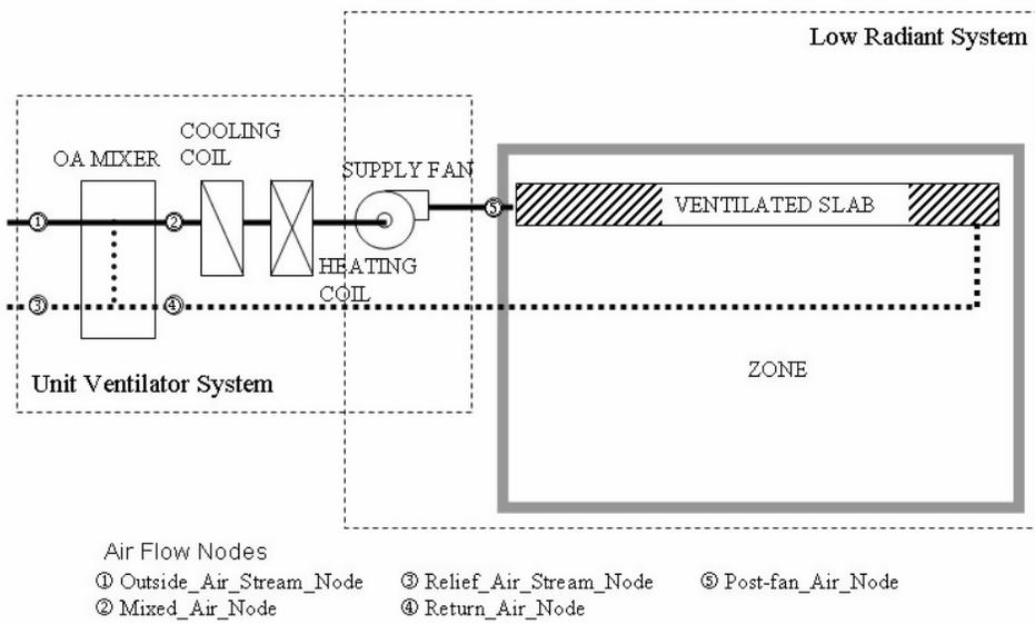
Figure 19.30: Basic System for the Ventilating Slab Module
