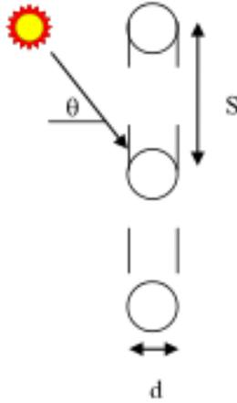
Figure 7.66: Geometry used for insect screen analysis
