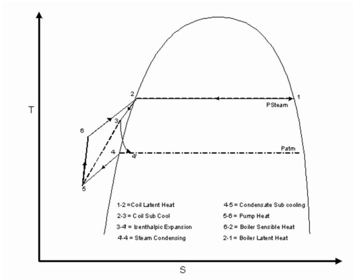
Figure 9.12: Schematic of Temperature – Entropy Diagram for Steam loop
