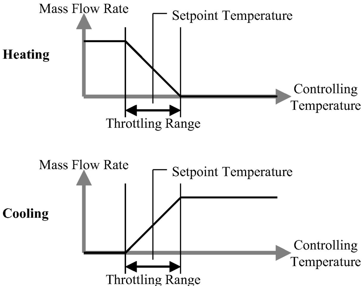
Figure 18.9: Variable Flow Low Temperature Radiant System Controls
