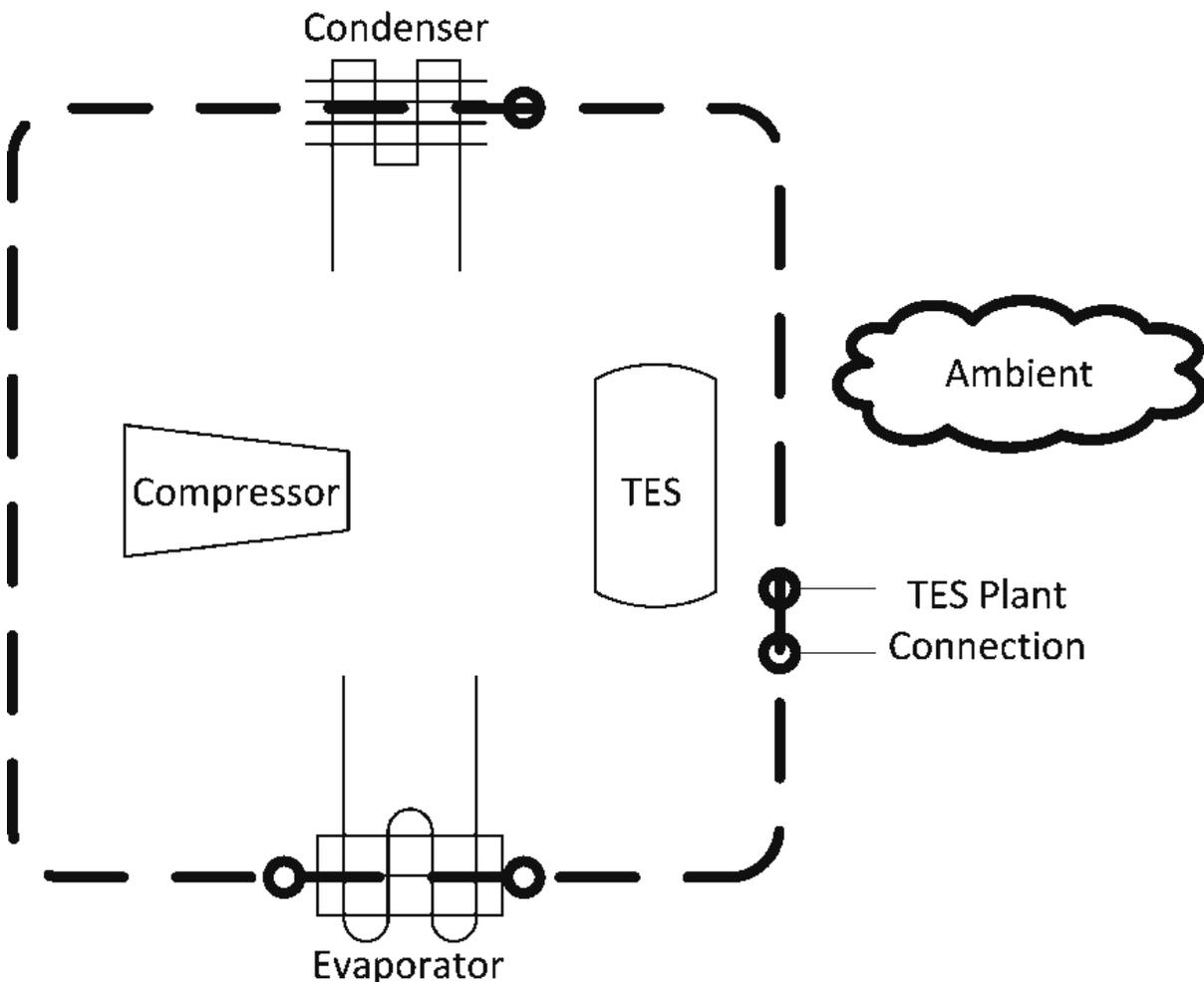
Figure 15.23: Highlights of Packaged Thermal Storage Cooling Coil
