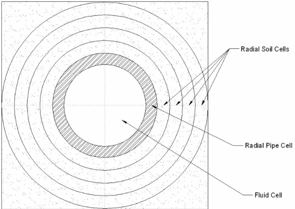
Figure 17.6: Close-up view of example radial cell
