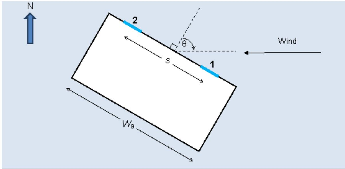
Figure 13.7: Plan view of building with 2-opening façade.
