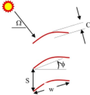
Figure 7.65: Geometry and properties used for venetian blind analysis. The effective longwave properties are obtained for the layer knowing longwave properties of the slats.
