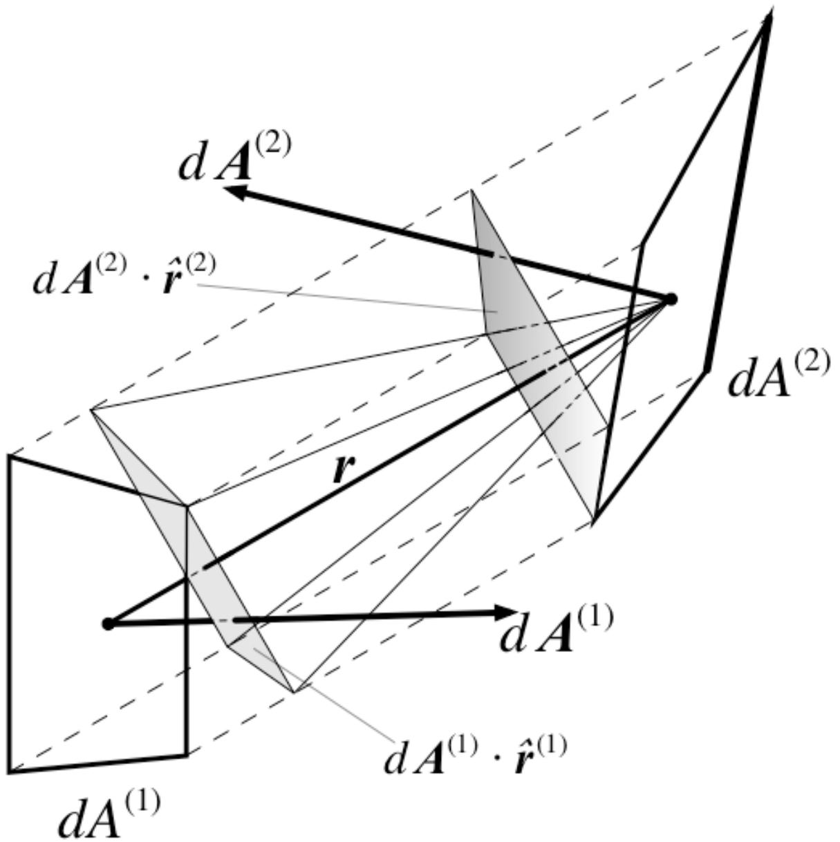
Figure 7.35: Radiation exchange between two surface elements
