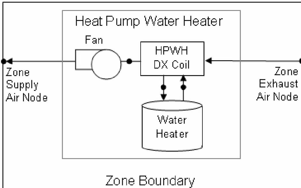
Figure 19.13: Schematic of a Heat Pump Water Heater with Inlet Air from a Zone
