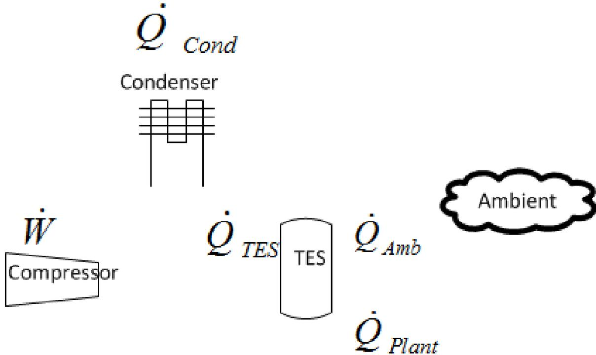
Figure 15.28: Thermal Storage Coil Charge Only Mode
