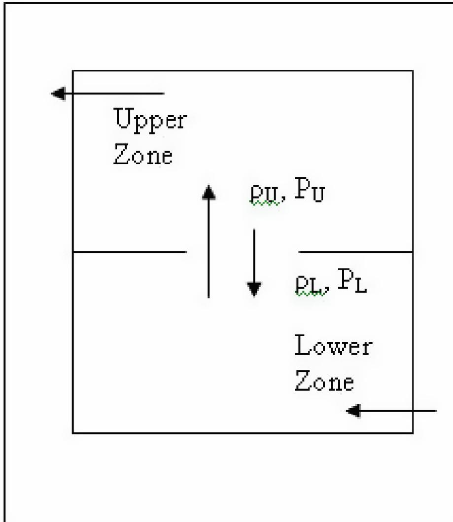
Figure 13.4: Air movements across a horizontal opening
