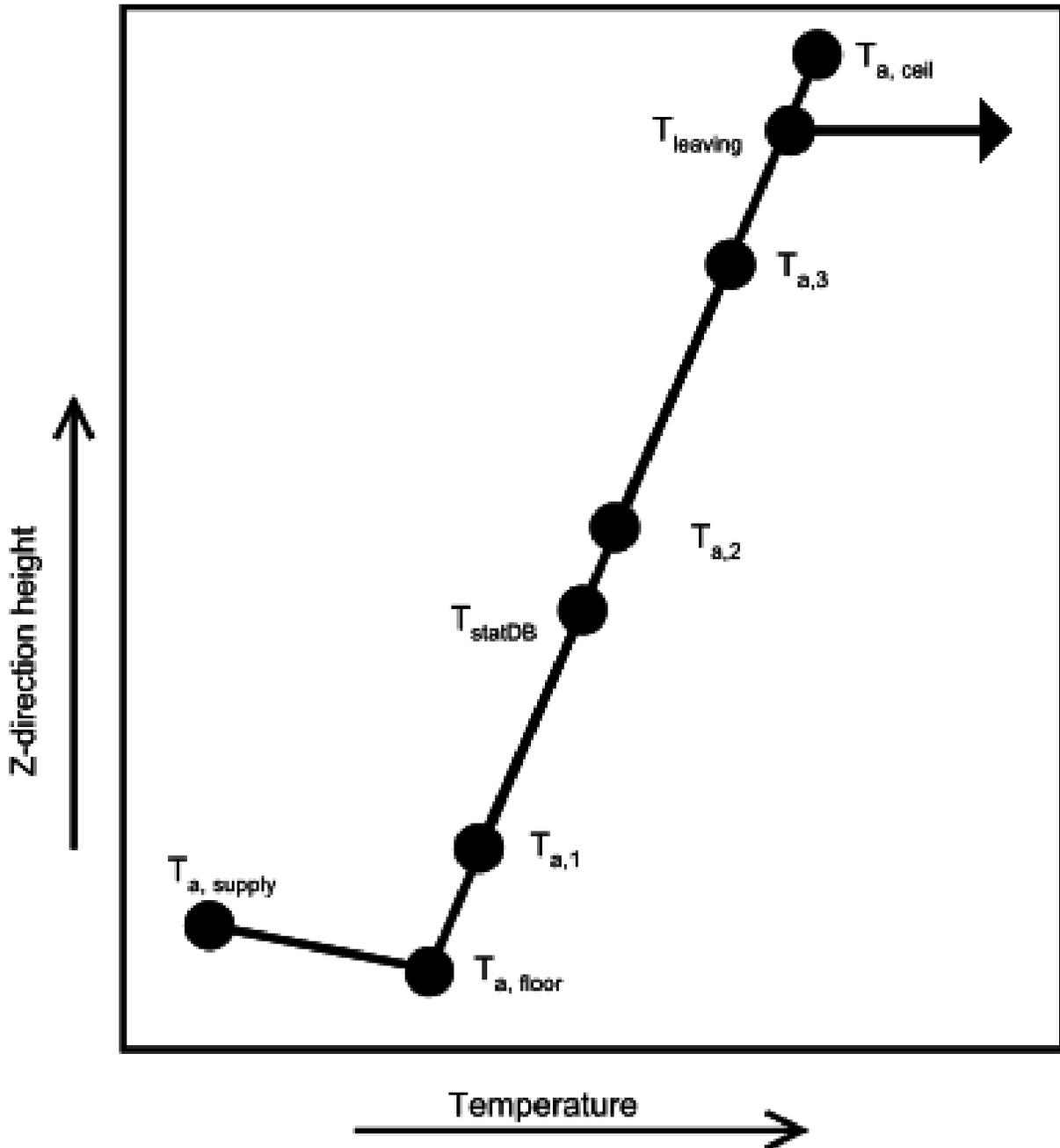
Figure 13.14: Height versus temperature schematic for Mundt model
