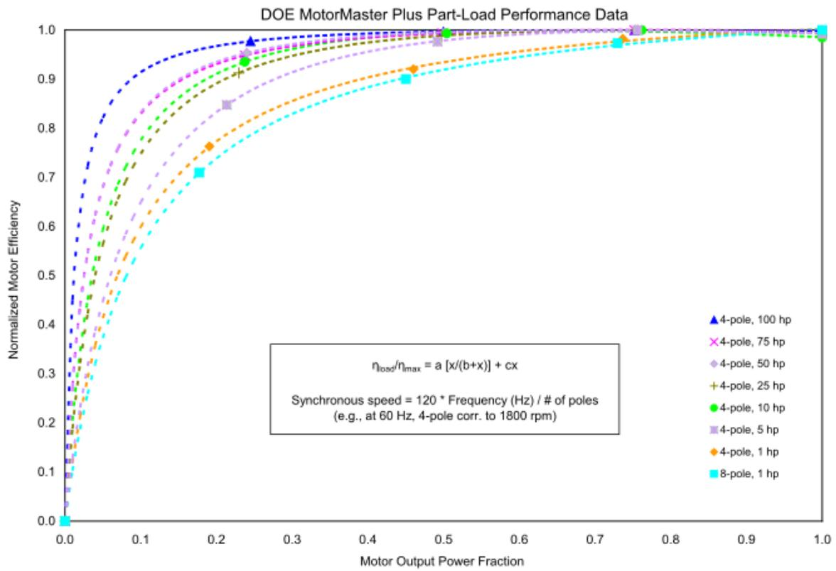
Figure 16.23: Motor Normalized Efficiency vs. Motor Load Fraction
