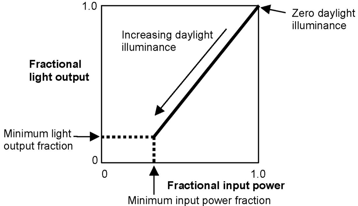
Figure 7.4: Control action for a continuous dimming system.
