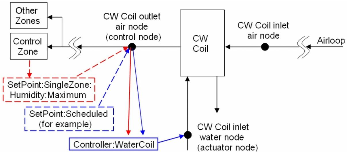
Figure 15.31: Two Setpoint managers used in Controller:WaterCoil
