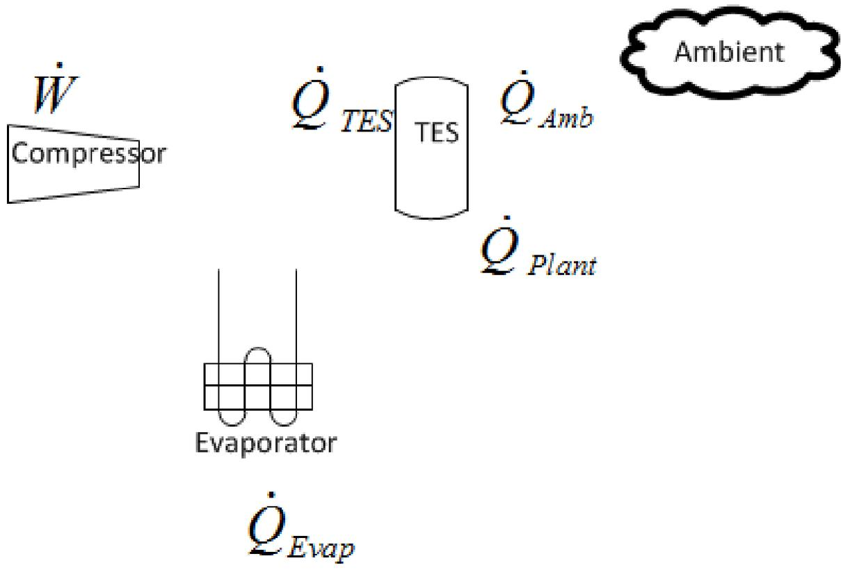
Figure 15.29: Thermal Storage Coil Discharge Only Mode
