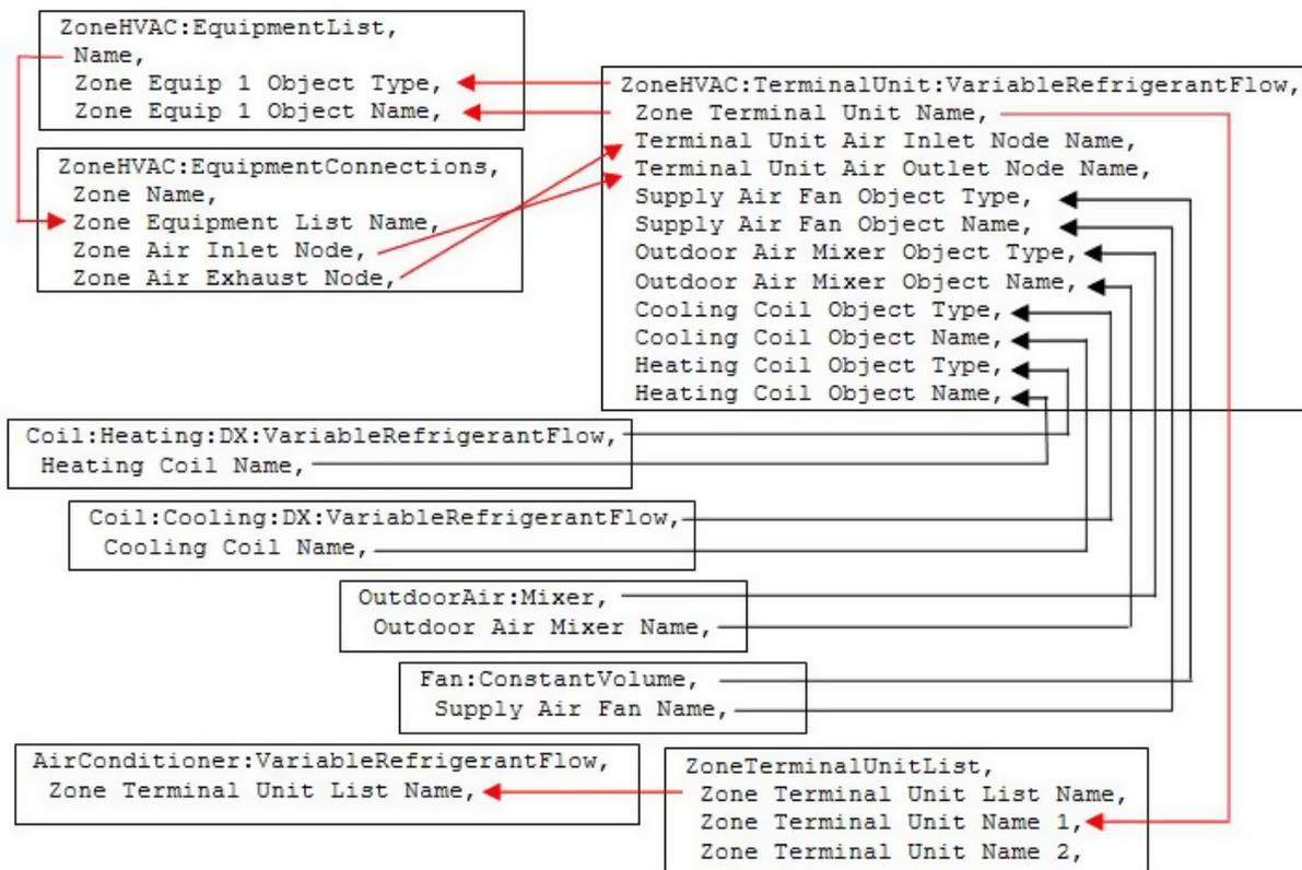
Figure 16.53: Energyplus object connections for VRF-SysCurve model
