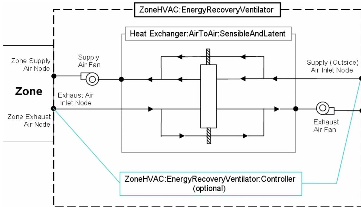
Figure 15.33: Schematic of the ZoneHVAC:EnergyRecoveryVentilator Compound Object
