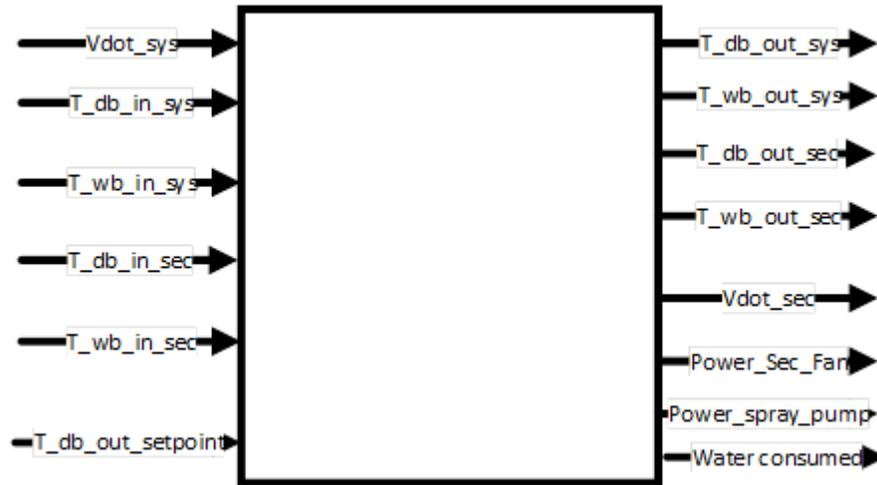
Figure 16.14: Research Special Indirect Evaporative Cooler Input/Output Model
