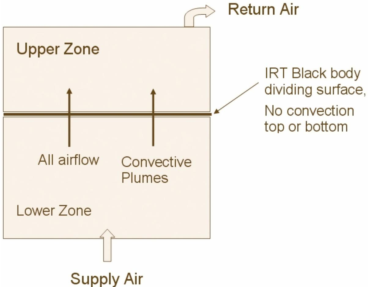
Figure 3.16: Schematic Model of a UFAD Zone
