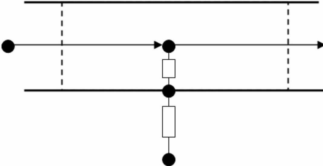
Figure 17.3: Control Volume drawn around node \*i\*
