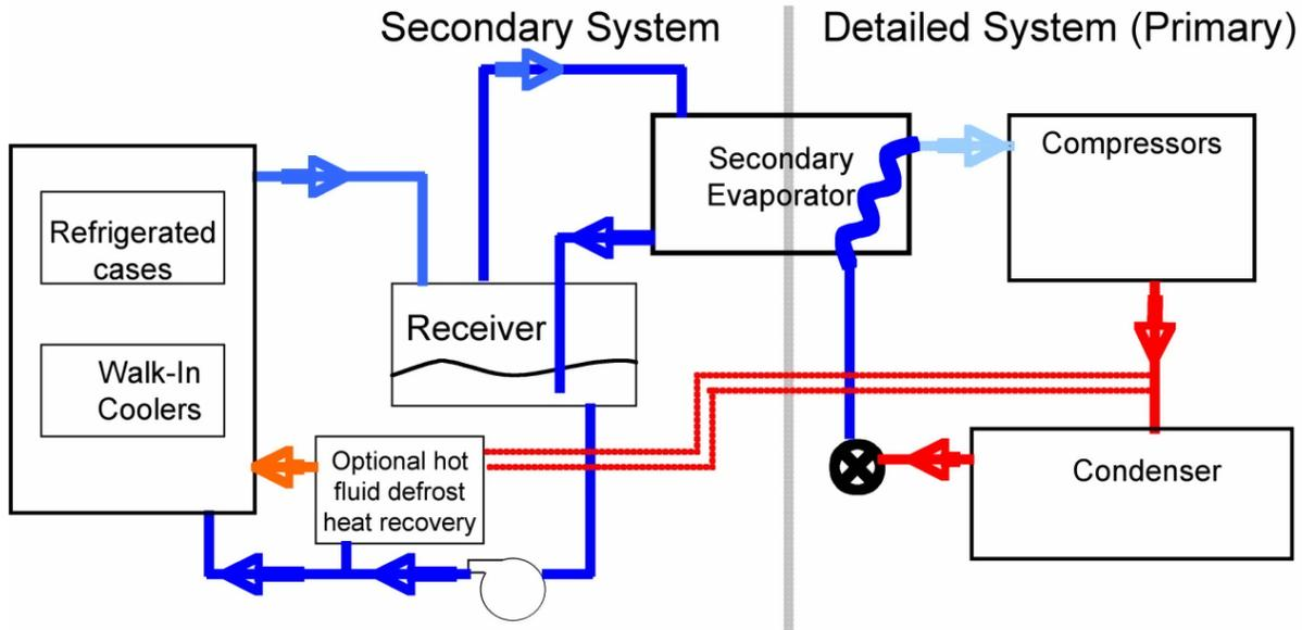
Figure 18.24: Secondary loop with liquid-overfeed refrigerant circulation
