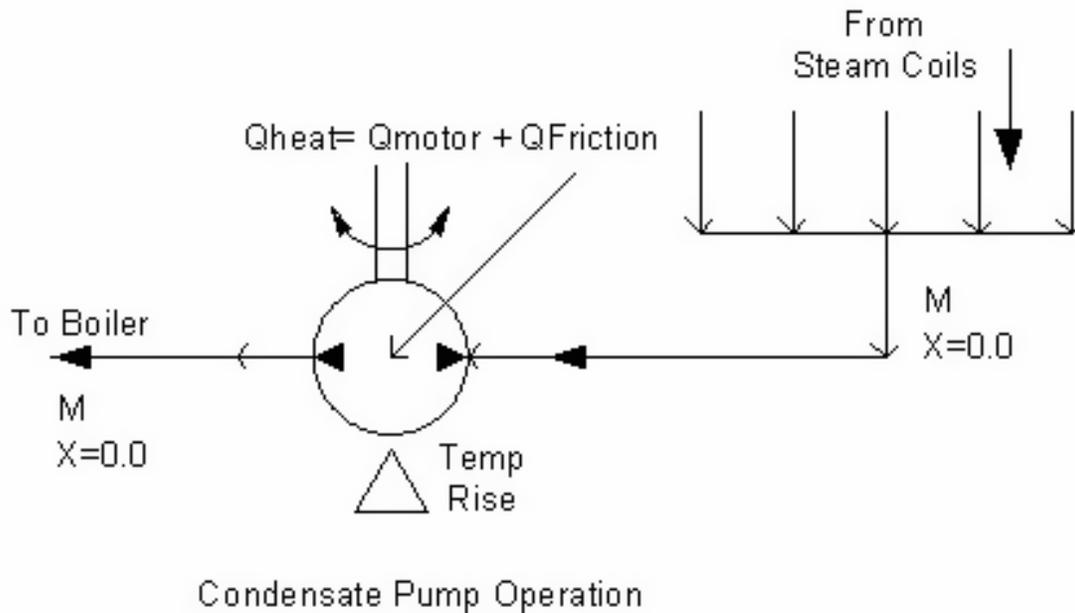
Figure 9.14: Schematic of Condensate Pump in Steam Loop
