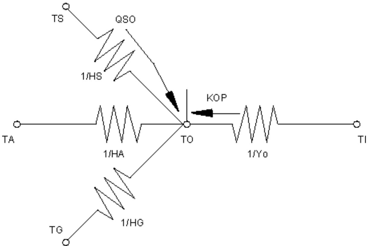
Figure 3.25: Thermal Network for Detailed Outside Surface Coefficient
