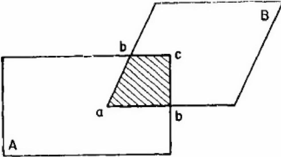
Figure 5.8: Point a – Vertex of A Enclosed by B
