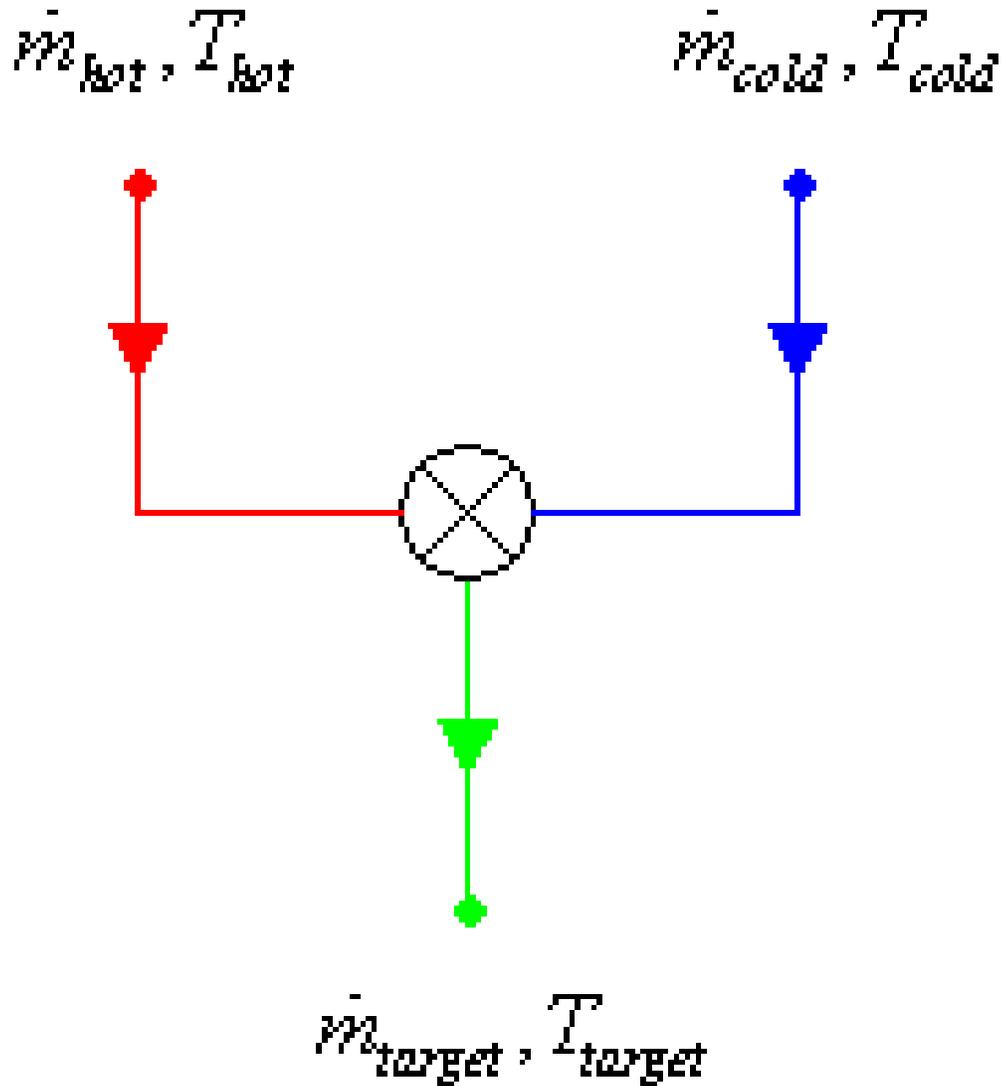
Figure 19.16: Hot and Cold Water Mixing
