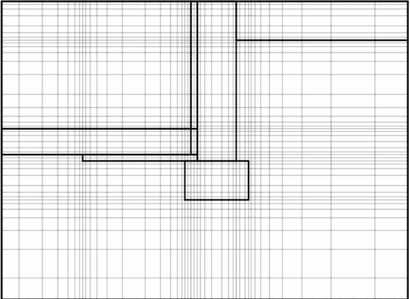
Figure 3.27: Example generated discretization near foundation perimeter
