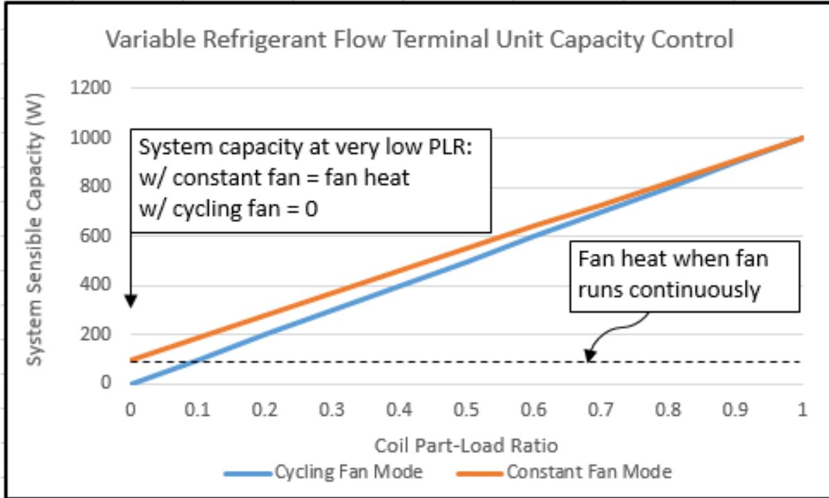
Figure 19.29: Variable Refrigerant Flow Terminal Unit Capacity Control
