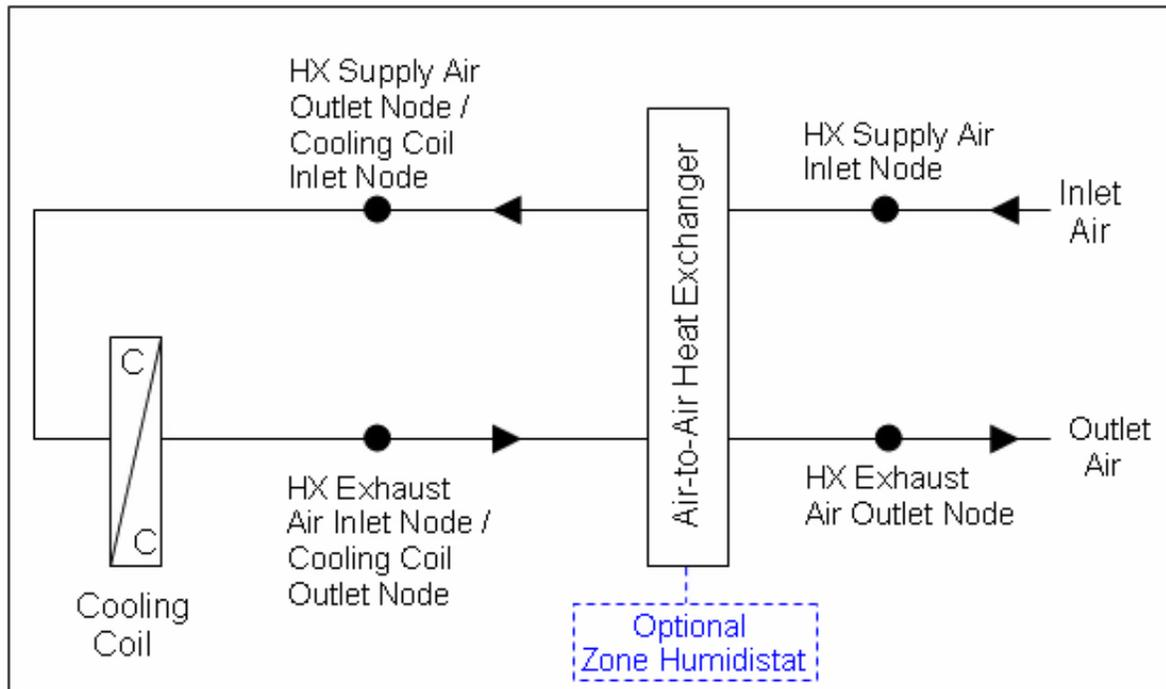
Figure 15.15: Schematic of a heat exchanger assisted DX cooling coil with optional humidistat
