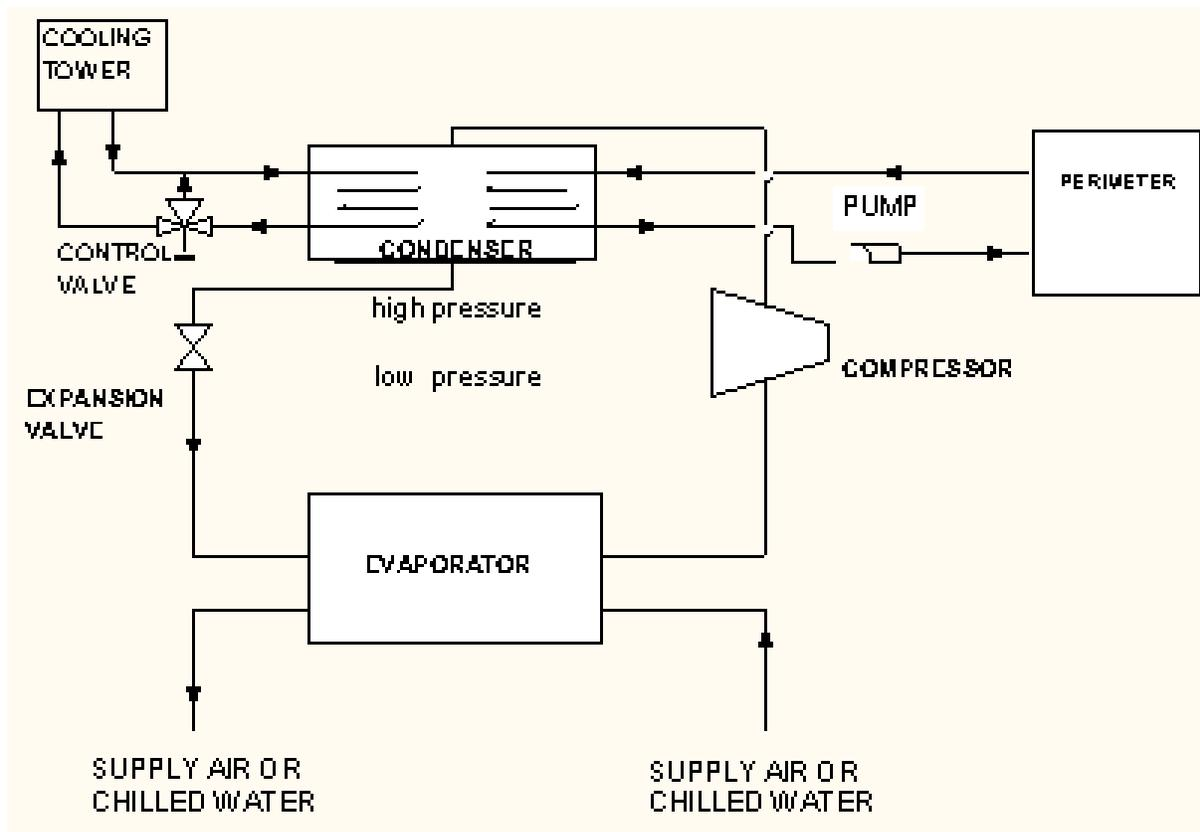
Figure 14.11: Diagram of Chiller:Electric with Heat Recovery
