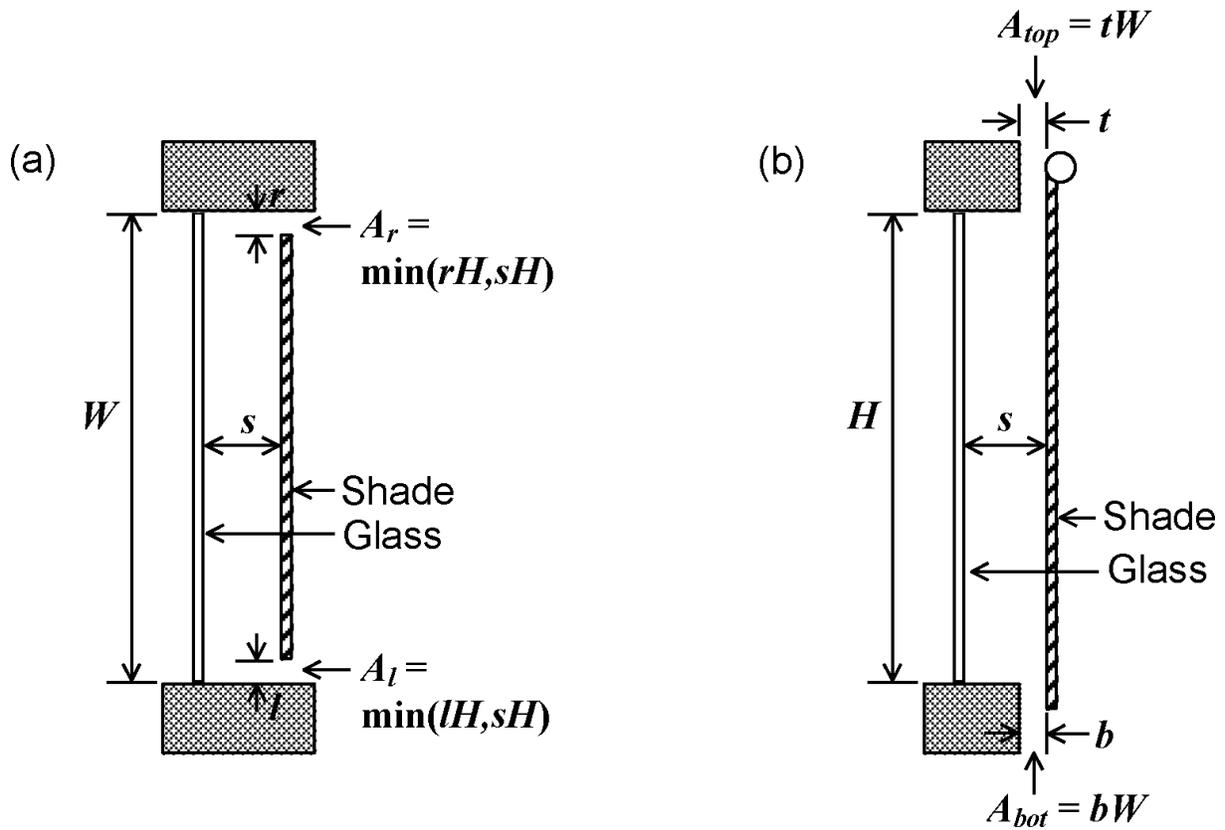
Figure 7.48: Examples of openings for an interior shading layer covering glass of height  $H$  and width  $W$ . Not to scale. (a) Horizontal section through shading layer with openings on the left and right sides (top view). (b) Vertical section through shading layer with openings at the top and bottom (side view).
