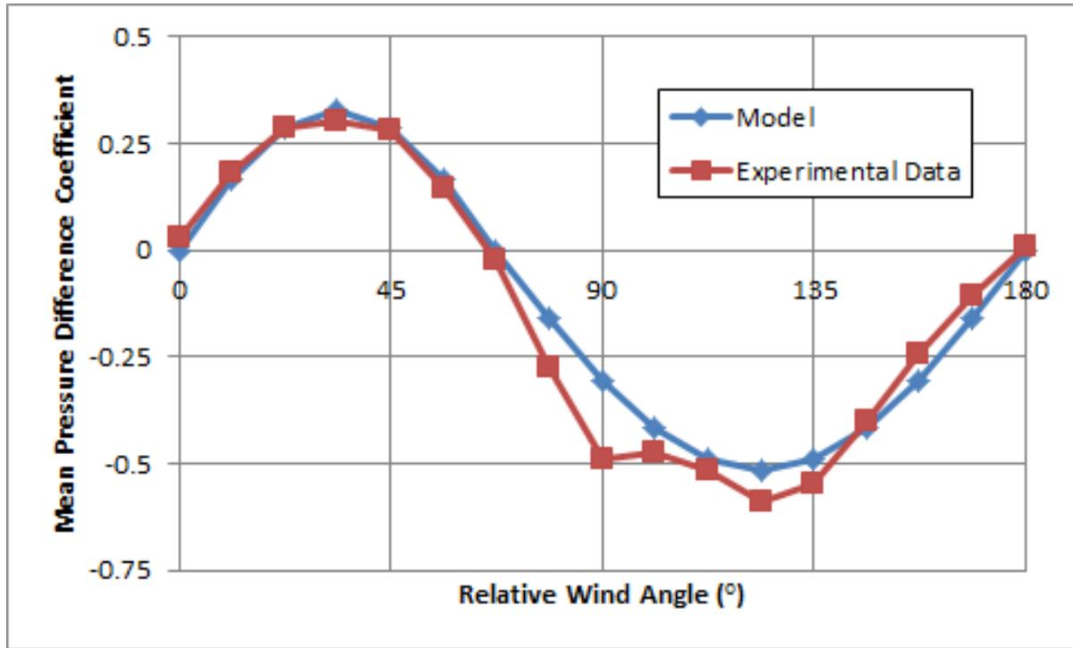
Figure 13.8: Mean pressure difference,  $\Delta c_p$  predicted by Equations 13.94 and 13.95, compared with experimental data. The façade containing the openings is facing South and the separation is large ( $s' = 0.85$ ).
