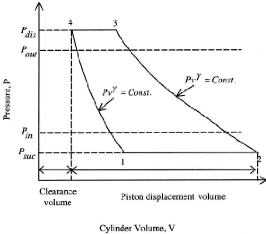
Figure 16.48: Schematic indicator diagram for a reciprocating Compressor(Jin 2002)
