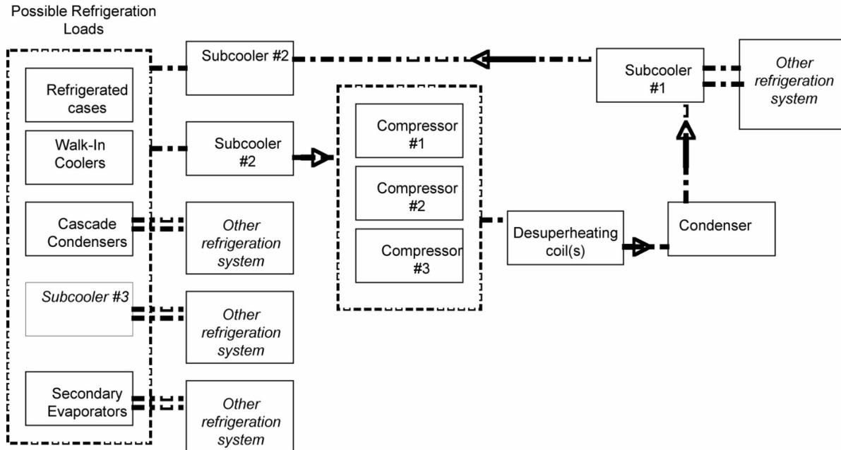
Figure 18.14: Typical Detailed Refrigeration System Equipment Schematic
