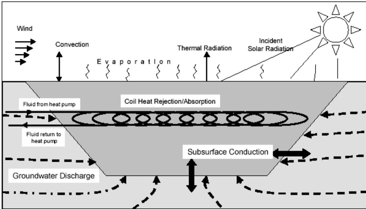
Figure 16.79: Heat Transfer Mechanisms in a Pond (Chiasson 1999)
