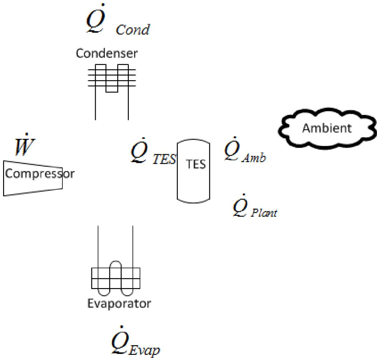
Figure 15.26: Thermal Storage Coil Cool and Charge Modes
