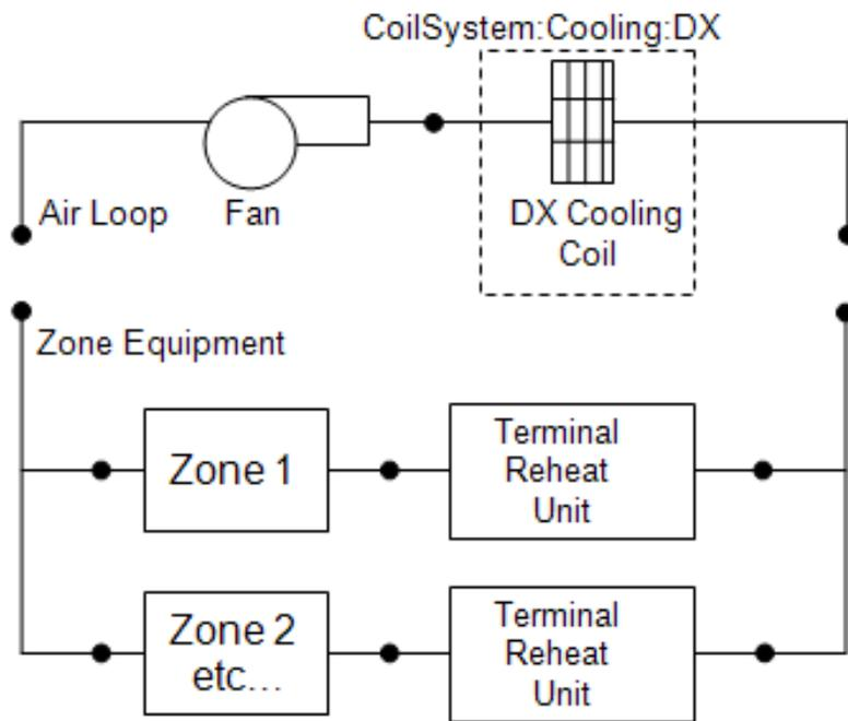
Figure 16.40: Schematic of Packaged DX Cooling Subsystem in Air Loop for a Blow-Thru Application
