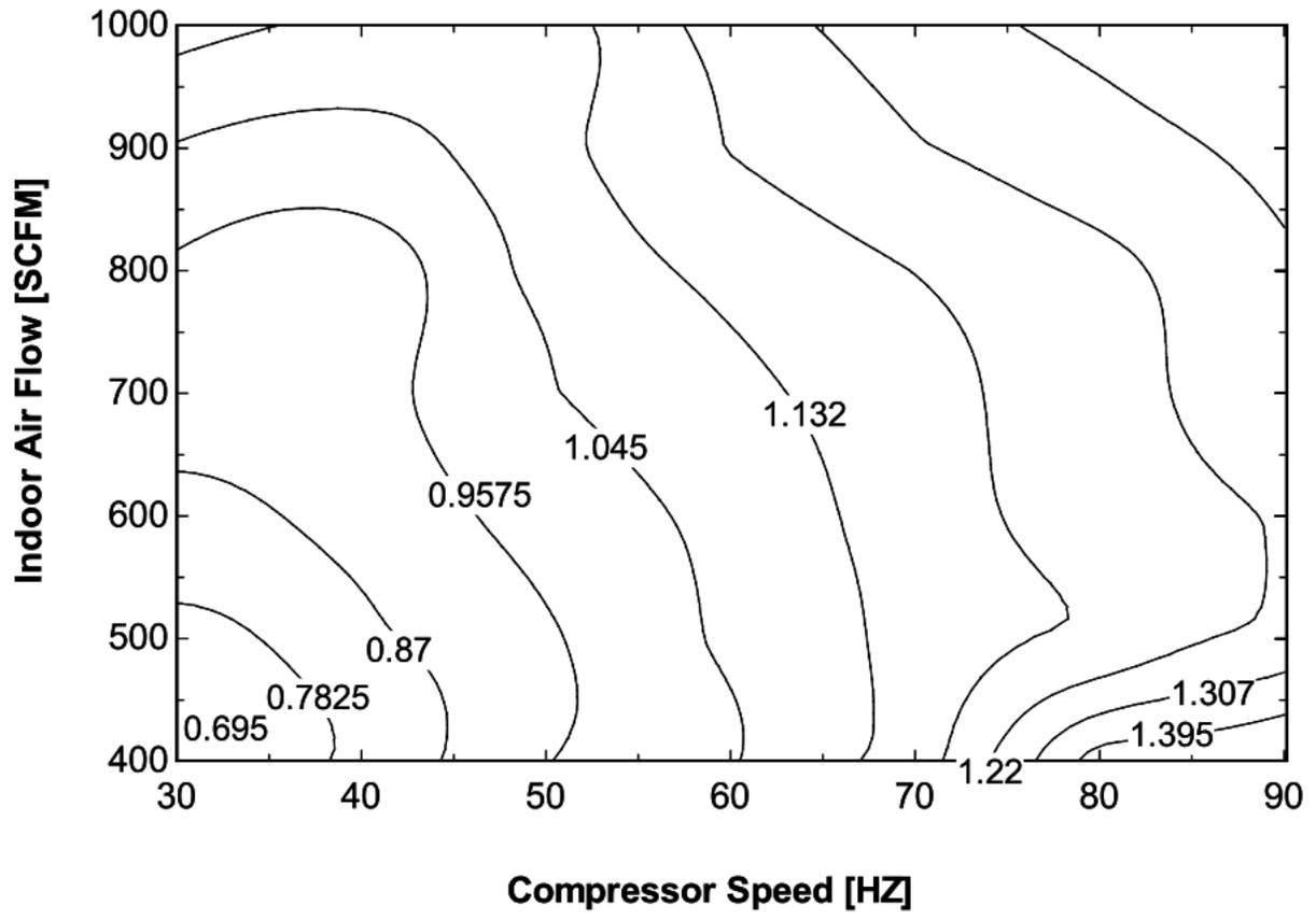
Figure 15.19: Effective Surface Area ( $A_o$ ) Changing with Compressor Speed and Indoor SCFM
