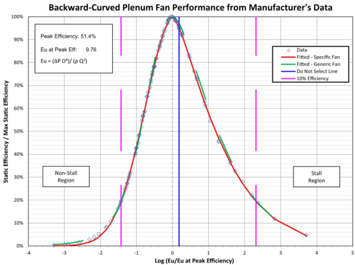
Figure 16.18: Example Normalized Efficiency Data for One Fan
