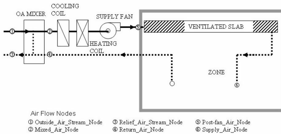
Figure 19.32: Zone Supply Model using Ventilated Slab (Slab and Zone mode)
