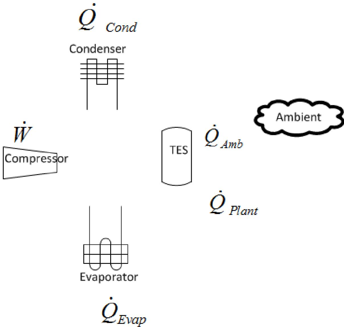
Figure 15.25: Thermal Storage Coil Cooling Only Mode
