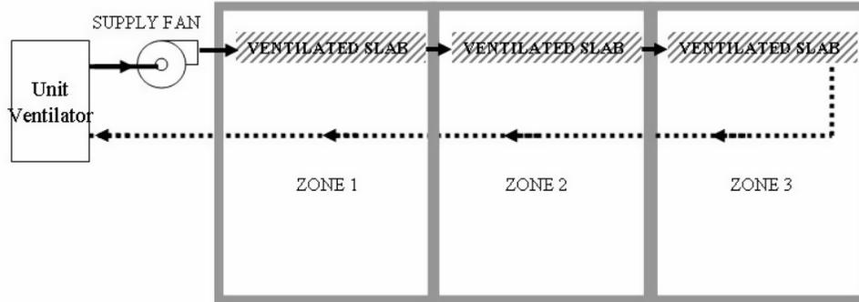
Figure 19.33: Multiple Slabs model with Several Zones (Series Slabs Mode)
