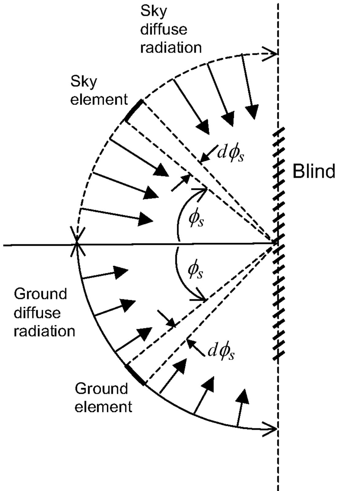
Figure 7.27: Side view of horizontal slats in a vertical blind showing geometry for calculating blind transmission, reflection and absorption properties for sky and ground diffuse radiation.
