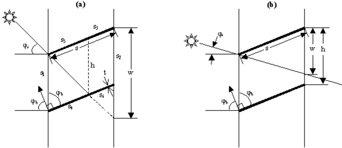
Figure 7.22: (a) Side view of a cell formed by adjacent slats showing how the cell is divided into segments,  $s_i$ , for the calculation of direct solar transmittance; (b) side view of a cell showing case where some of the direct solar passes between adjacent slats without touching either of them. In this figure  $\phi_s$  is the profile angle and  $\phi_b$  is the slat angle.
