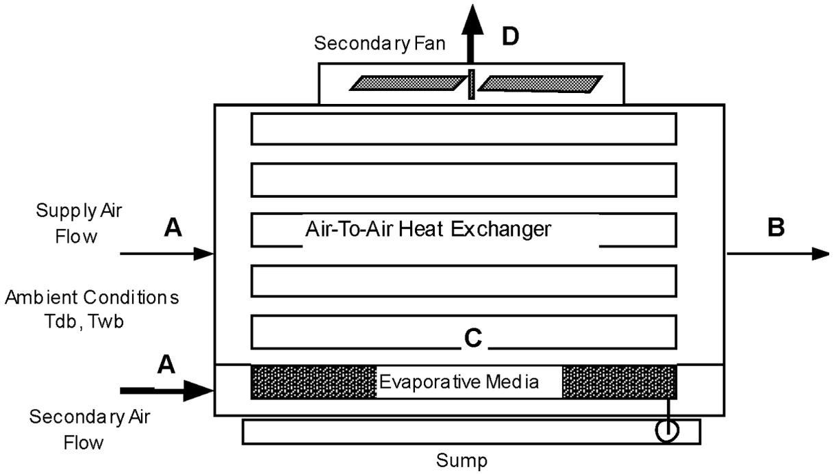
Figure 16.7: Evaporative Cooler – Indirect Dry Coil
