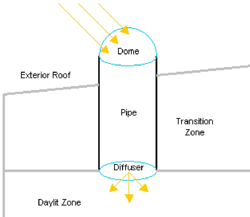
Figure 7.10: Tubular Daylighting Devices
