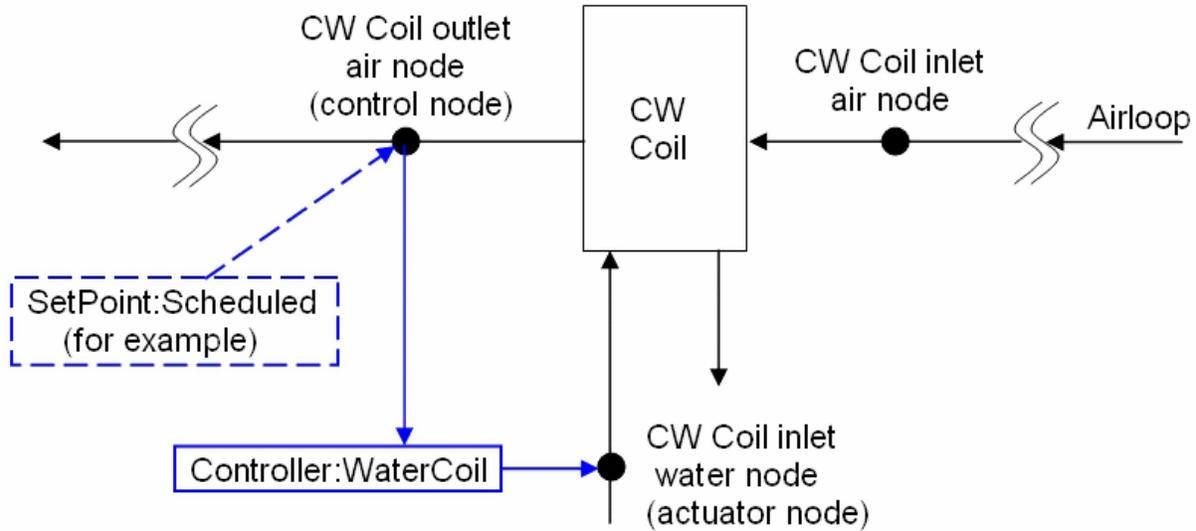
Figure 15.30: Controller:WaterCoil used with Central Chilled Water Coil
