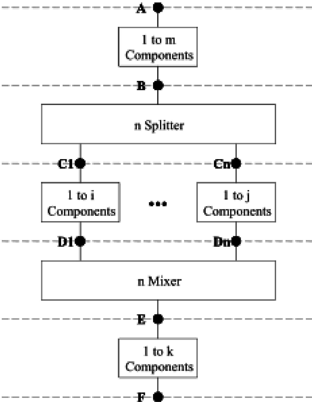
Figure 9.2: Branch Layout for Individual Plant Half-Loops
