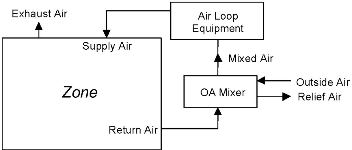
Figure 16.3: Demand Control Ventilation – Air Flow Paths
