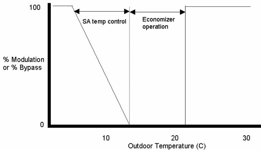
Figure 16.73: Air to Air Heat Exchanger with Supply Air Temperature Control
