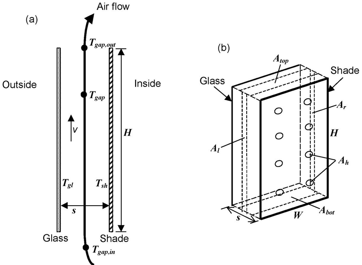
Figure 7.47: Vertical section (a) and perspective view (b) of glass layer and interior shading layer showing variables used in the gap airflow analysis. The opening areas  $A_{bot}$ ,  $A_{top}$ ,  $A_l$ ,  $A_r$  and  $A_h$  are shown schematically.
