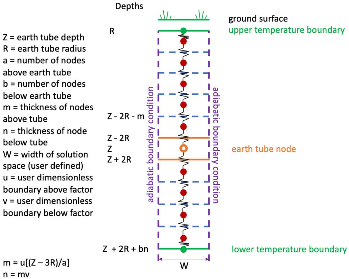
Figure 19.35: Earth Tube Vertical Model Solution Space
