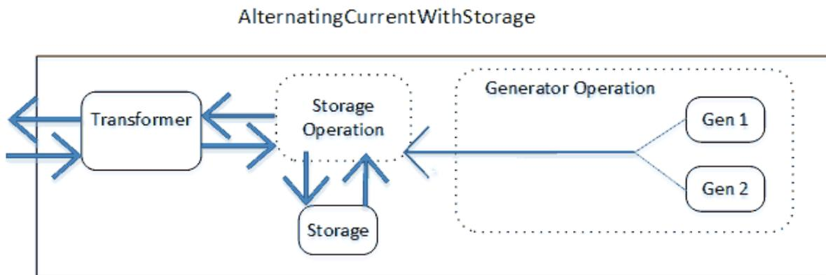
Figure 20.2: AC Generators with On-site Electrical Storage Schematic
