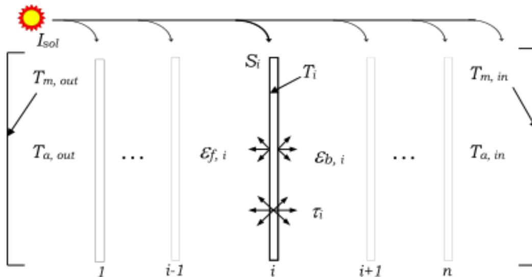
Figure 7.60: Multi-layer fenestration analysis structure (ASHRAE 1311-RP)
