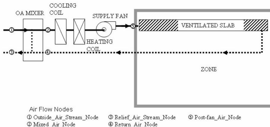
Figure 19.31: Model with Air Delivered to Slab (Slab Only Mode)
