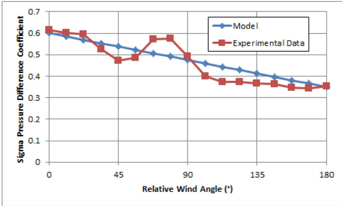
Figure 13.9: Standard deviation of pressure difference,  $\sigma_{\Delta c_p}$ , predicted by Equations 13.96 and 13.97, compared with experimental data. The façade containing the openings is facing South and the separation is large ( $s' = 0.85$ ).
