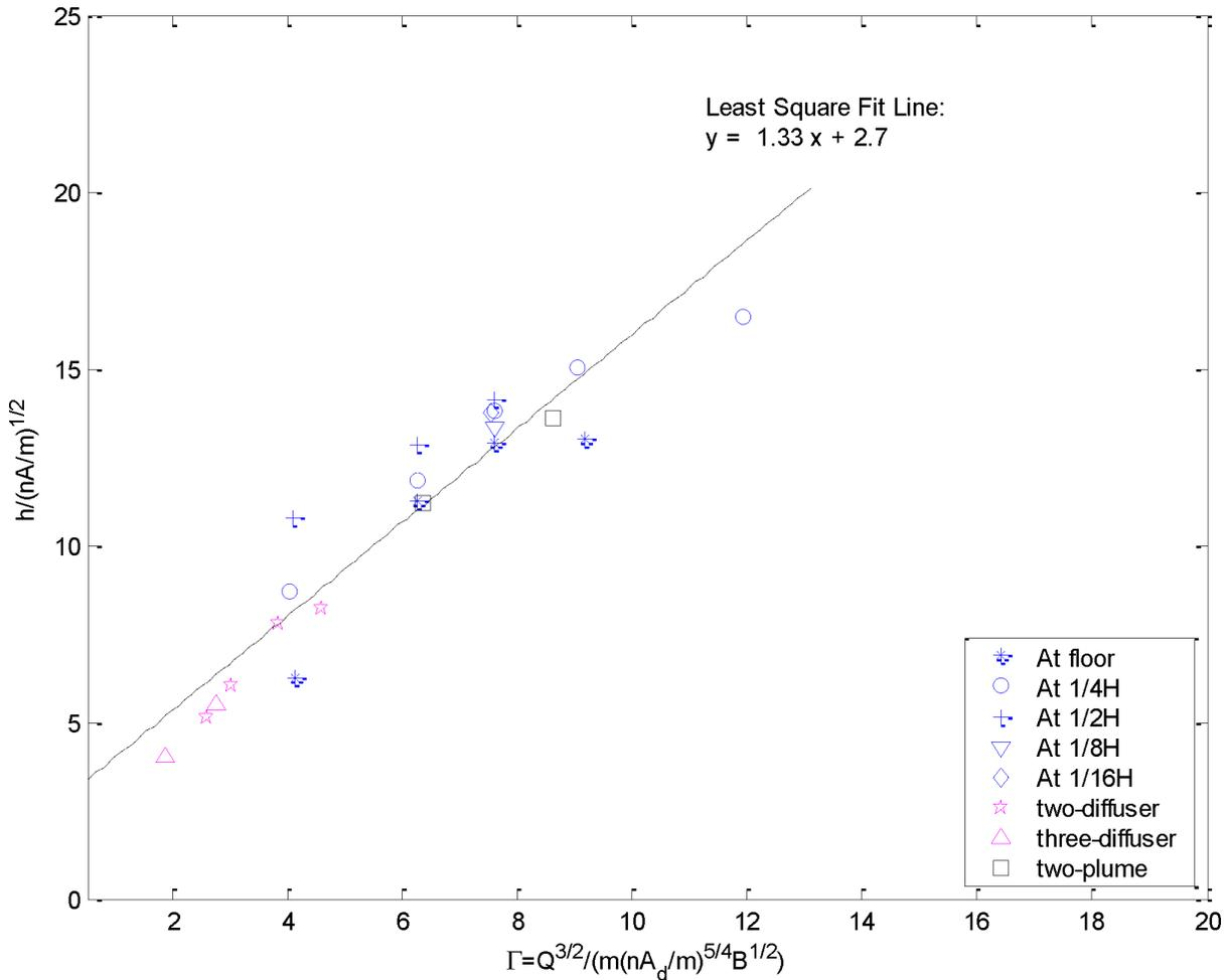
Figure 13.17: Non-dimensional interface height of small-scale experiments.
