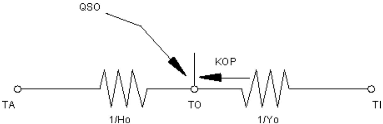
Figure 3.24: Thermal Network for Simple Outside Surface Coefficient
