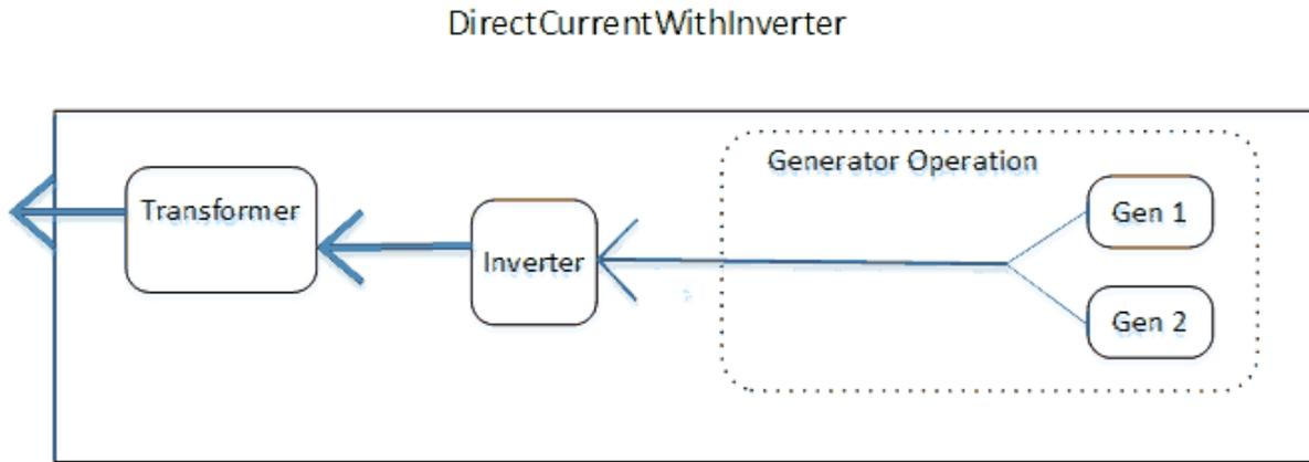
Figure 20.3: Direct Current With Inverter Photovoltaic Generators Schematic
