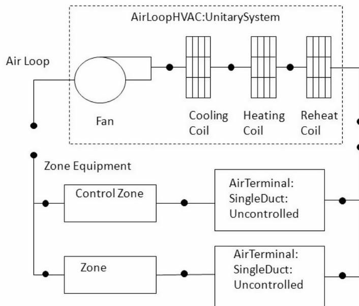
Figure 16.26: Schematic of the EnergyPlus Unitary System (Blow Through Configuration)
