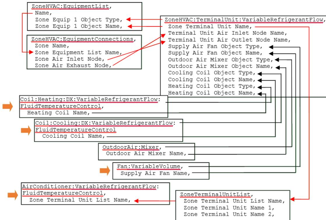
Figure 16.61: EnergyPlus object connections for VRF-FluidTCtrl model
