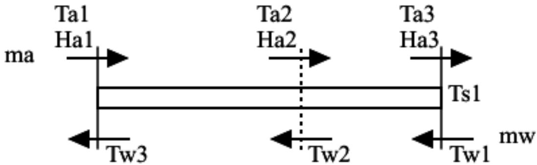
Figure 15.6: Simplified Schematic of Cooling/Dehumidifying Coil
