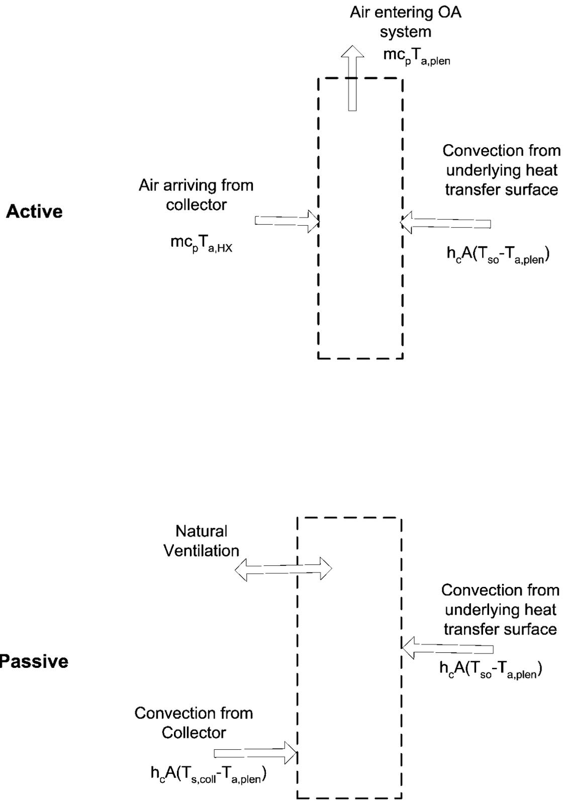
Figure 18.40: Transpired Collector Plenum Air Heat Balance
