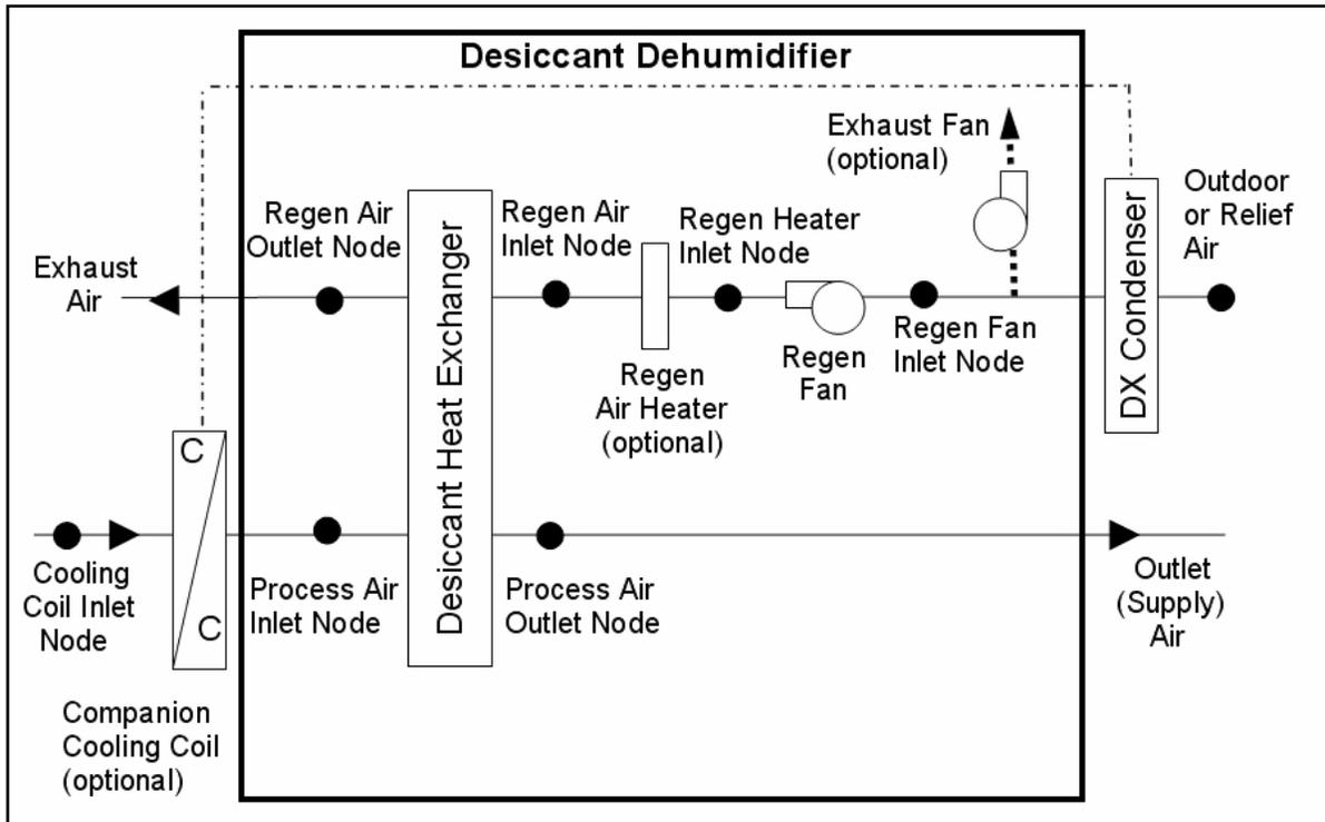
Figure 16.41: Schematic of a Desiccant Dehumidifier with Draw Through Regeneration Fan Placement
