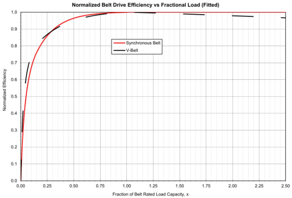
Figure 16.21: Belt Normalized Efficiency vs. Belt Fractional Load)
