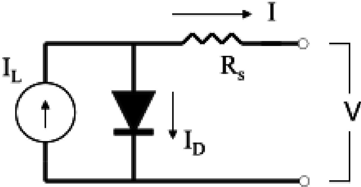
Figure 20.8: Equivalent circuit in the four parameter model
