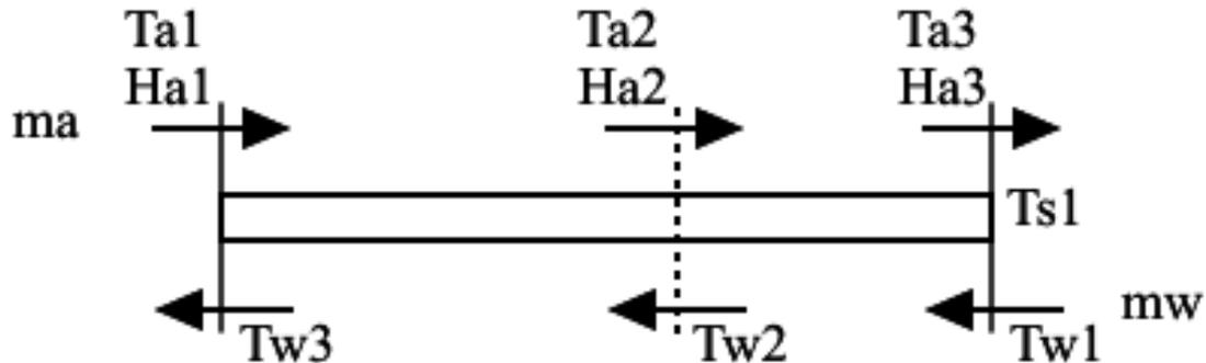
Figure 15.1: Simplified Schematic of Cooling/Dehumidifying Coil
