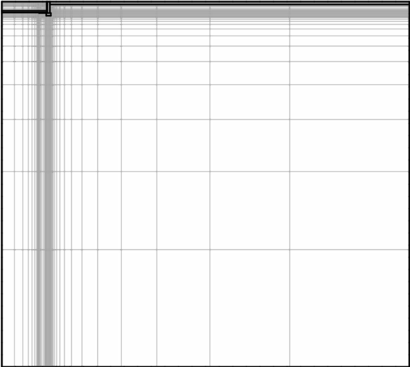
Figure 3.28: Example generated discretization of full domain
