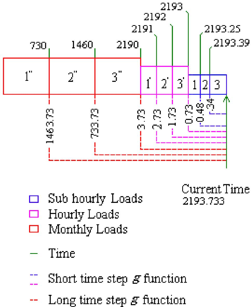
Figure 16.76: Schematic of Variable Time Step Model  $g$  Function Calculation.
