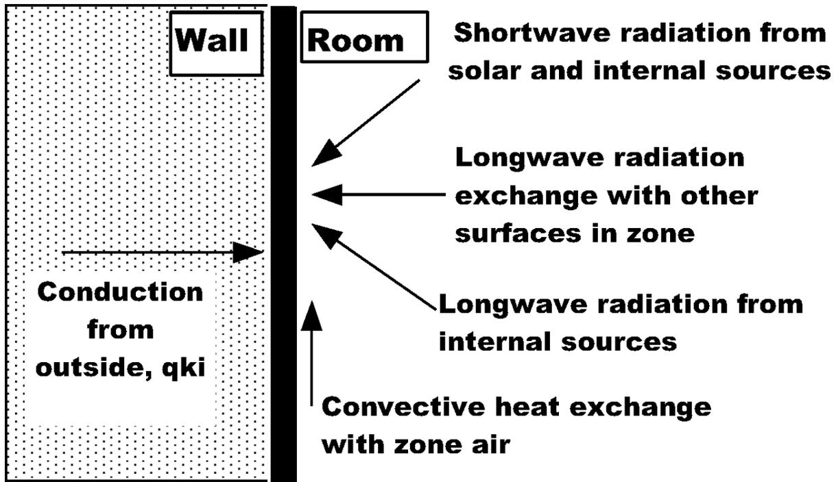
Figure 3.11: Inside Heat Balance Control Volume Diagram
