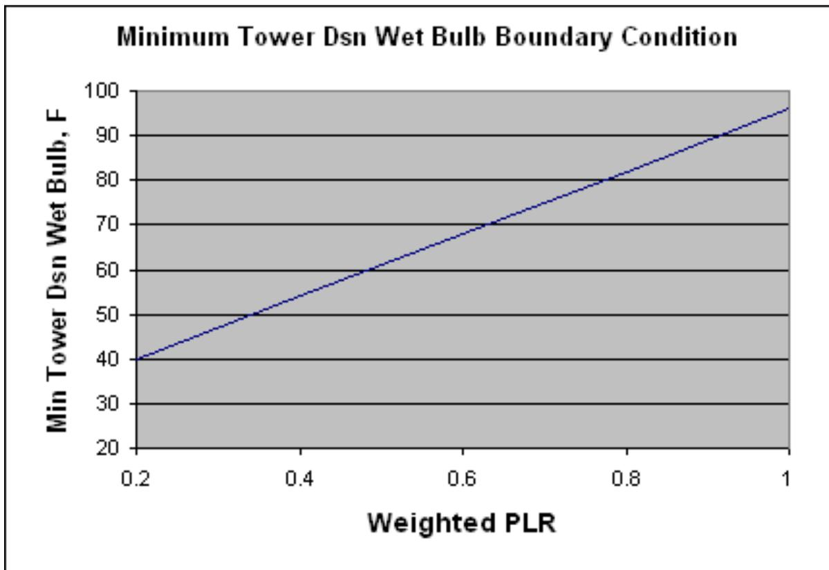
Figure 18.29: Minimum Tower Design Wet Bulb Boundary Condition
