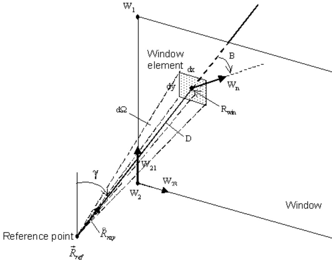
Figure 7.2: Geometry for calculation of direct component of daylight illuminance at a reference point. Vectors  $R_{ref}$ ,  $W_1$ ,  $W_2$ ,  $W_3$  and  $R_{win}$  are in the building coordinate system.
