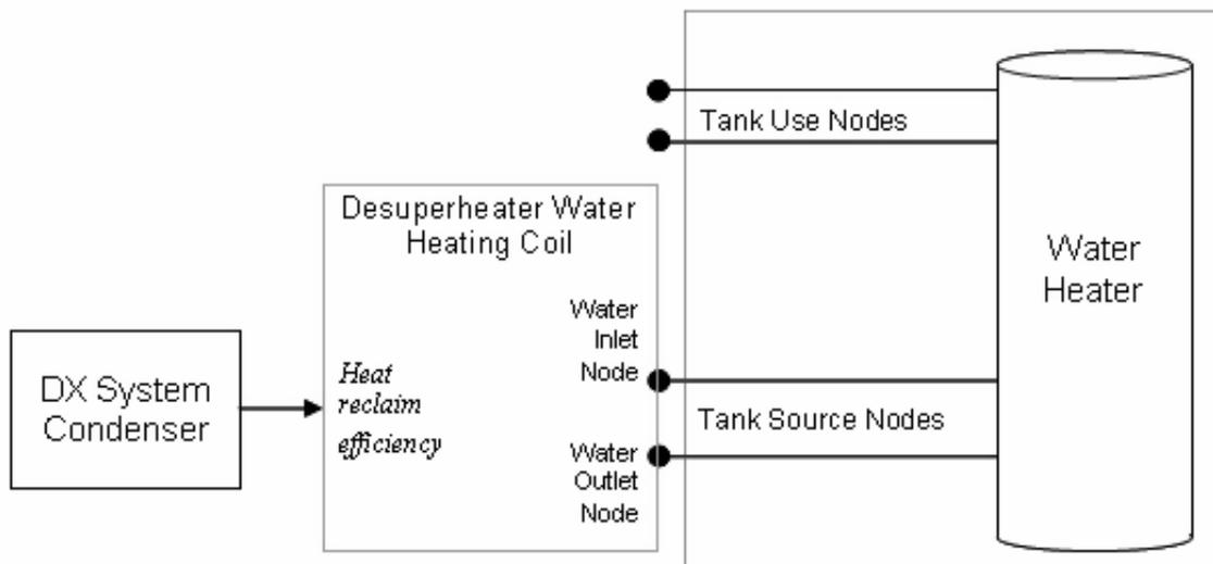
Figure 15.11: Schematic of Desuperheater Water Heating Coil
