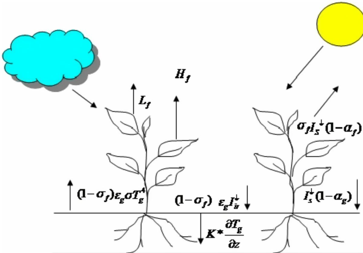
Figure 4.3: The Energy Balance for a Green Roof.
