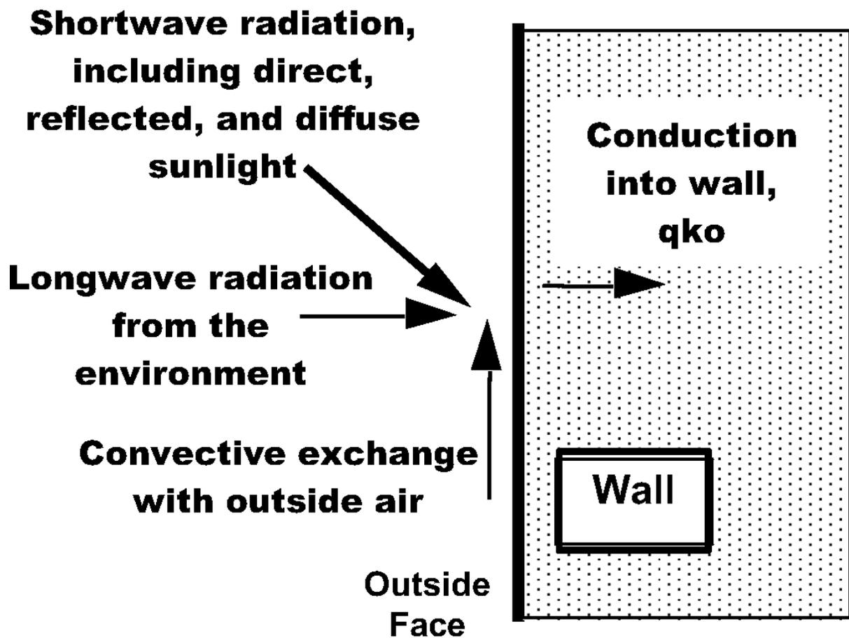
Figure 3.10: Outside Heat Balance Control Volume Diagram
