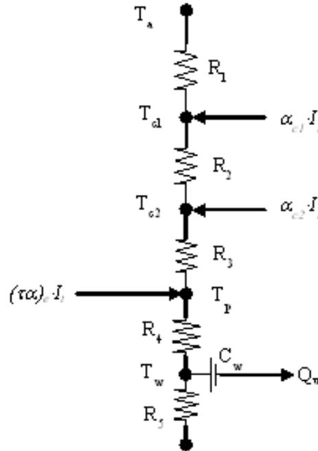
Figure 18.36: Thermal network diagram for ICS Solar Collector
