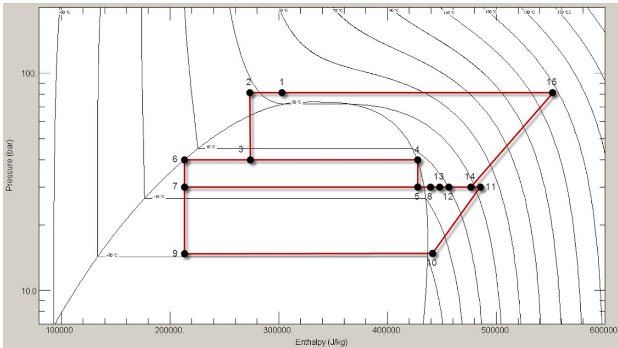
Figure 18.27: Pressure-Enthalpy (\*p-H\*) Diagram for the Transcritical CO<sub>2</sub> Booster Refrigeration Cycle.
