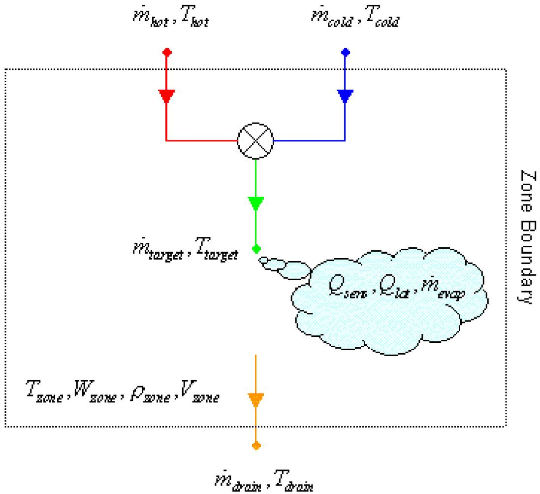
Figure 19.17: Zone Heat Gain from Water Use Equipment
