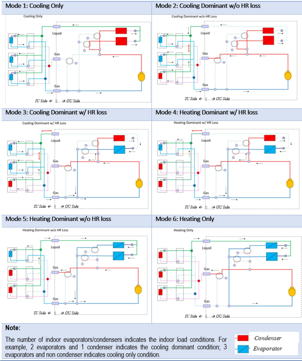
Figure 16.68: Piping diagrams for the six VRF-HR operational modes
