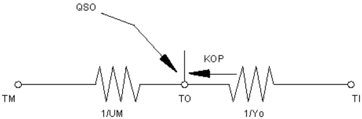
Figure 3.26: Thermal Network for Outside Moveable Insulation
