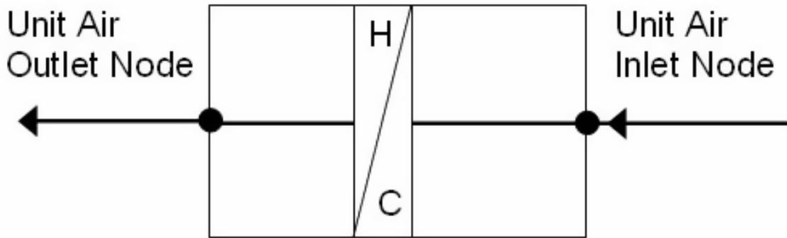
Figure 14.1: Schematic of AirTerminal:SingleDuct:ConstantVolume:Reheat Unit
