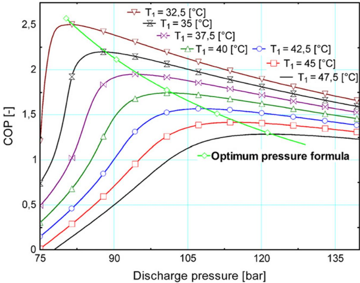
Figure 18.28: COP of CO<sub>2</sub> Transcritical Cycle vs. Discharge Pressure at Different Gas Cooler Exit Temperatures (Sawalha 2008).
