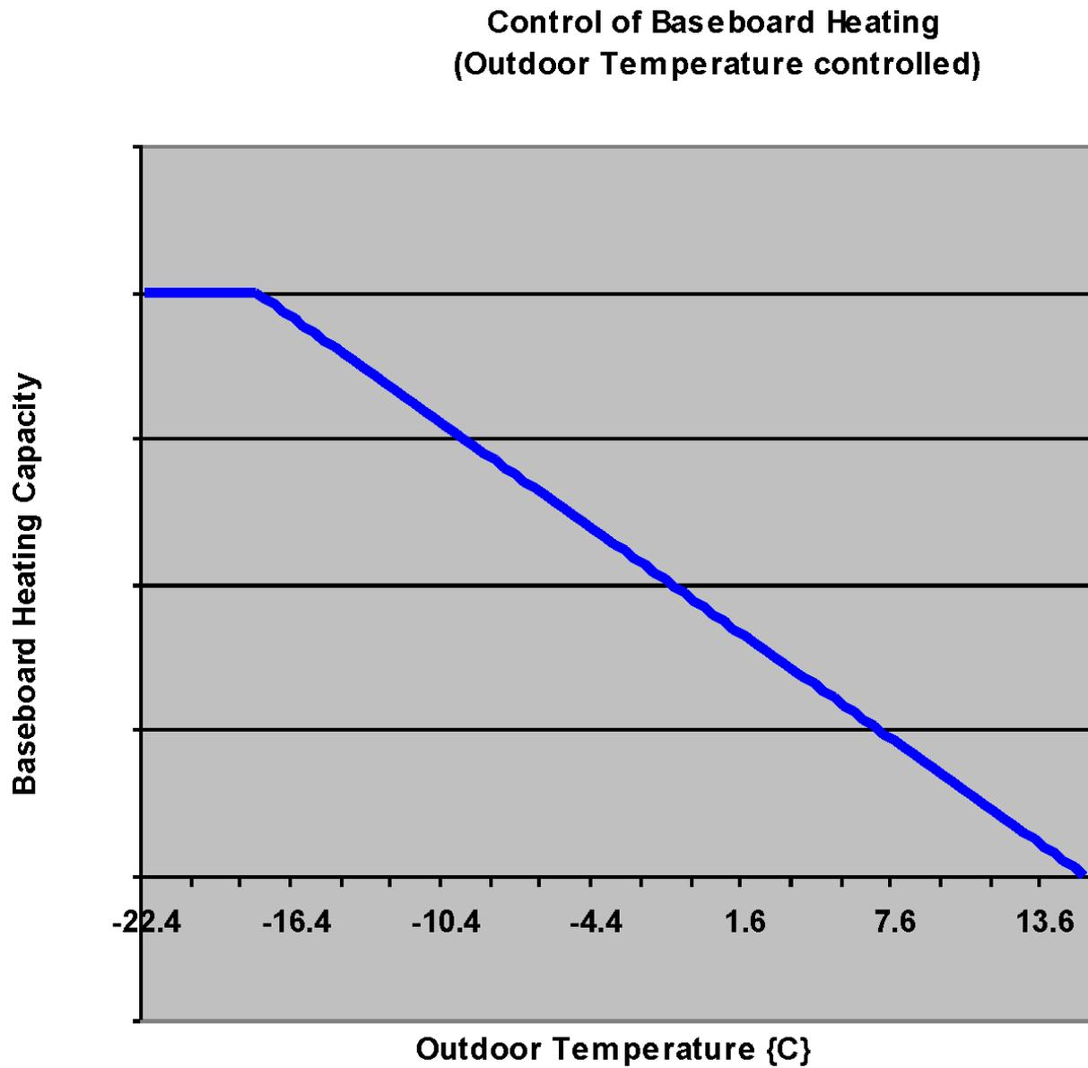
Figure 17.2: Control of Outdoor Temperature Controlled Baseboard Heat
