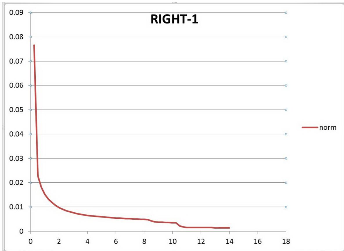
Figure 23.3: Load Component - Decay Curve of Exterior Wall
