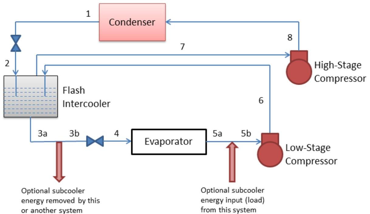
Figure 18.19: Two-Stage Compression System with a Flash Intercooler.
