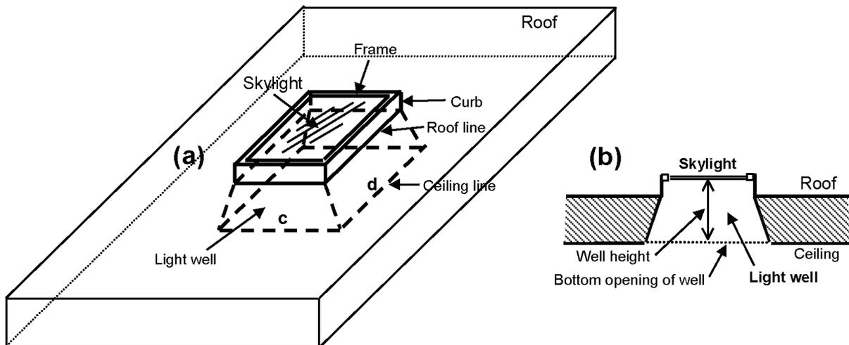
Figure 7.16: Skylight with light well: (a) perspective view, (b) vertical section. If the bottom of the light well is a rectangle of side lengths  $c$  and  $d$ , as shown in (a), then the perimeter of the bottom of the well =  $2(c+d)$  and the area =  $cd$  (see description of field names for the Light Well object).
