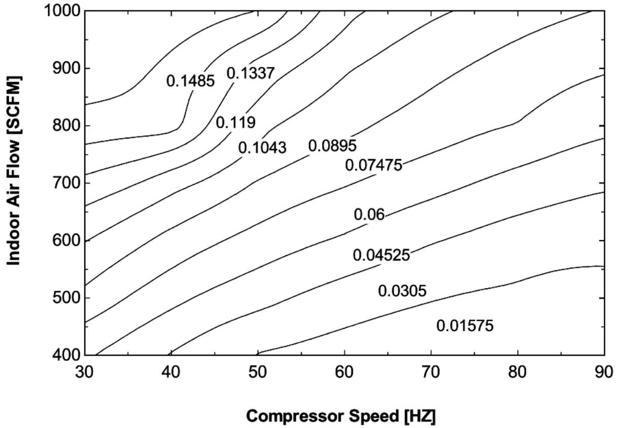
Figure 15.20: Bypass Factor (BF) Changing with Compressor Speed and Indoor SCFM
