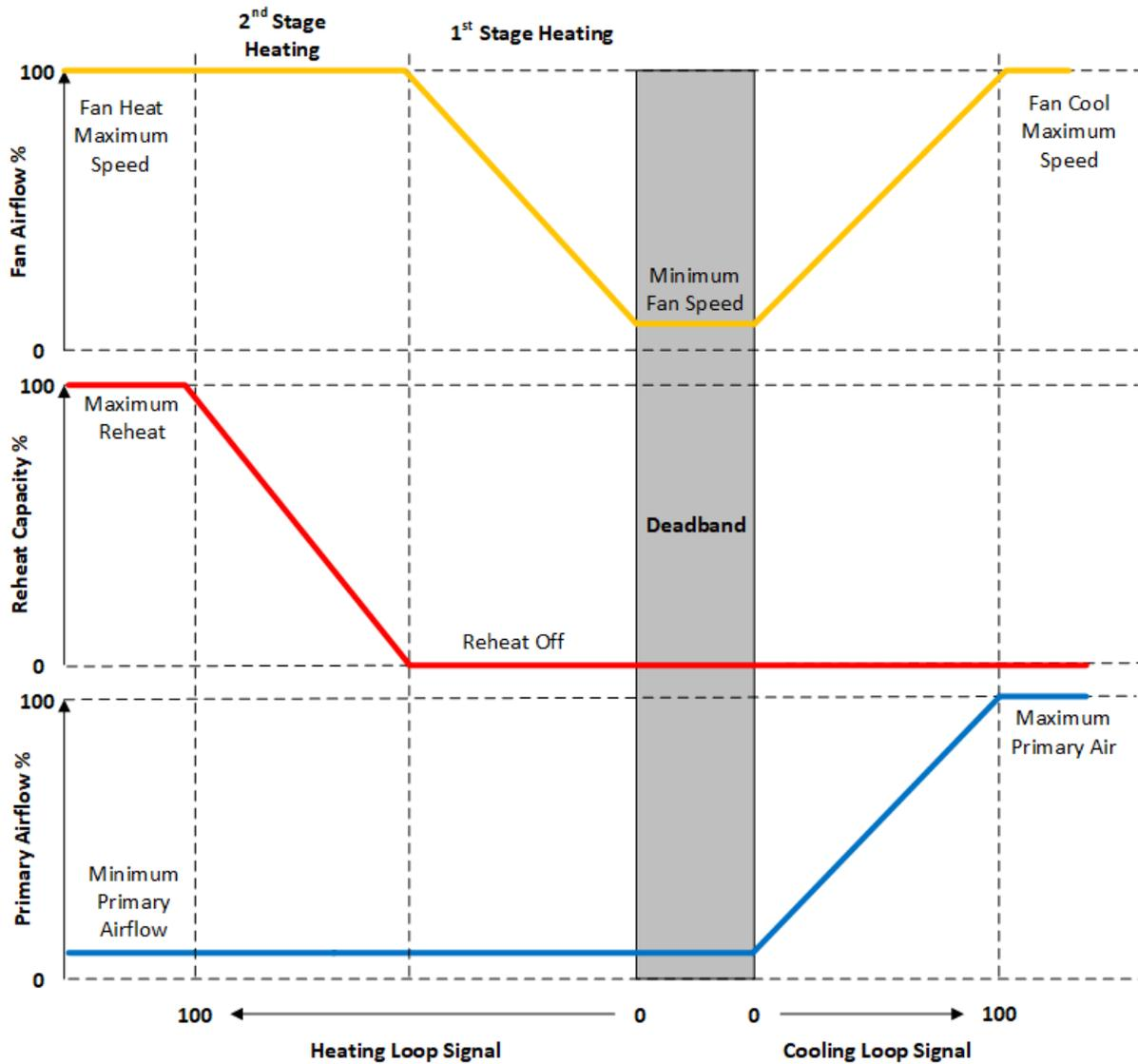
Figure 1.134: Variable Speed Fan with Staged Heat Control
