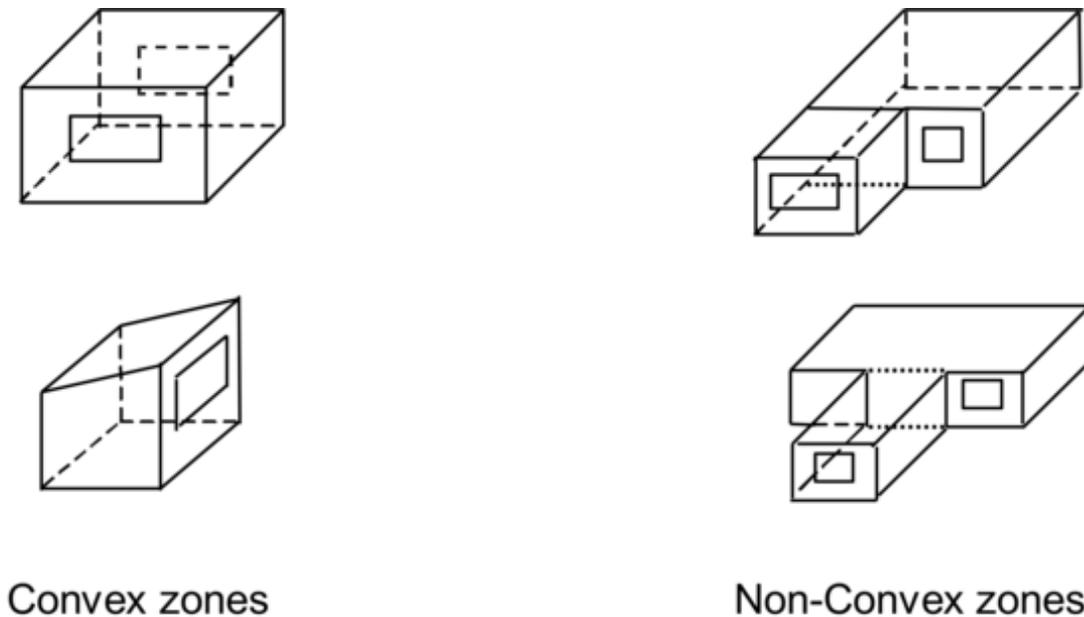
Figure 1.2: Illustration of Convex and Non-convex Zones
