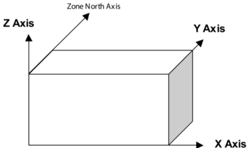
Figure 1.30: EnergyPlus Coordinate System
