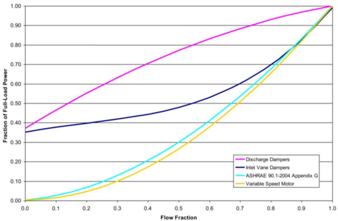
Figure 2.9: VAV Supply Fan Part-Load Power Coefficient Options
