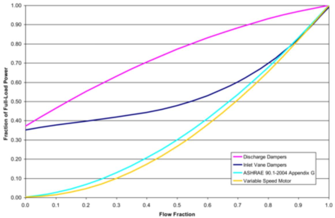
Figure 2.8: VAV Supply Fan Part-Load Power Coefficient Options
