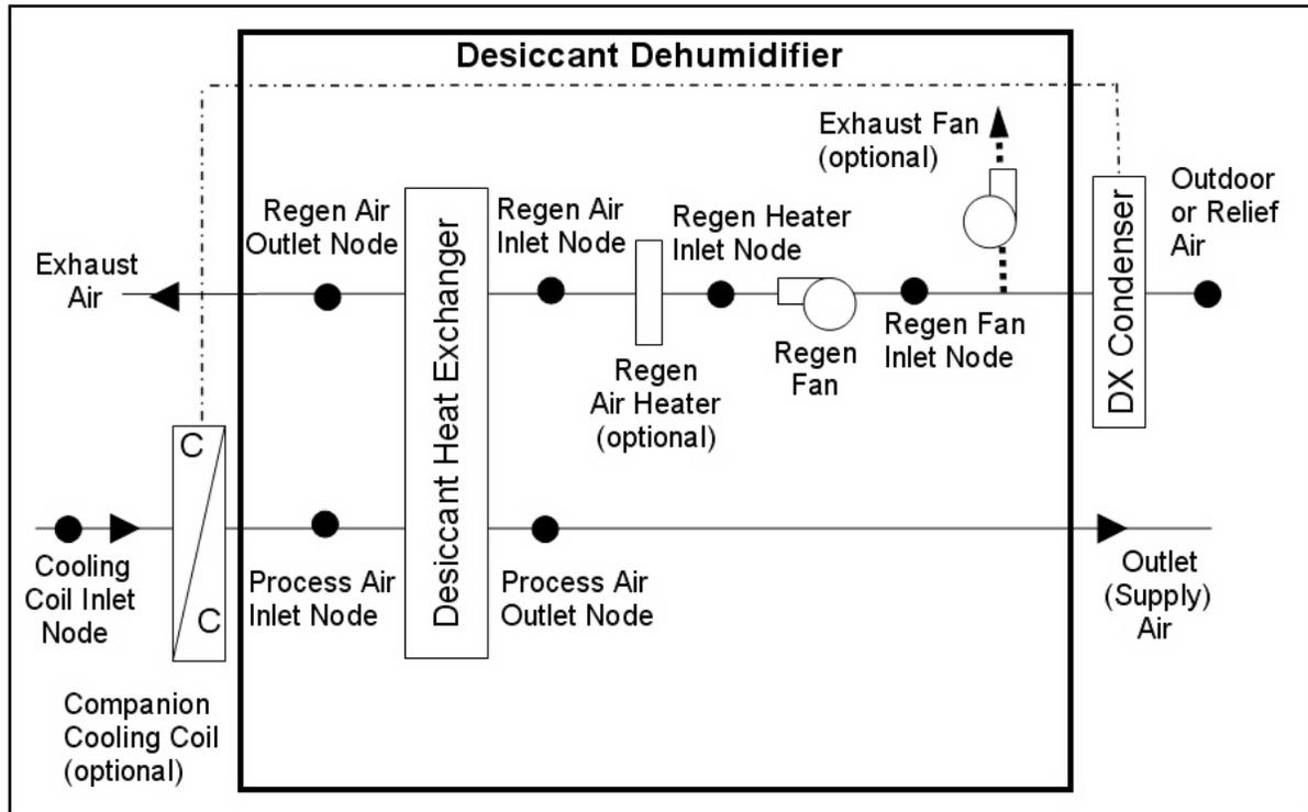
Figure 1.196: Schematic of Dehumidifier:Desiccant:System with Blow Through Regeneration Fan Placement
