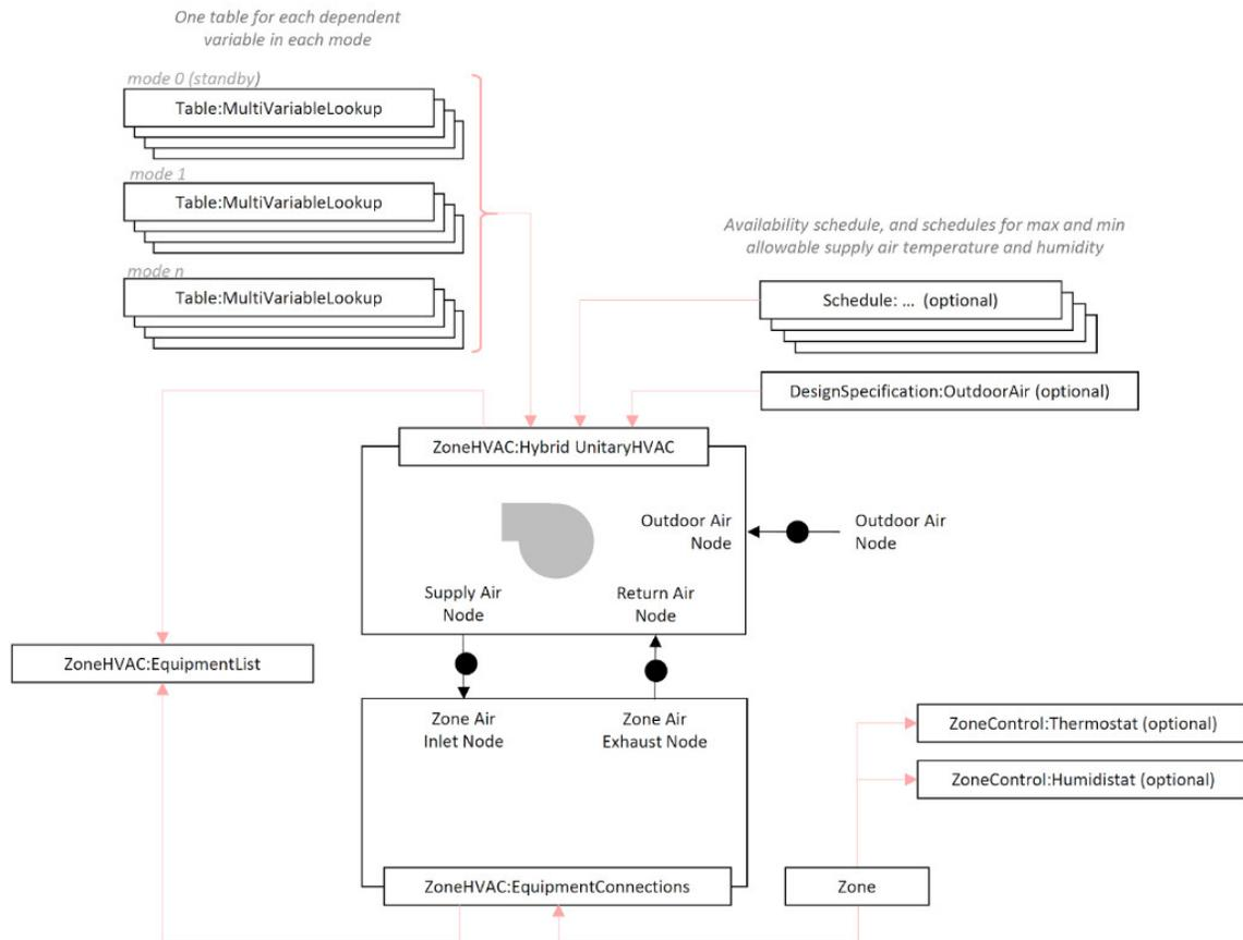
Figure 1.150: Schematic of object links for ZoneHVAC:HybridUnitaryHVAC
