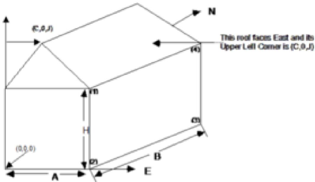
Figure 1.31: Illustration for Surface Vertices
