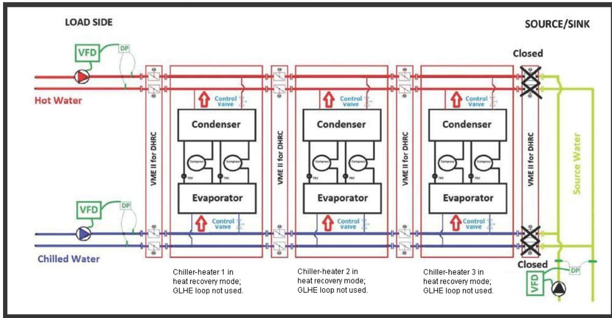
Figure 1.98: Diagram of a central heat pump system with three chiller-heaters in heat recovery mode (No heat is exchanged with the ground source loop)
