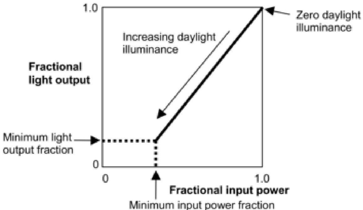
Figure 1.73: Illustration of continuous dimming relationship
