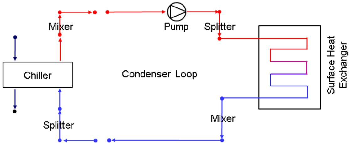
Figure 1.109: Example of Surface Ground Heat Exchanger as only heat exchanger on condenser loop
