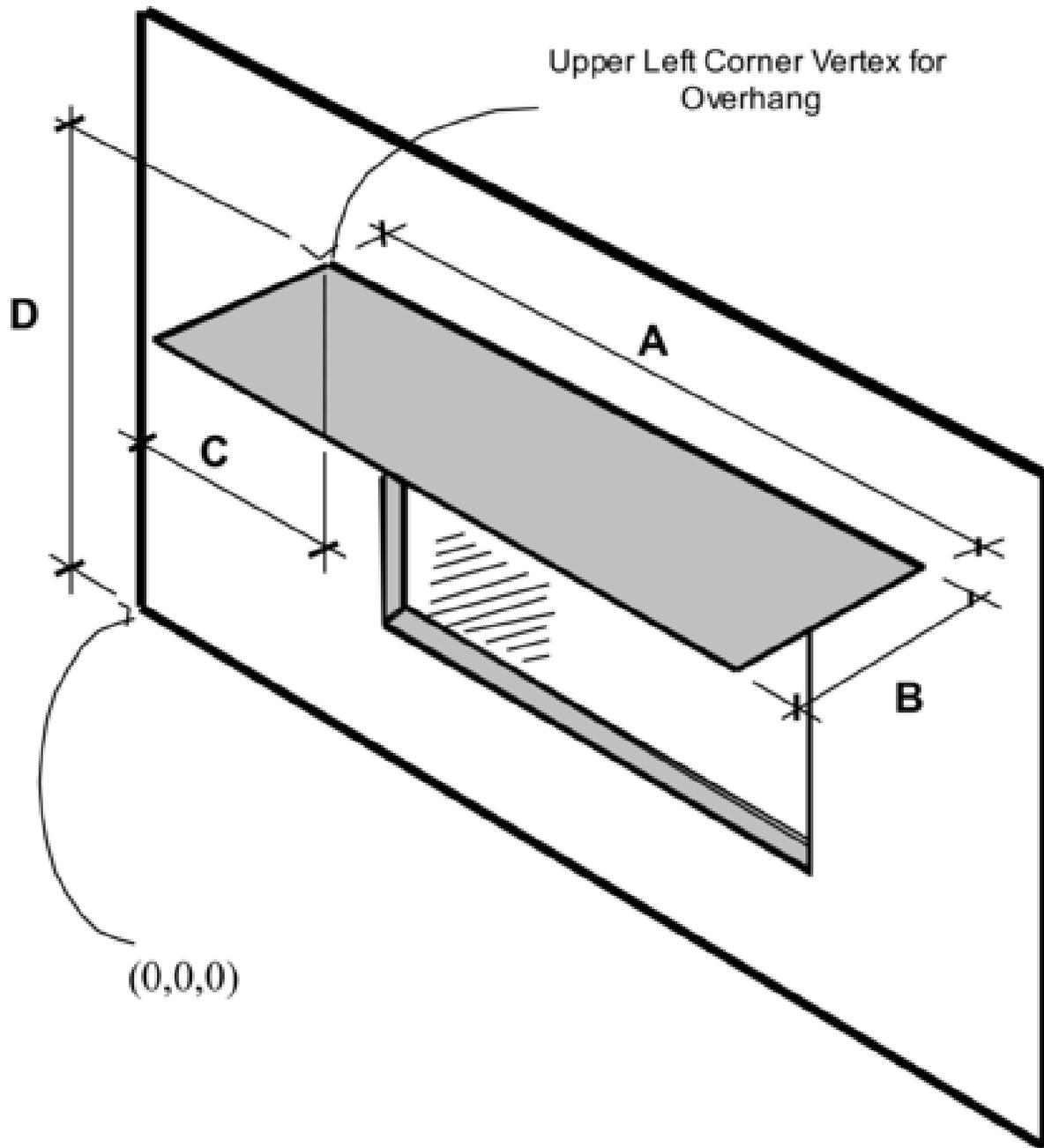
Figure 1.35: Illustration for Attached Shading Surface
