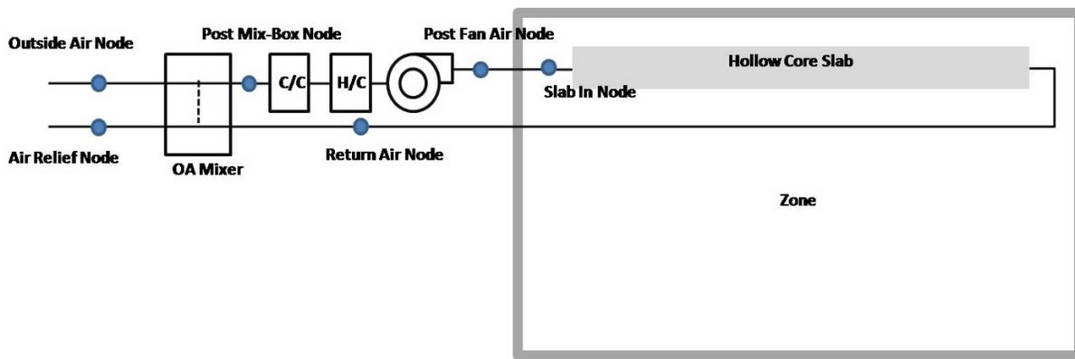
Figure 1.167: Ventilated Slab model - basic system
