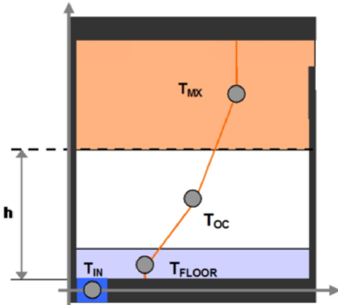
Figure 1.66: Schematic representation of the three temperature points and temperature gradients
