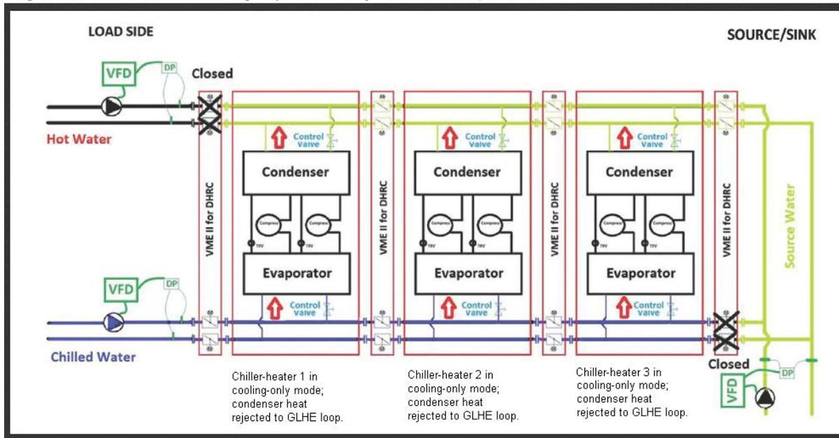
Figure 1.97: Diagram of a central heat pump system with three chiller-heaters in cooling-only mode (Condensers reject heat to the ground source loop)
