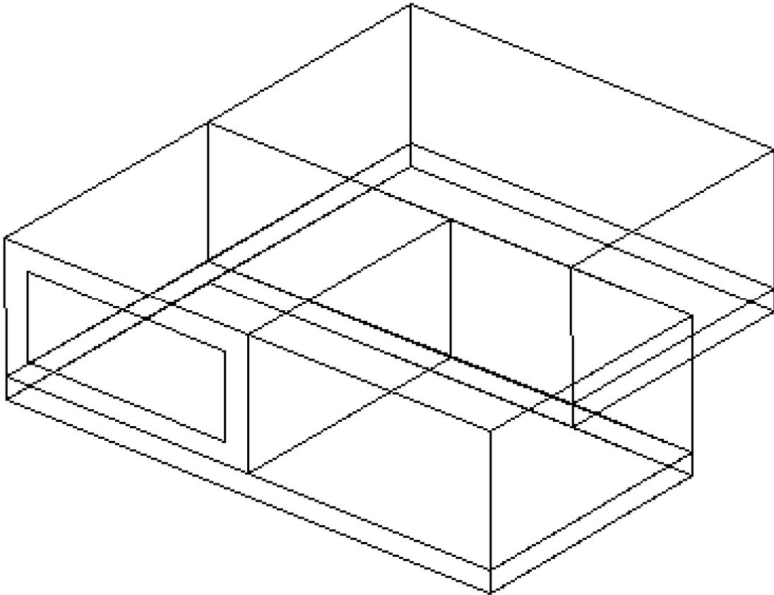
Figure 1.170: Illustration of AirLoopHVAC:SupplyPlenum
