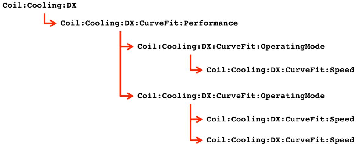
Figure 1.194: Hierarchy of references between cooling coil objects
