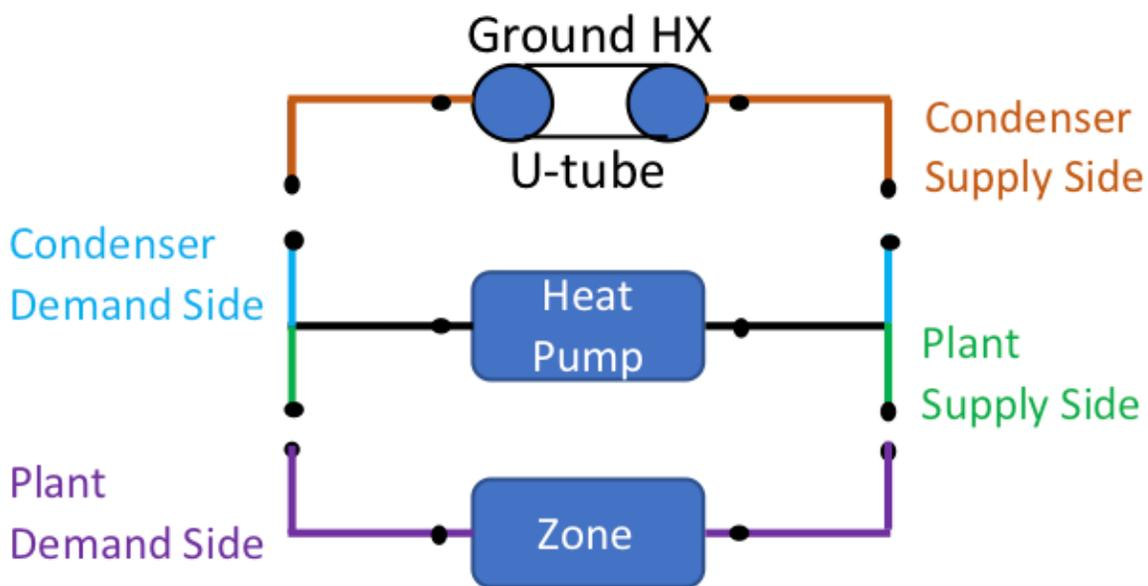
Figure 1.96: Schematic of EnergyPlus Ground Loop Heat Exchanger
