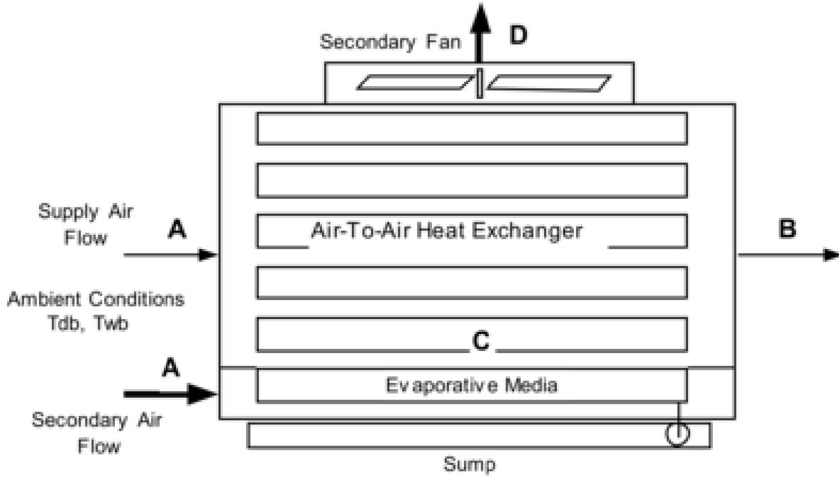
Figure 1.200: Evaporative Cooler – Indirect Dry Coil
