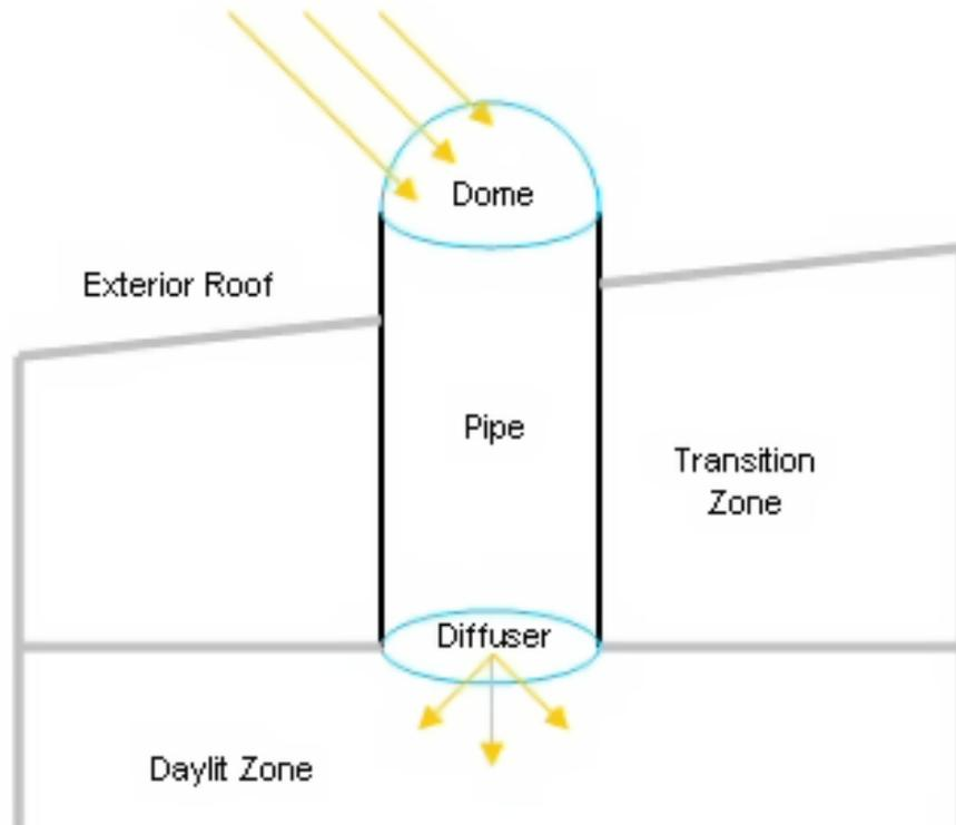
Figure 1.83: Tubular daylighting device diagram.
