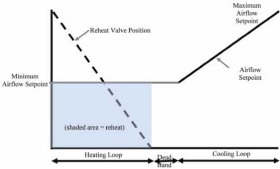
Figure 1.129: The Single Maximum Control Logic
