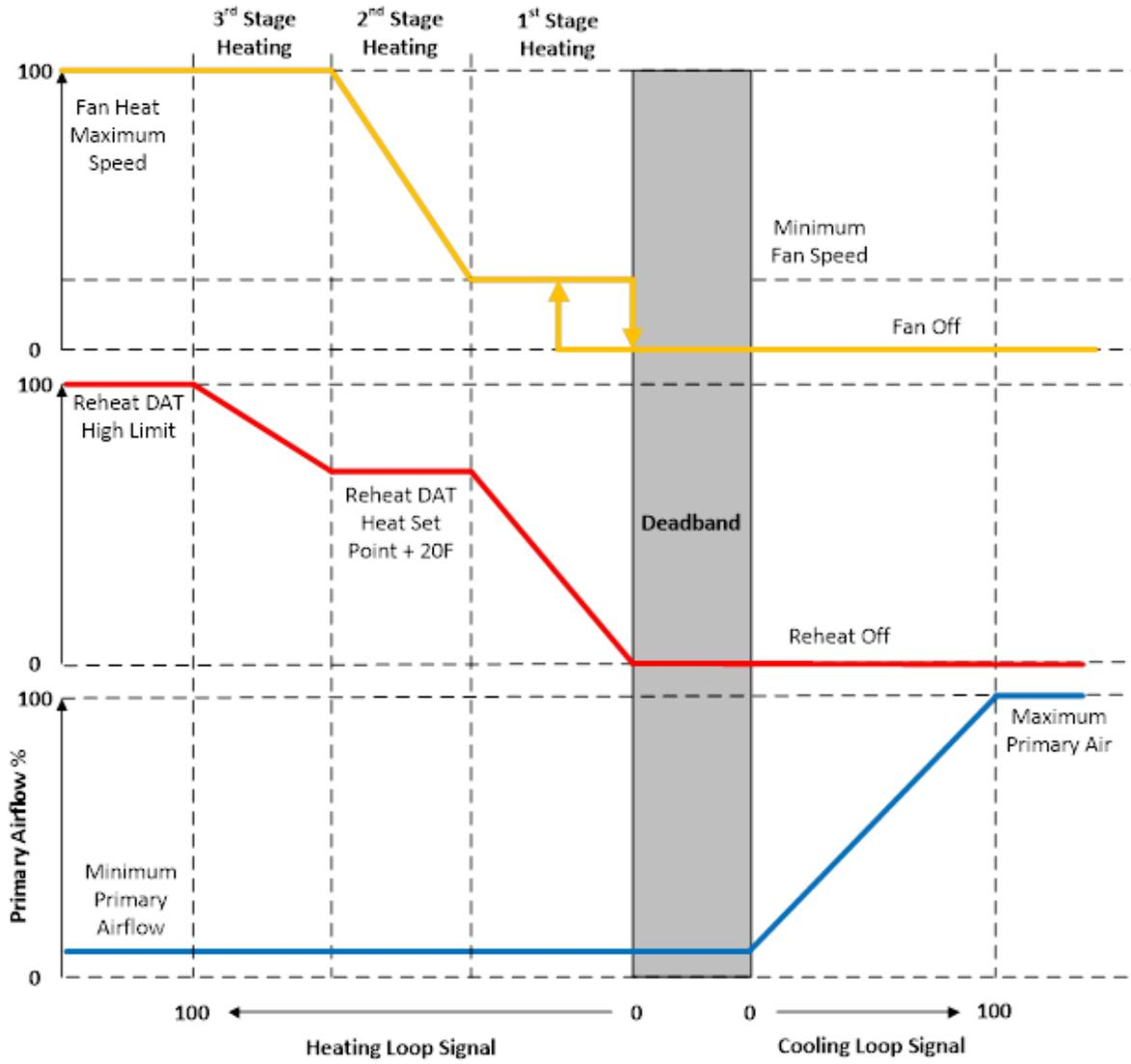
Figure 1.138: Variable Speed Fan with Modulated Heat Control
