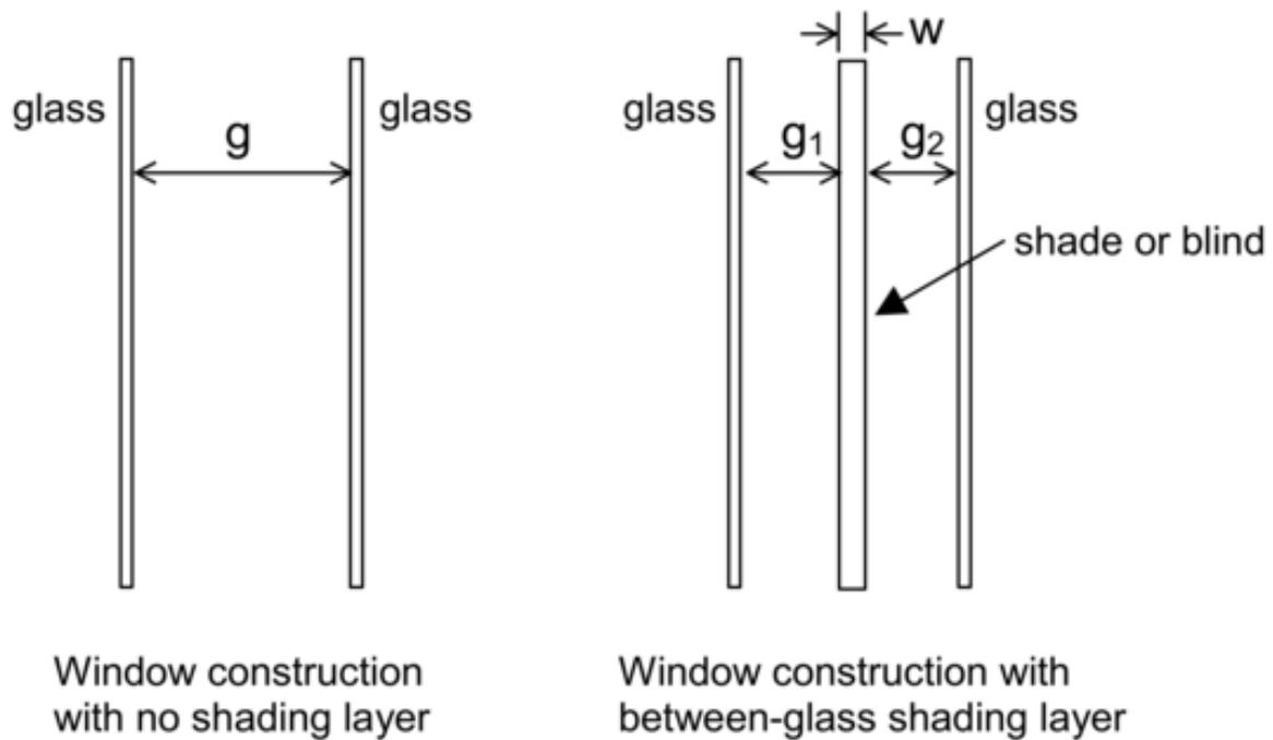
Figure 1.28: Window construction with and without a between-glass shading layer. Shown are gap widths  $g$ ,  $g_1$  and  $g_2$ , and shading layer width,  $w$ . An error will result if  $g_1 + g_2 + w$  is not equal to  $g$ , where  $w$  is zero for a blind and greater than zero for a shade.
