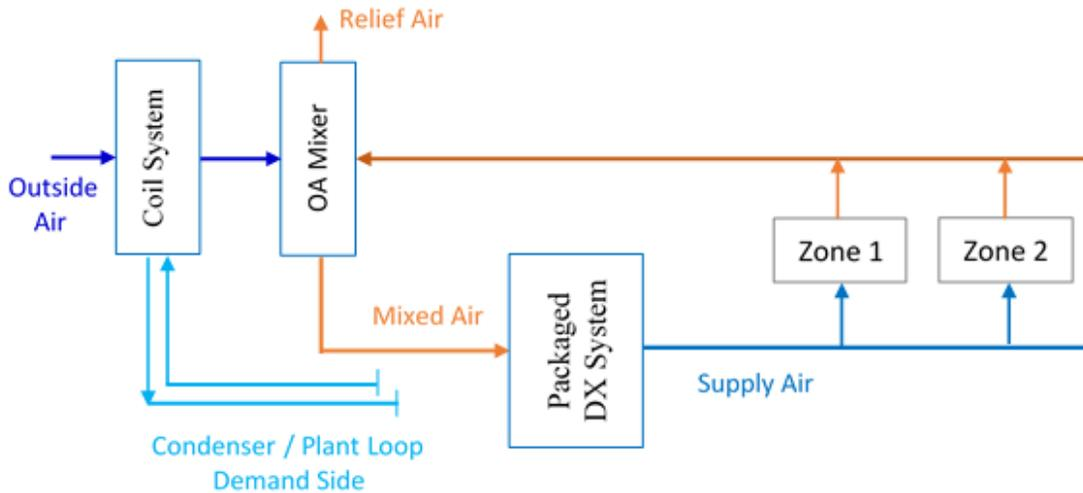
Figure 1.180: Water Side Economizer Coil System In Outdoor Air System
