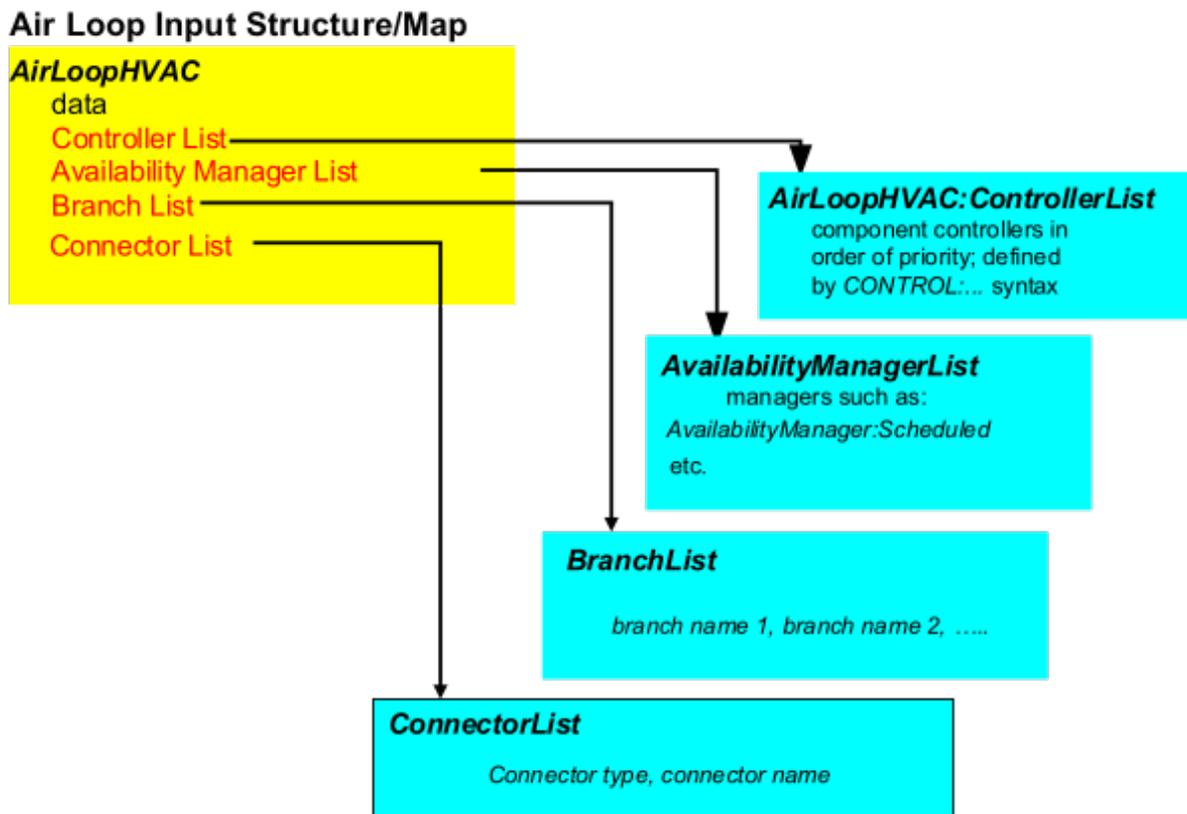
Figure 1.115: Air Loop Input Syntax Map
