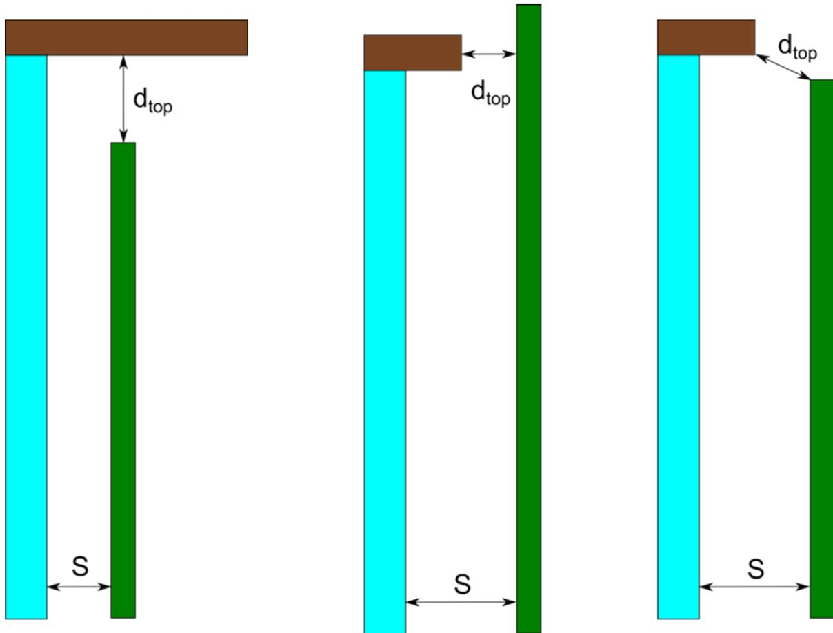
Figure 1.17: Three cases for the  $D_{top}$  calculation for an indoor/outdoor shade: Case a) A shading device between the frame; Case b) A shading device outside the frame, covering the frame; Case c) a shading device outside the frame, not covering the frame.
