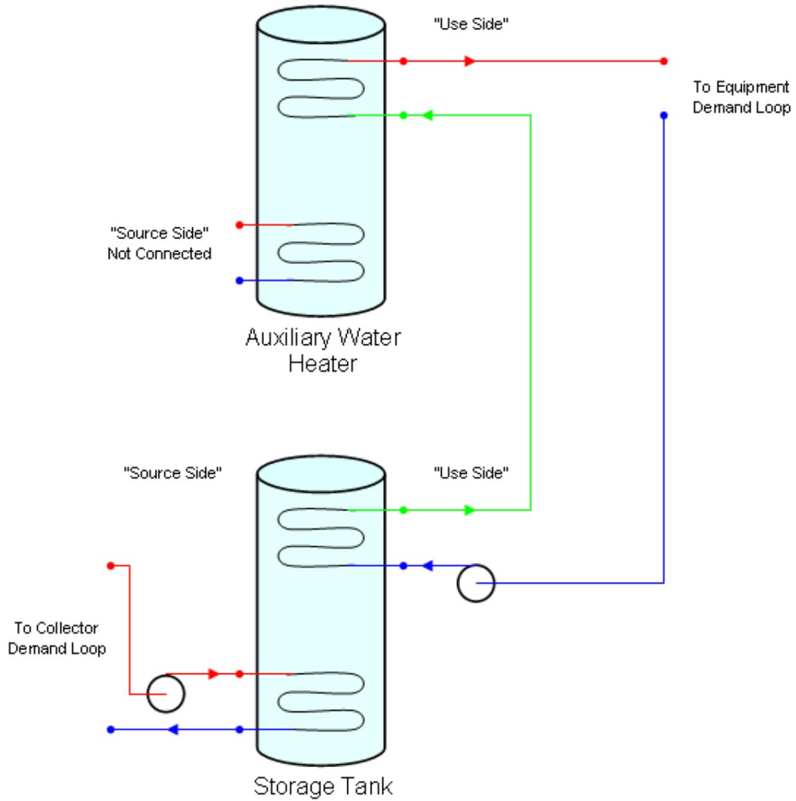
Figure 1.172: Two-Tank Solar Heating System Connection Diagram
