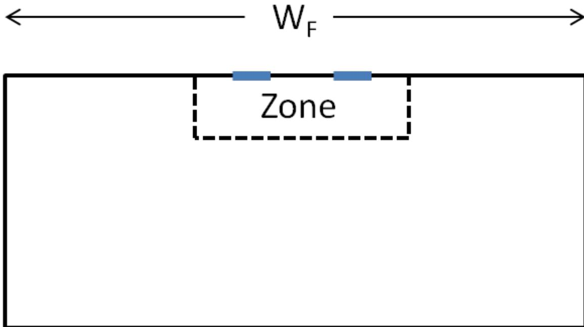
Figure 1.120: Footprint of a rectangular building showing  $W_F$ , the “Façade Width”, used by the Single Sided Wind Pressure Coefficient Algorithm.
