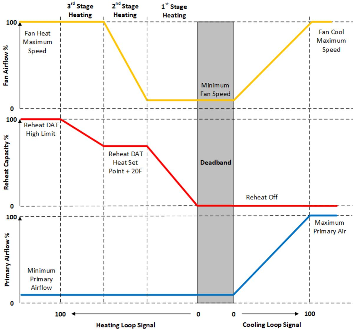
Figure 1.135: Variable Speed Fan with Modulated Heat Control
