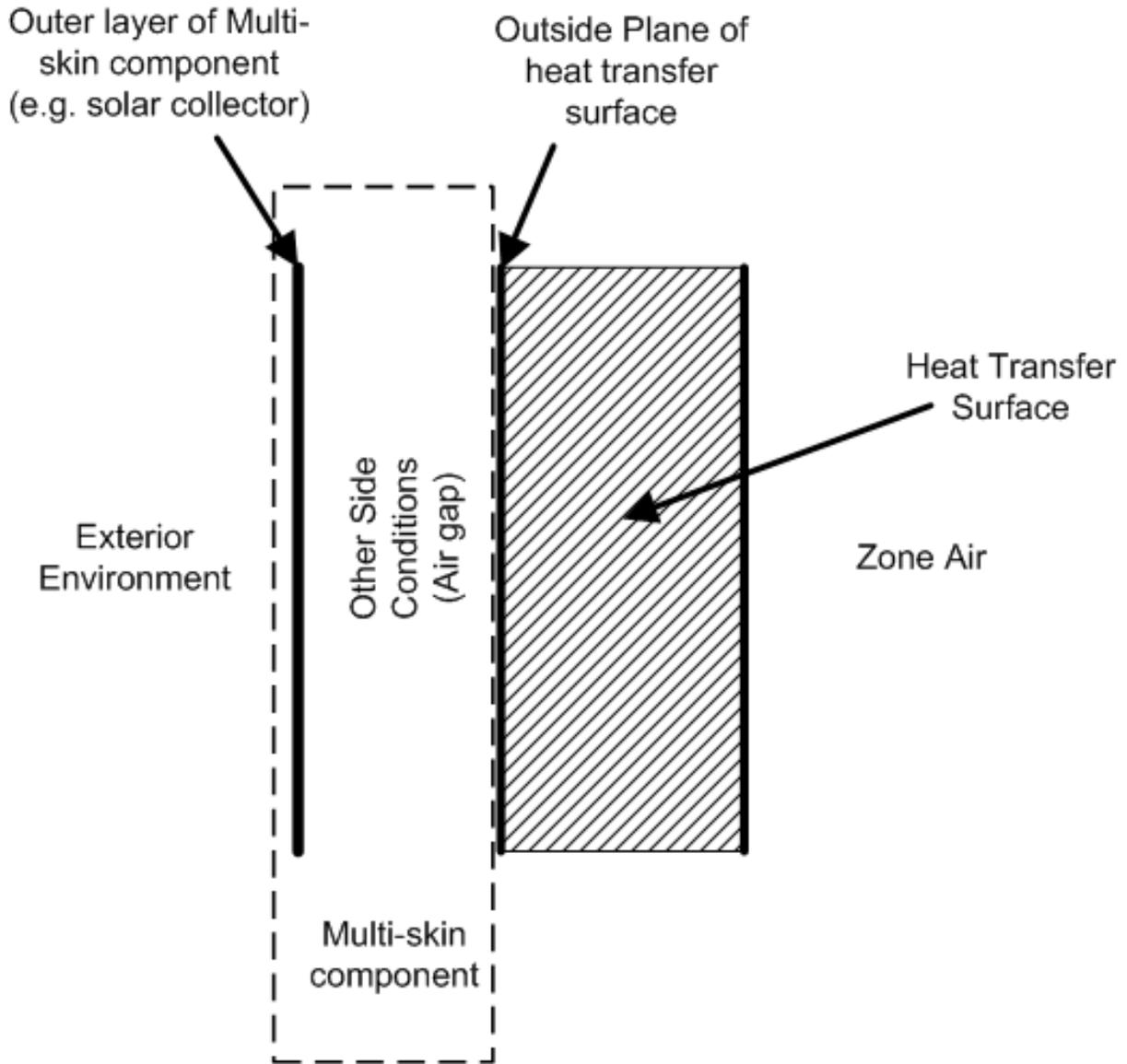
Figure 1.45: Illustration for Other Side Conditions Model
