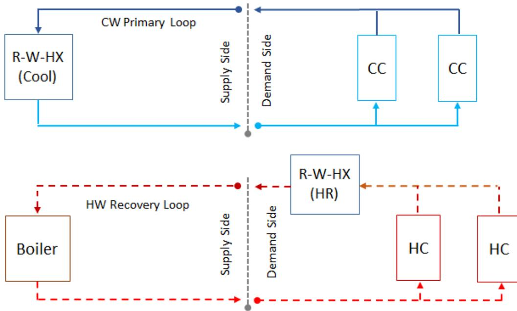
Figure 1.94: Schematic of Four-Pipe Air-to-Water Heat Pump with Heat Recovery
