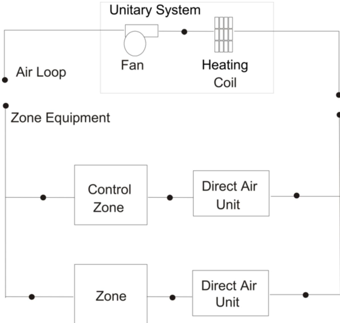
Figure 1.159: Schematic of Blow Through Heat-Only Unitary System
