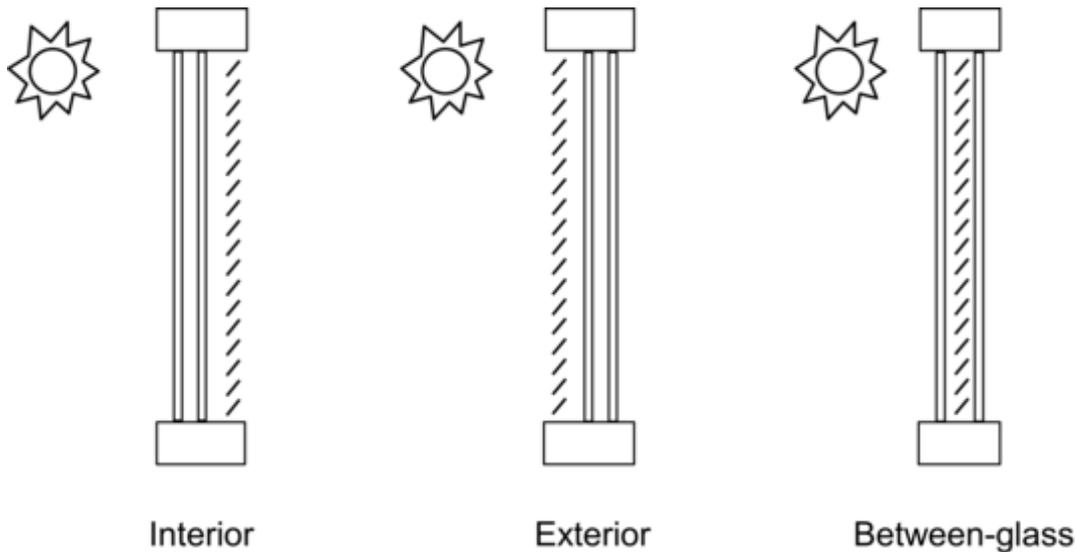
Figure 1.36: Allowed locations of a window shading device.
