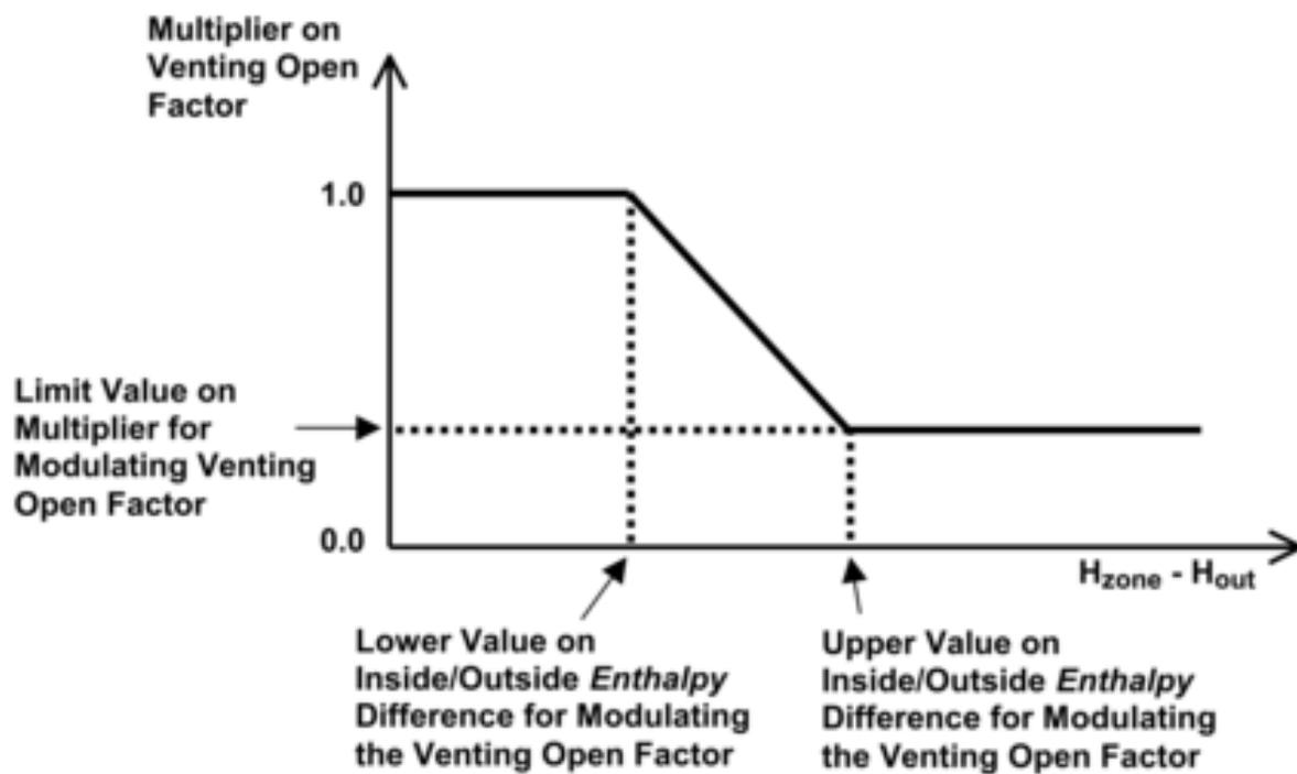
Figure 1.122: Modulation of venting area according to inside-outside enthalpy difference.
