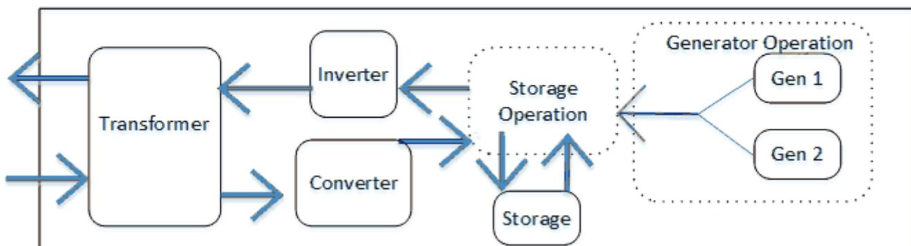
Figure 1.210: LoadCenterBusType
