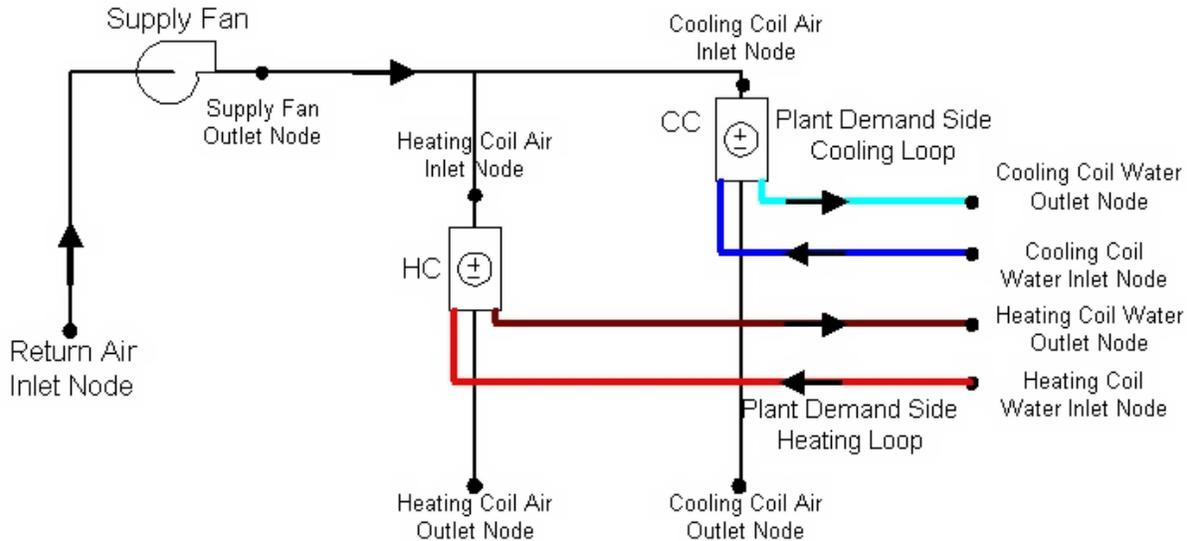
Figure 1.175: Example Air Loop Heating &amp; Cooling Coil
