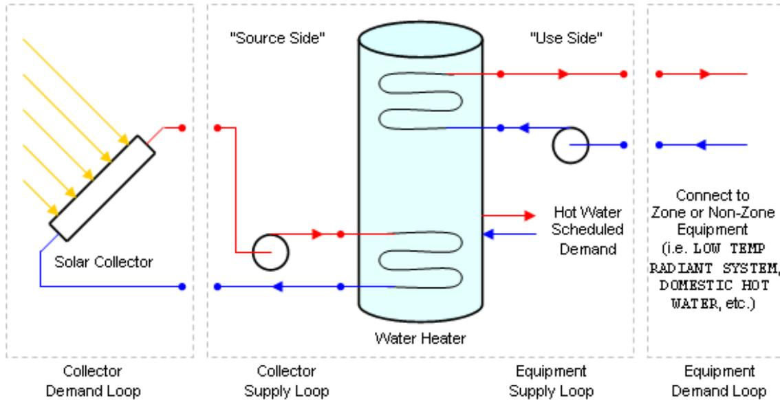
Figure 1.171: Solar Collector Plant Loop Connection Diagram
