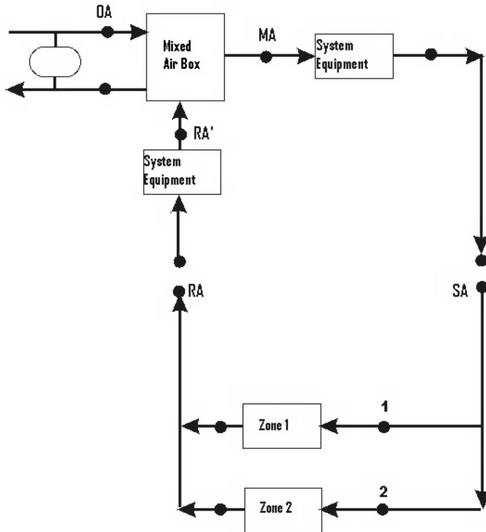
Figure 1.113: Example System for Ventilation Loads Report
