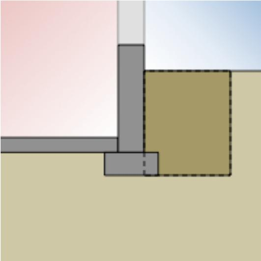
Figure 1.60: Custom block representing exterior backfill
