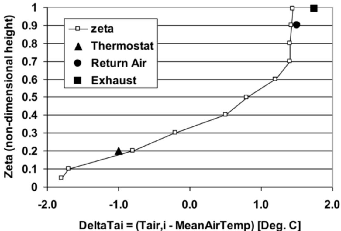
Figure 1.65: Example of a Vertical Air Temperature Pattern
