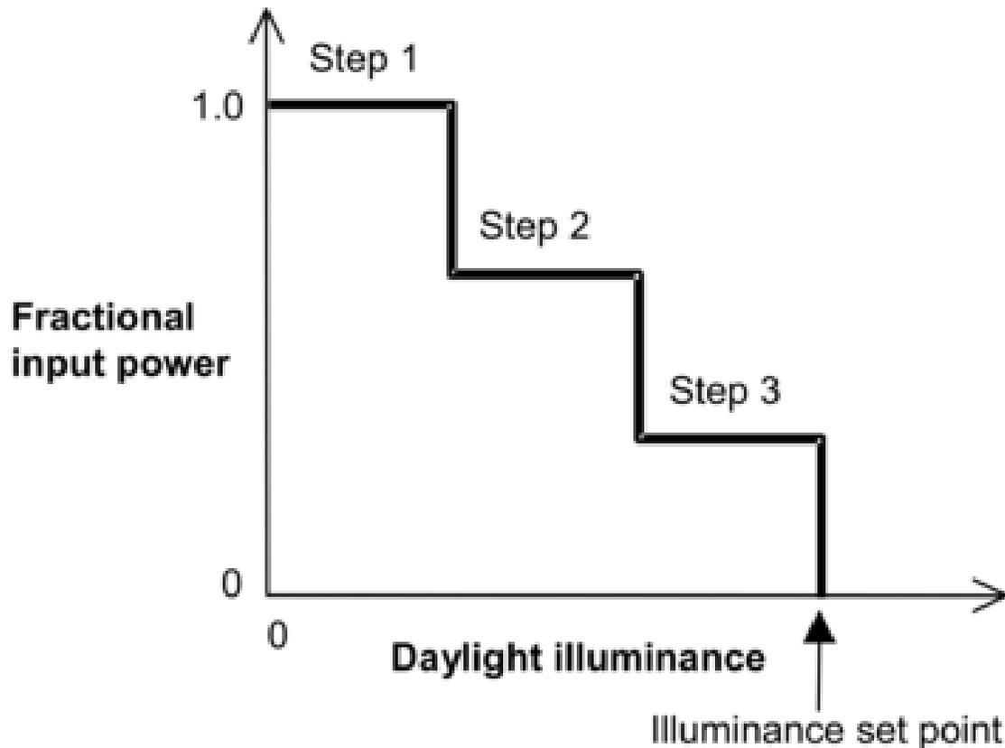
Figure 1.74: Stepped lighting control with Number of Steps = 3.
