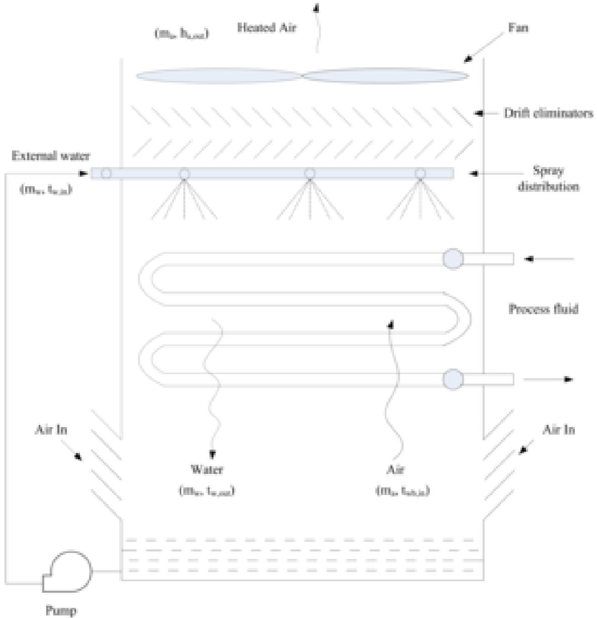
Figure 1.103: Schematic diagram for evaporative fluid cooler
