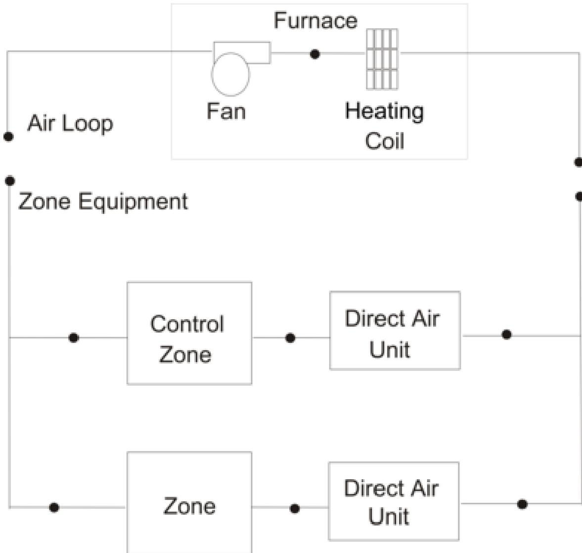
Figure 1.158: Schematic of Blow Through Furnace Model
