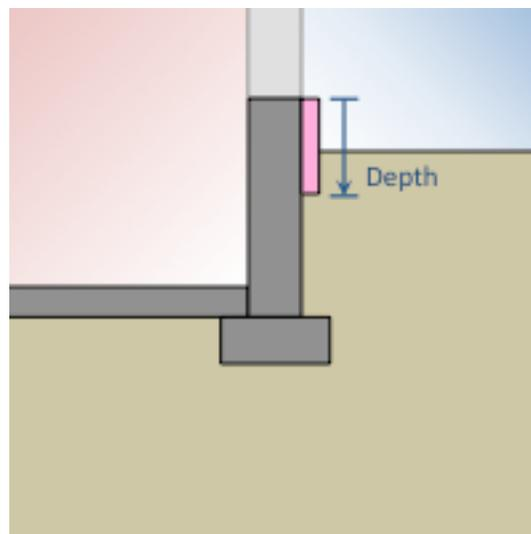
Figure 1.55: Placement of exterior vertical insulation
