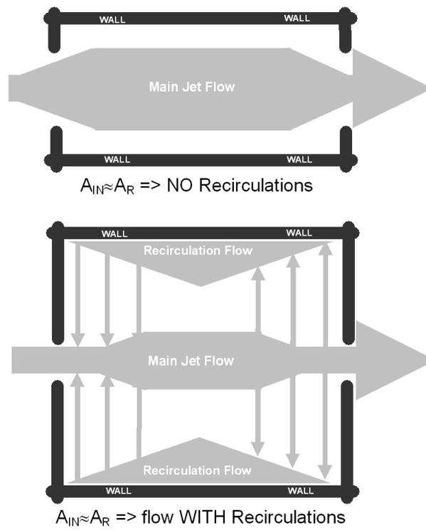
Figure 1.68: Schematic top view — possible airflow patterns in cross-ventilation.
