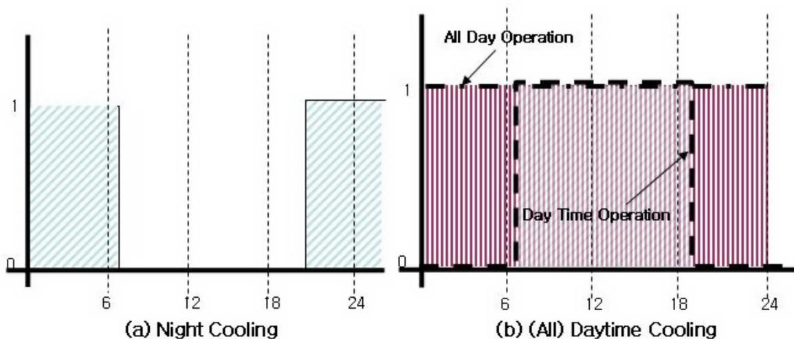
Figure 1.168: Example operating schedule for Ventilated Slab
