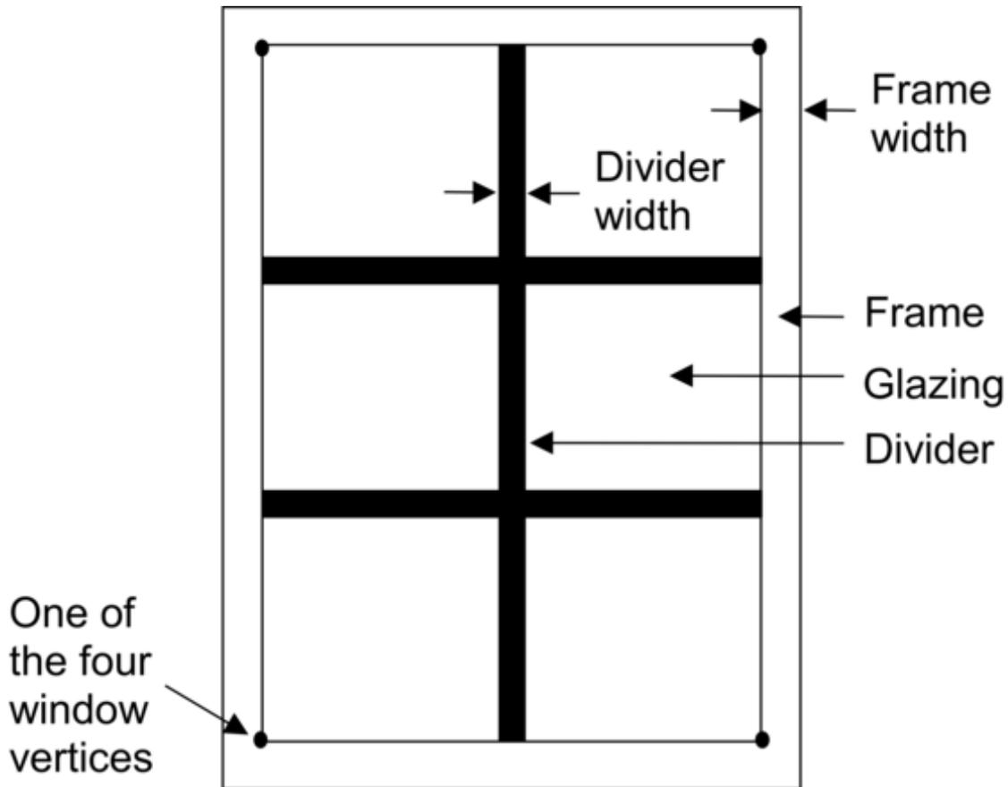
Figure 1.37: A window with a frame and divider.
