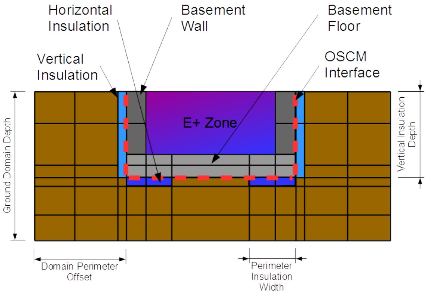
Figure 1.9: Basement Configuration
