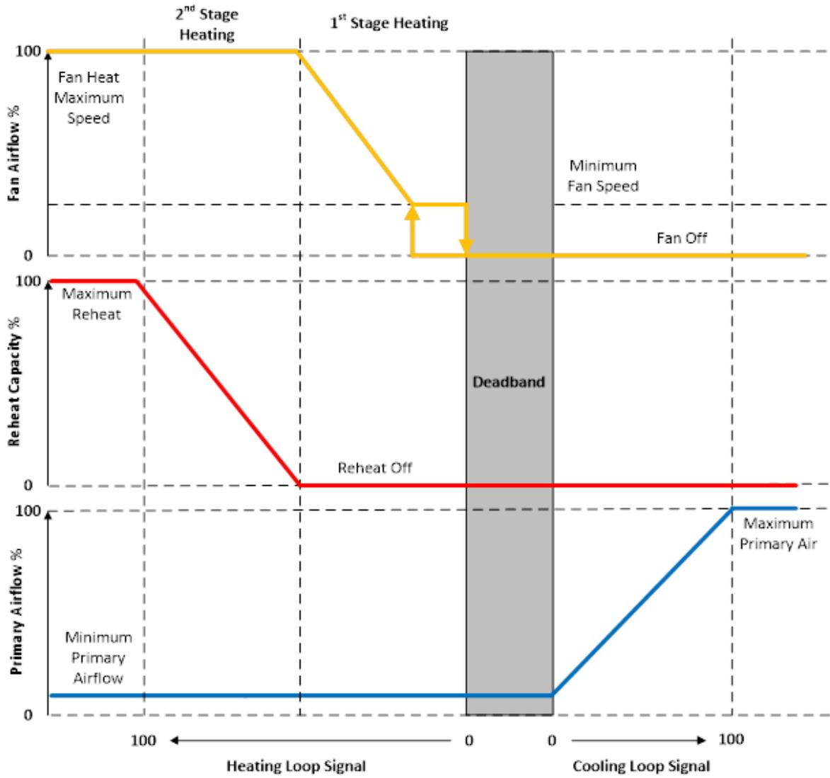
Figure 1.137: Variable Speed Fan with Staged Heat Control
