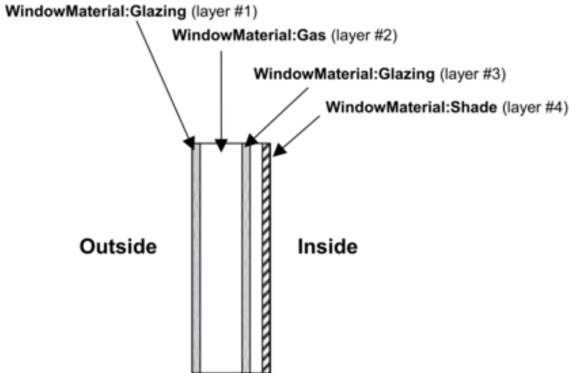
Figure 1.27: Illustration for material ordering in windows.
