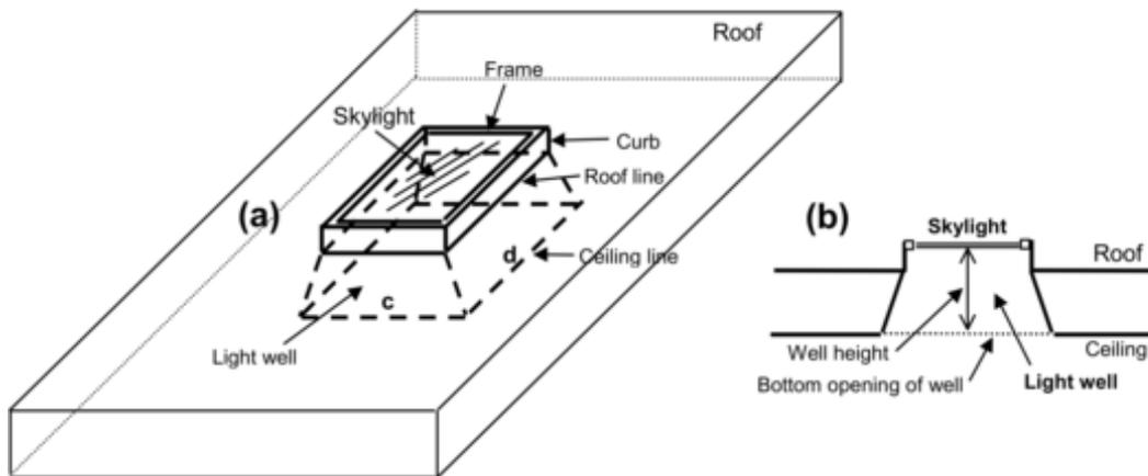
Figure 1.87: Skylight with light well: (a) perspective view, (b) vertical section. If the bottom of the light well is a rectangle of side lengths  $c$  and  $d$ , as shown in (a), then the perimeter of the bottom of the well =  $2(c+d)$  and the area =  $cd$  (see description of field names for the Light Well object).
