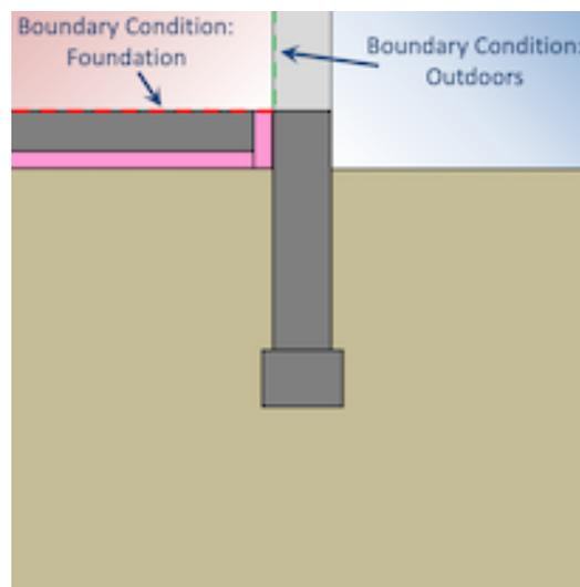
Figure 1.49: Two-dimensional interpretation of foundation surface data
