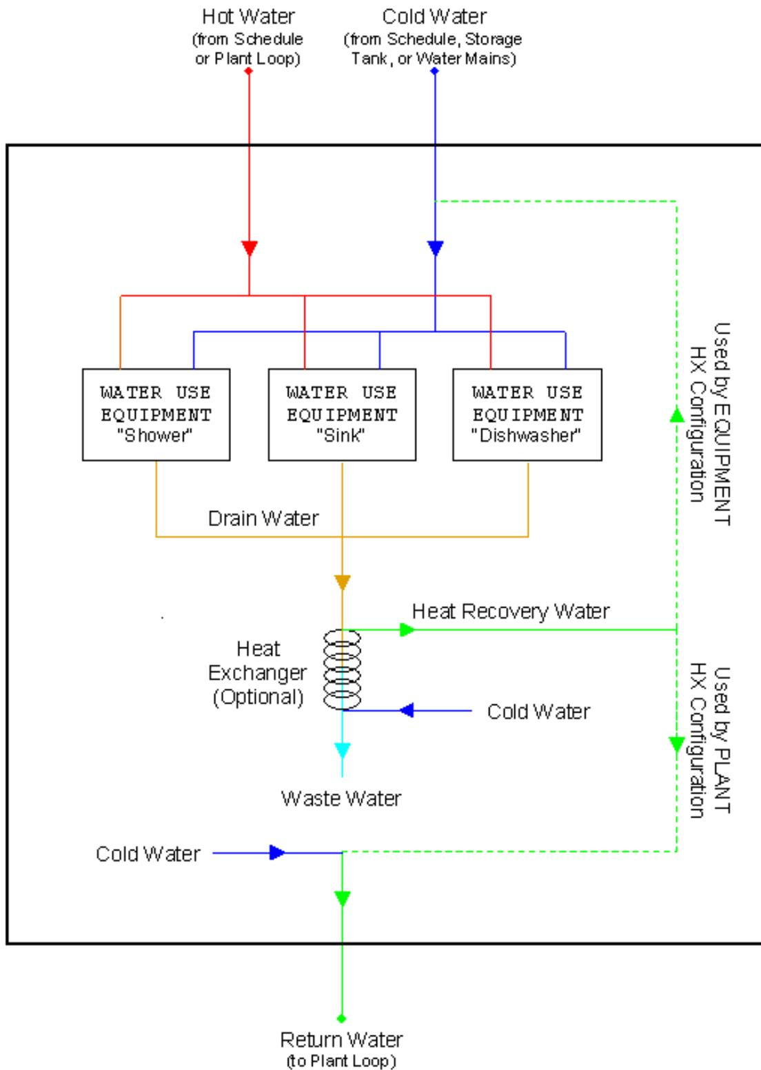
Figure 1.213: Diagram of internal connections for WaterUse:Connections
