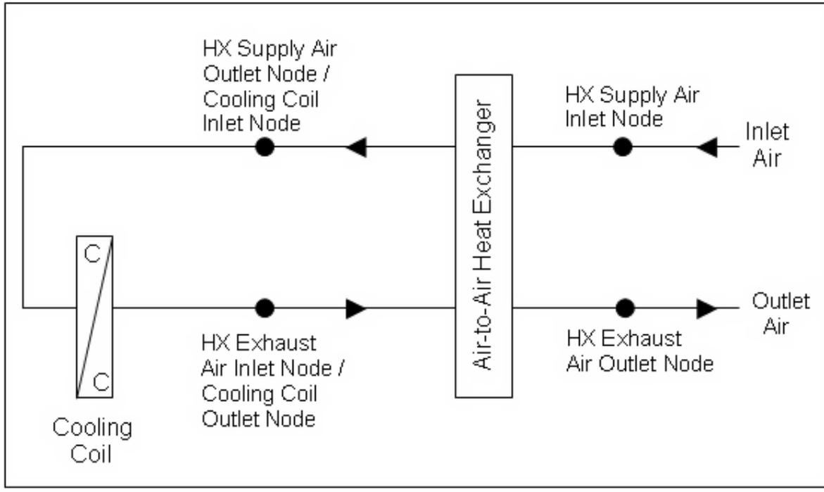
Figure 1.185: Schematic of the CoilSystem:Cooling:DX:HeatExchangerAssisted compound object
