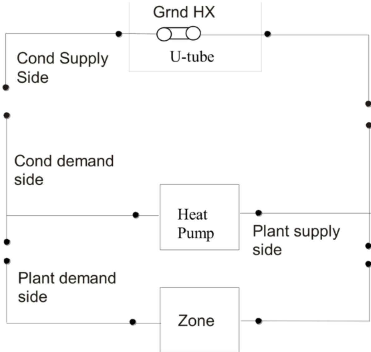
Figure 1.104: Schematic of EnergyPlus Ground Loop Heat Exchanger
