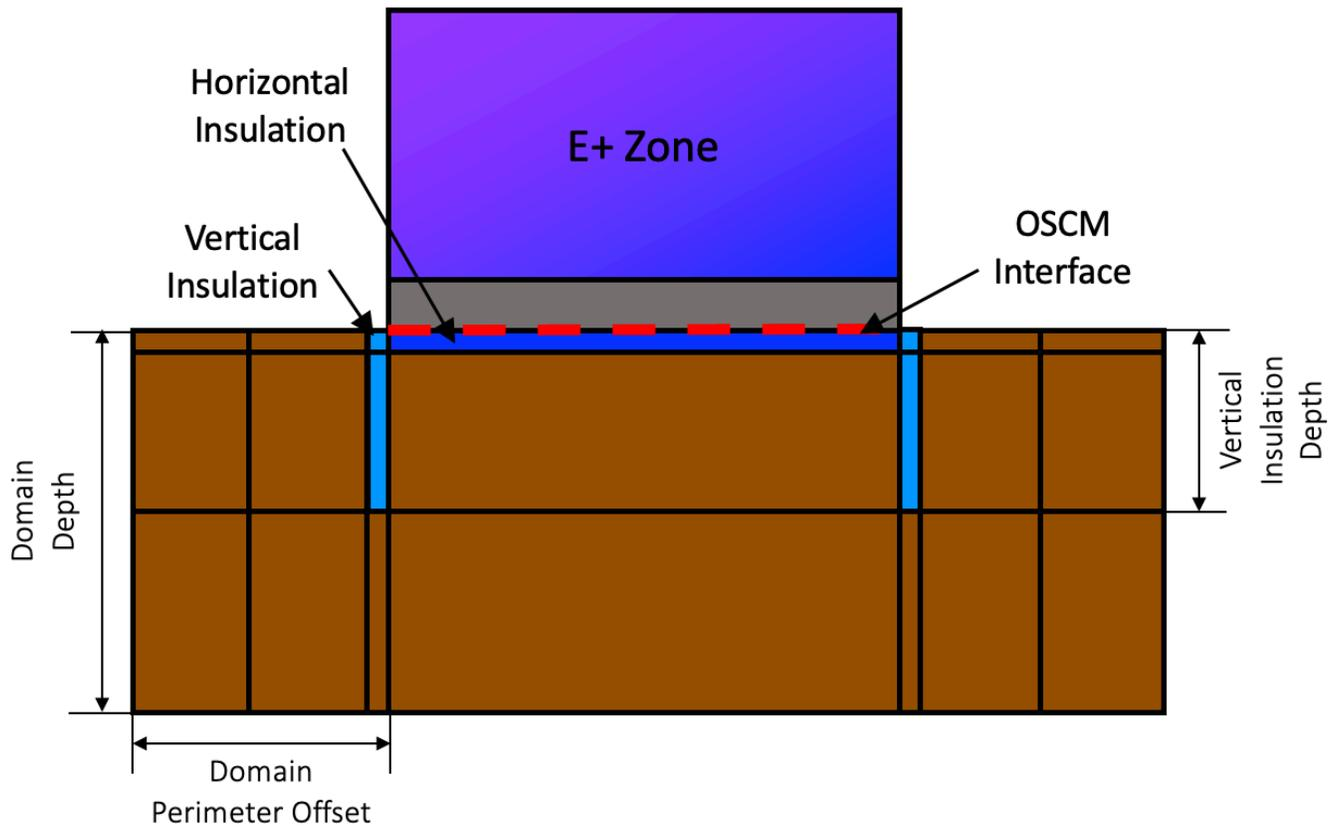
Figure 1.8: On-grade configuration
