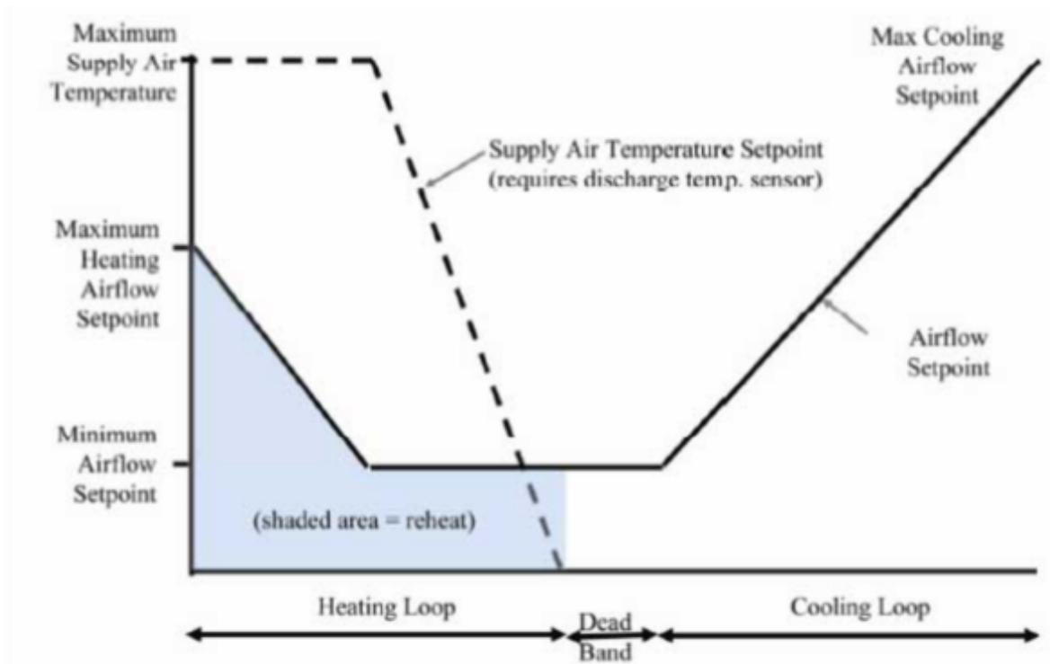
Figure 1.130: The Dual Maximum Control Logic
