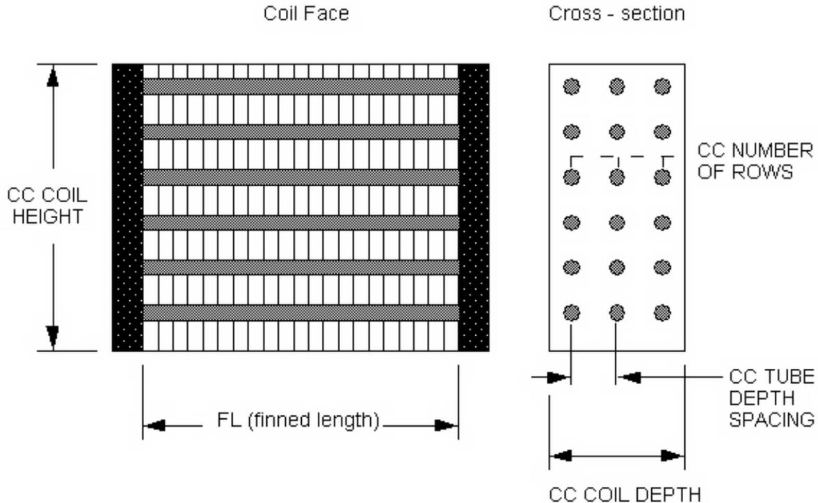
Figure 1.176: Geometry of a Cooling Coil (CC)
