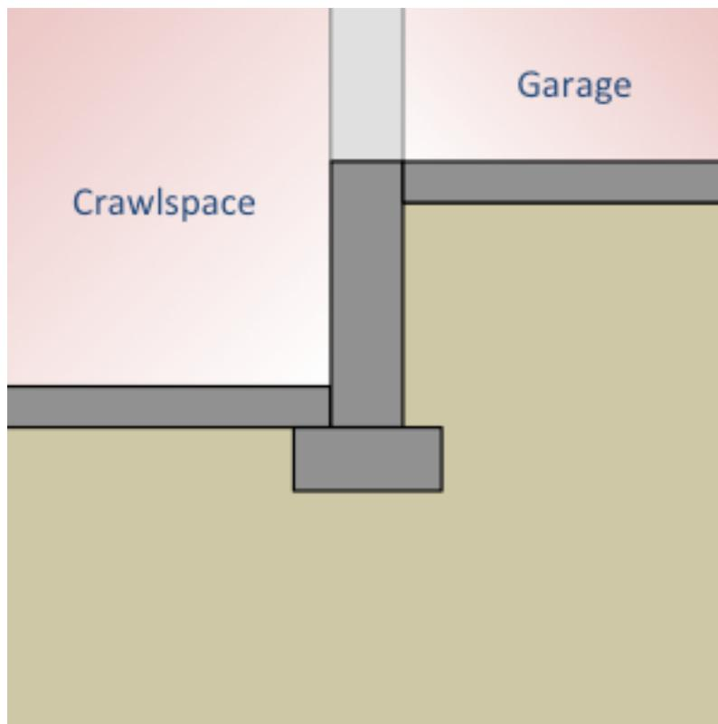
Figure 1.63: Interior foundation wall
