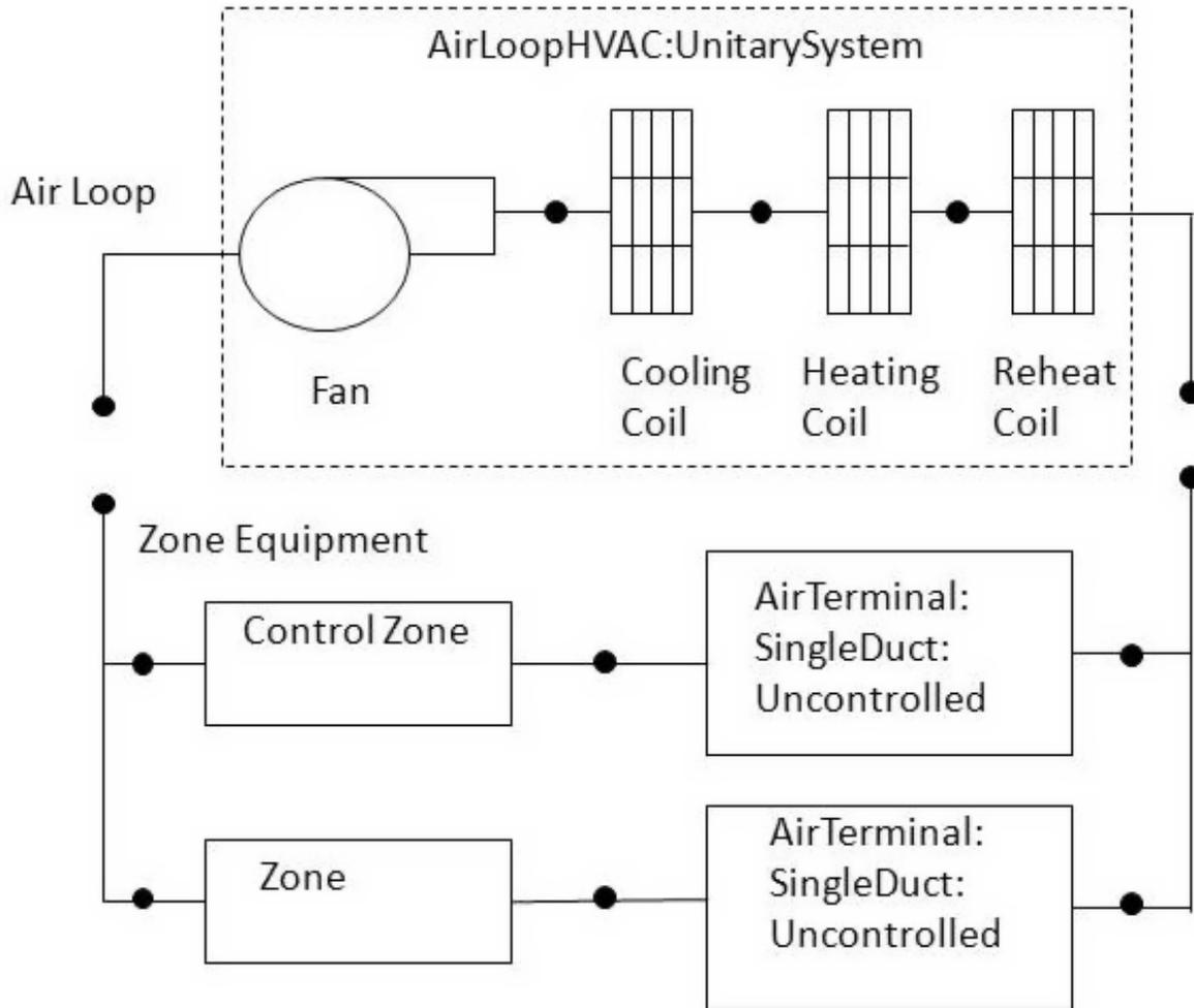
Figure 1.153: Schematic of the EnergyPlus Unitary System
