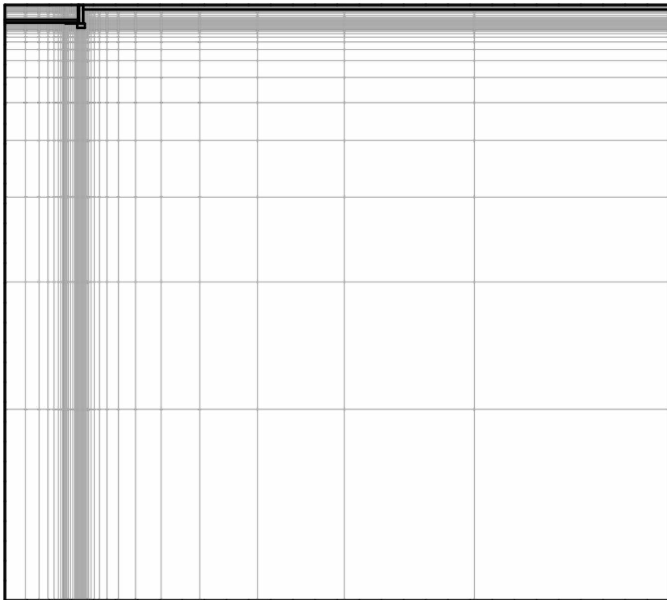
Figure 3.28: Example generated discretization of full domain
