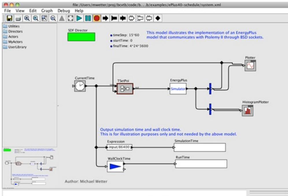
Figure 2: System model in the BCVTB.
