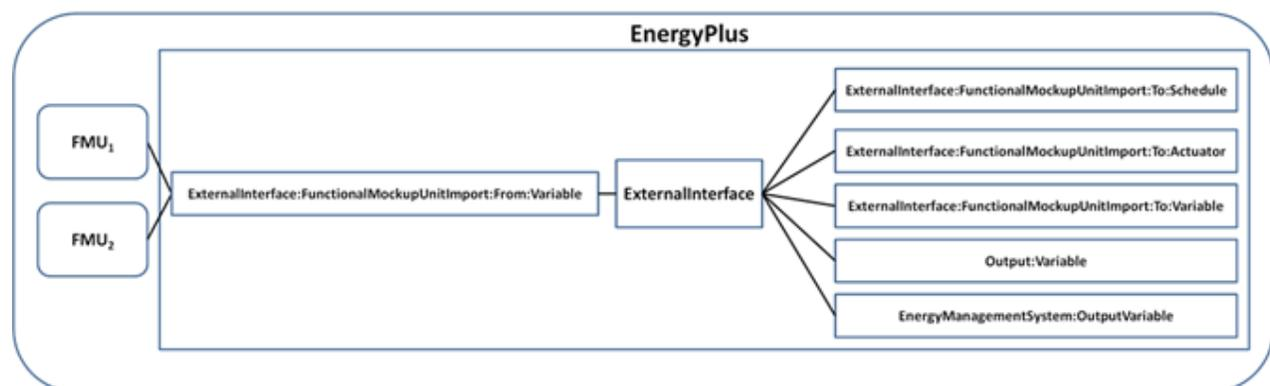
Figure 9: Architecture of the FMU for co-simulation import.
