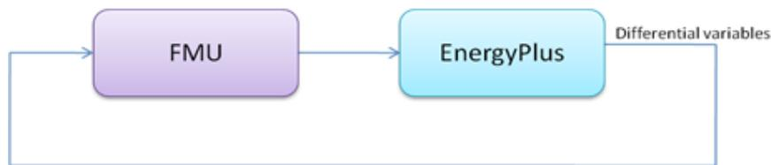
Figure 7: System with one FMU linked to EnergyPlus.
