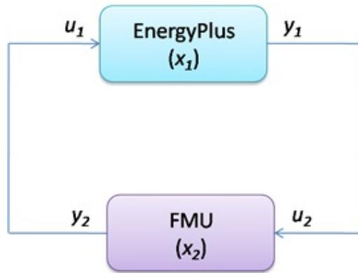
Figure 6: System with one FMU linked to EnergyPlus. HERHERHEHERHERHERHERH Table 2 shows the different system configurations that are possible.
